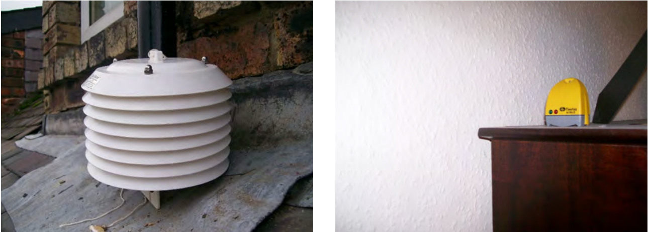
Figure 2.2 - The TinyTag temperature logger inside radiation shield (left) and dwelling (right).
