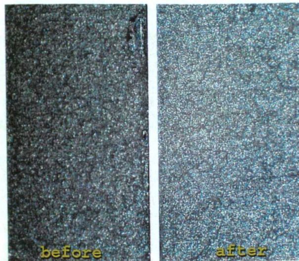
Fig. 3.7 (b) Anodised aluminium sample, without and after the test, showing no signs of corrosion
