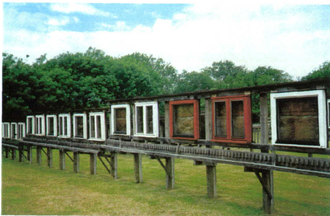
Fig. 3.2 (a) Different designs of windows being tested under natural exposure
