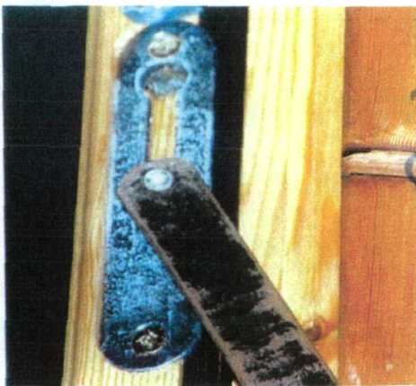
Fig. 3.14 (c) Oxidation of ironmongery of timber window under the humidity/temperature test
