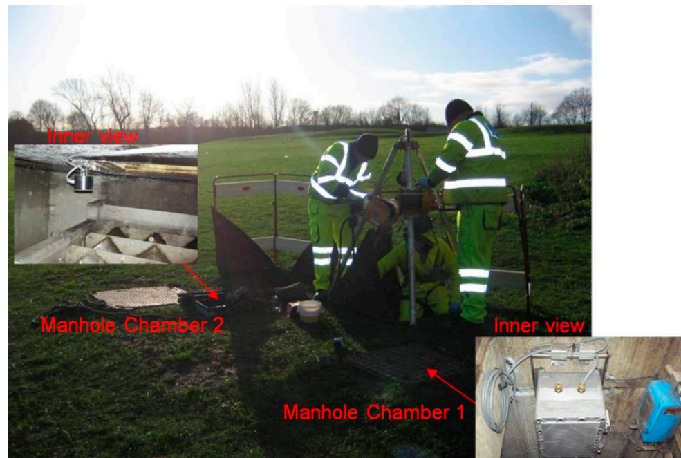
Figure 12. Practical implementation of the proposed acoustic system used in phase 2 field experiments.
