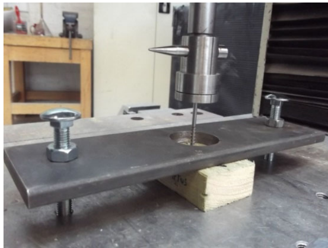
Figure 7-7: Screw pull-out test set-up
