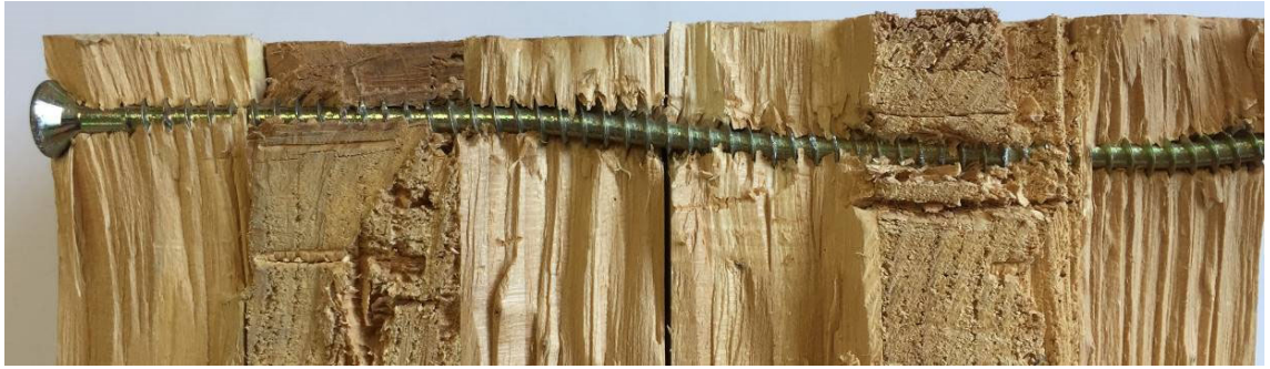
Figure D- 2 Screw dowel double shear test
