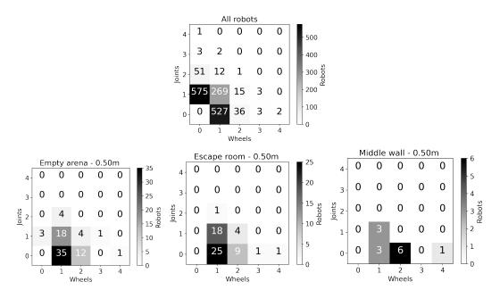
**Figure 7.** The number of robots with different combinations of organs. The top plot shows all the robots in all the bootstrap populations. The bottom figures show only the robots that got within 0.5 m of the target for the empty arena, escape room and the middle wall mazes, respectively.
