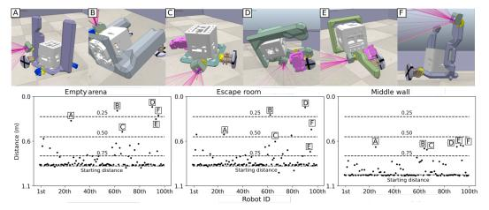
**Figure 8.** Evaluation of each robot of a single bootstrap population for the empty arena, the escape room and the middle wall. The performance of the same 6 robots (**A–F**) changes from one environment to another.
