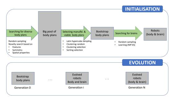
**Figure 2.** Overall system diagram. Upper image: Initialisation process. Firstly a large pool of robot body plans is generated, aiming for diversity. Then a subset of these body plans is selected focusing on manufacturability and viability. In the third step, controllers are generated for these body plans to form complete robots. Lower image: Evolutionary process. The robots from the bootstrap population are evolved.
