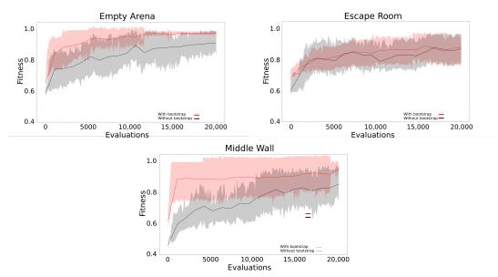
**Figure 12.** The fitness curve of the body plan + controller evolution experiments for the empty arena, escape room and middle wall. Experiments with the bootstrap population take fewer evaluations to converge to a solution than with a random initial population for the empty arena and the middle wall.
