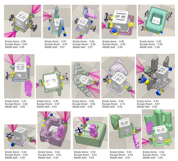
**Figure 11.** This figure shows 15 robots with their performance in each environment. The robots in the upper row had a good performance, the robots in the middle row had medium performance and the robots in the bottom row had a low performance. Under each picture is written the fitness of the robot in each environment.
