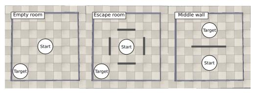
**Figure 6.** Environments used for the experiments in this paper: *empty arena, escape room* and *middle wall*. Each robot has to reach the target from the starting point. The size of the arena is  $2 \times 2$  m. In each experiment the robot starts in the same location with the same orientation.
