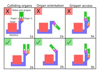
**Figure 4.** This figure shows the constraints imposed by the Robot Fabricator. The top row shows some examples of invalid body plans and the bottom row shows valid examples of body plans. If one of the organs violates at least one of these constraints, that organ is removed from the final body plan.
