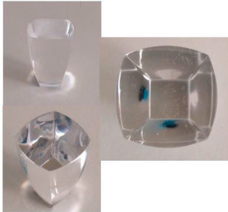
Fig. 1. RACPC manufactured using CNC machining.
