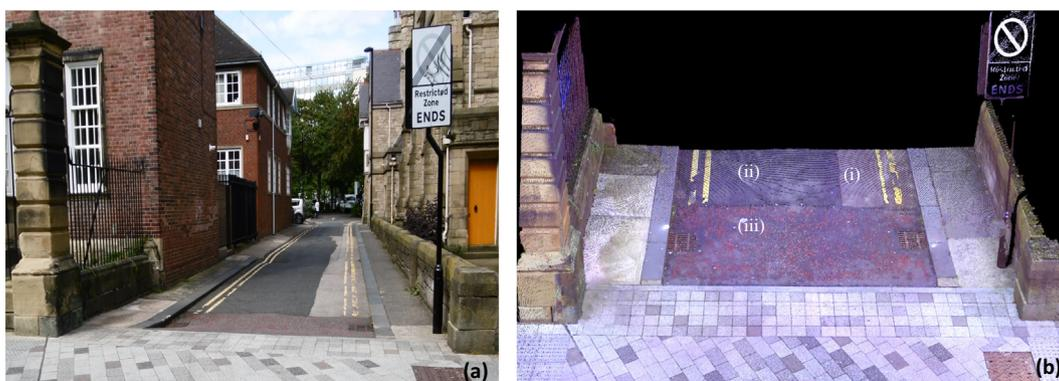
**Fig. 4.** Field site: The field site was located adjacent to St James Church on Northumberland Road, Newcastle Upon Tyne, UK Grid Reference NZ 251 12 64814. (a) Conventional photograph of the field site. (b) Point cloud panorama of the site captured using the Faro Focus 3D X Series phased-based laser scanner. The three surfacing materials studied are (i) surface dressing, (ii) dense bitumen macadam, and (iii) hot rolled asphalt.
