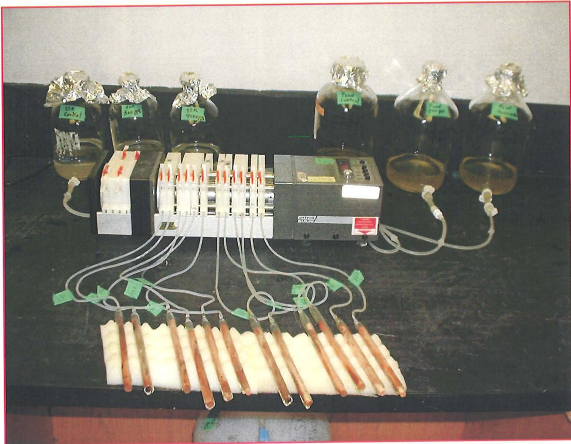
**Figure 34.** Photograph of apparatus used to determine the colonizing behaviour, over 33 days, of bacteria and fungi on the surface of previously dry *Scirpus* stems after they were introduced to natural and tetracycline-spiked river and pond water. Note the *Scirpus* stems in glass tubes in the foreground.
