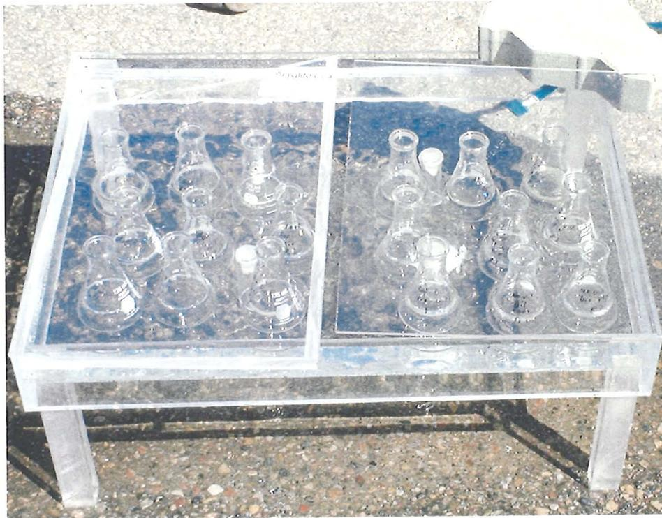
**Figure 24.** Photograph of apparatus used to conduct the tetracycline photolysis in natural sunlight experiment.
