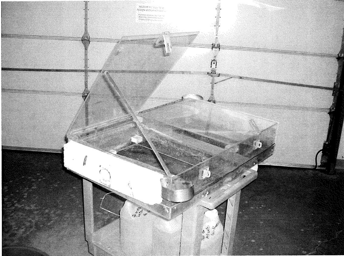
**Figure 12.** Photograph of the floating two compartment chamber used in the solar radiation experiment to study *Scirpus* decomposition in the water, as affected by solar radiation.
