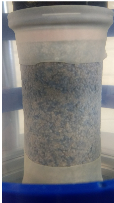
Figure 5.4: Membrane after consolidation during cyclic triaxial test
