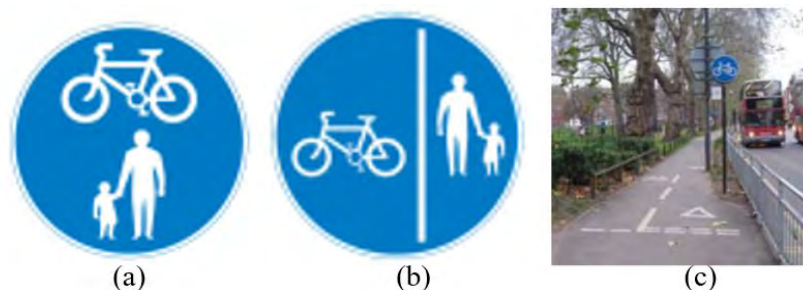
Figure 2-10 Shared cycling infrastructure signage (a) Unsegregated, (b) Segregated and (c) signage placement at the start/end of footway converted to a shared facility 3 .
