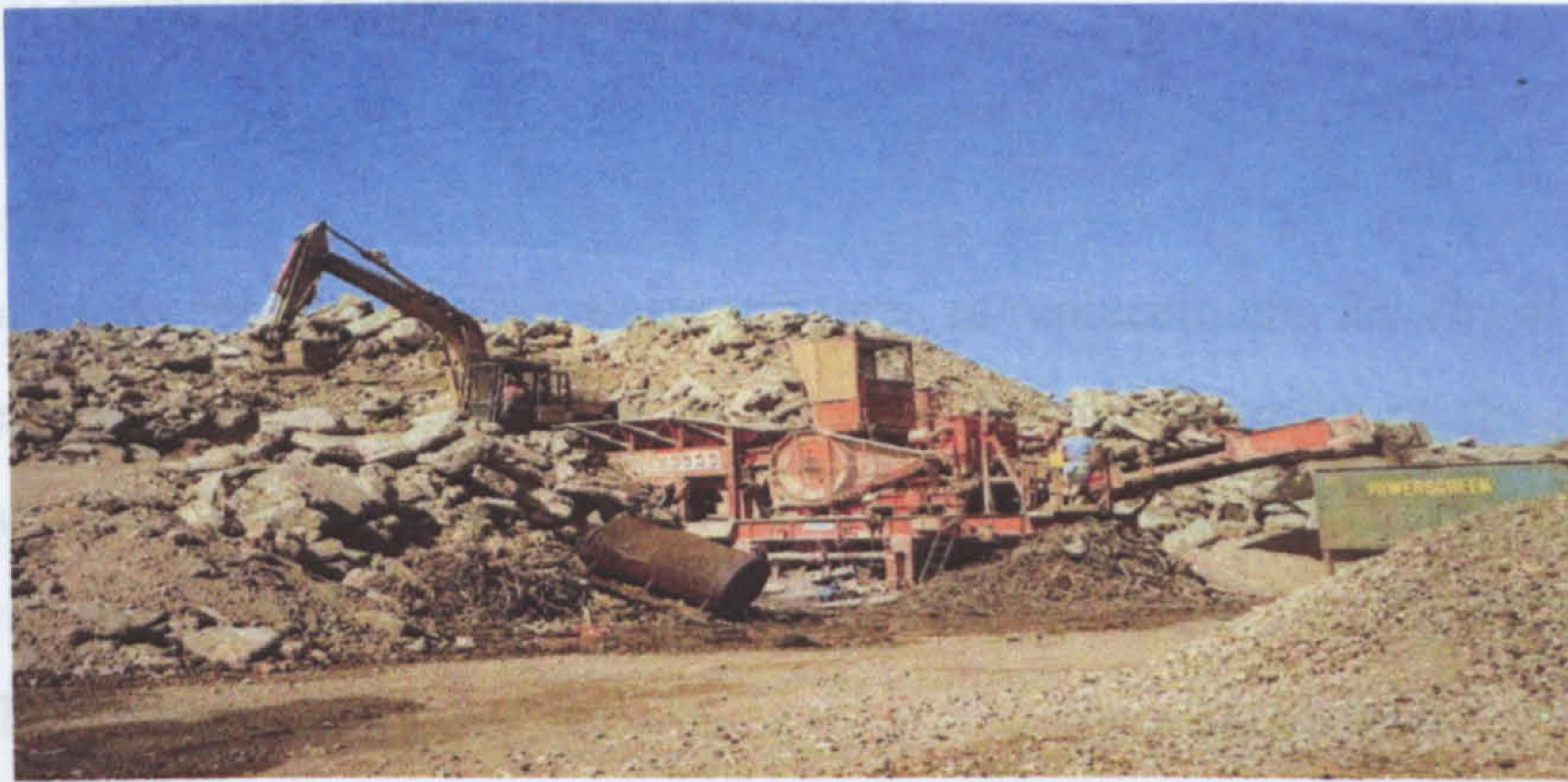
Fig. 2.13 - Crusher with manual picking belt (Humphreys 1994)
