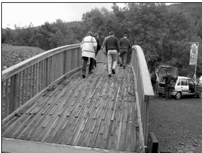
Fig. 9. Bridge at Glentress during dynamic testing: excitation by crowd walking
