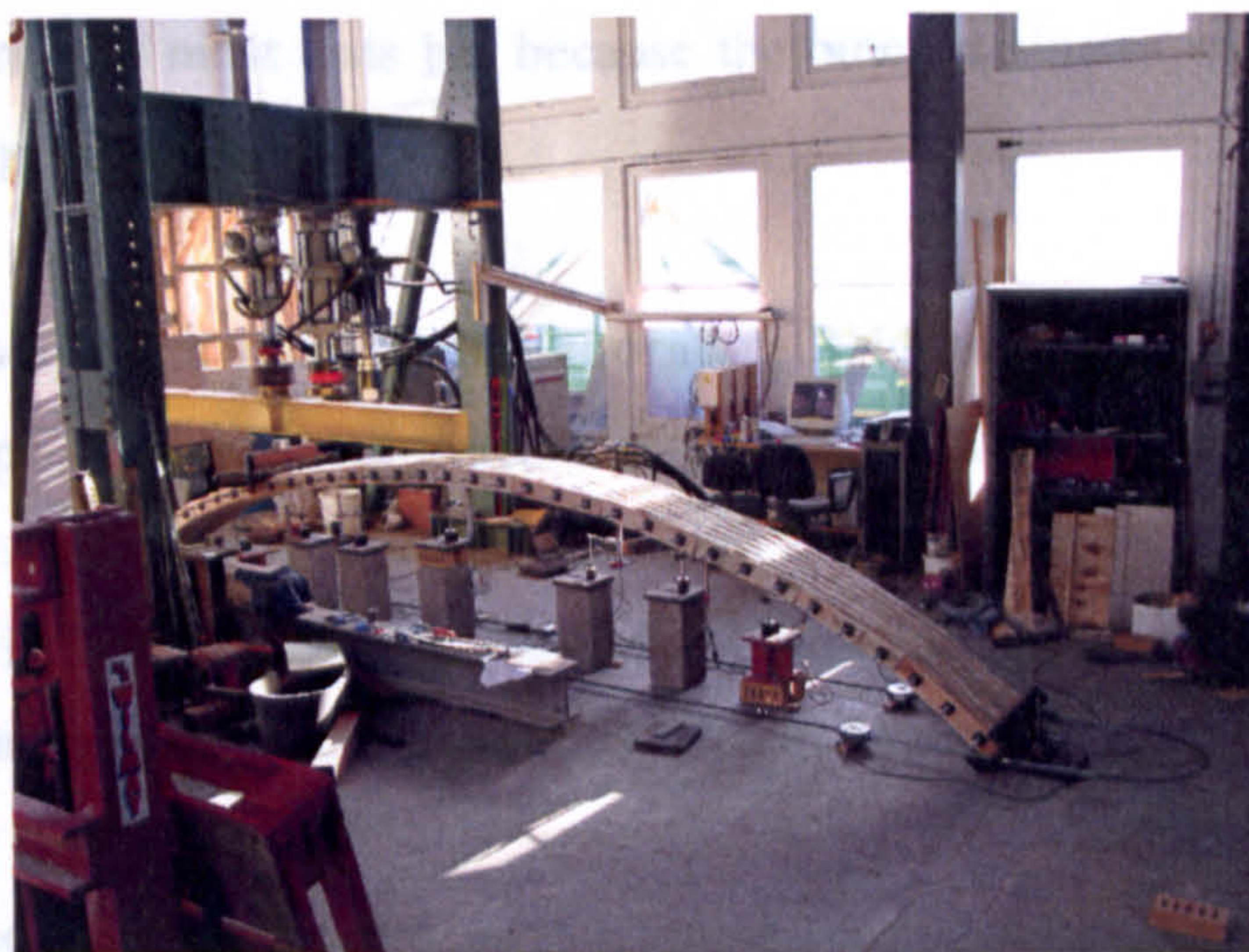
Fig 6.58 – 6m span, 1000mm rise under quarter point loading
