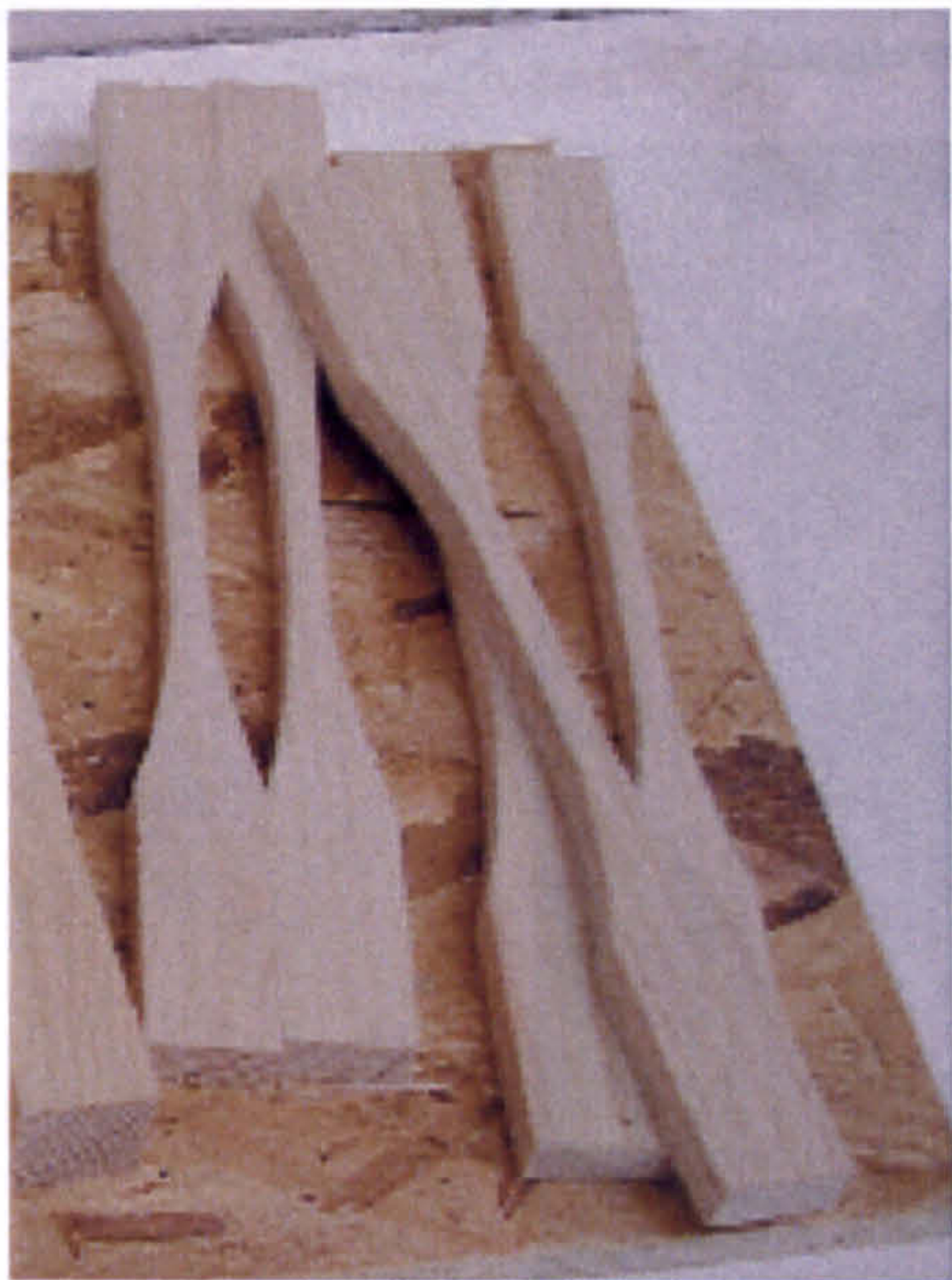
I shaped samples (left) for tension testing and sample in rig (right)
