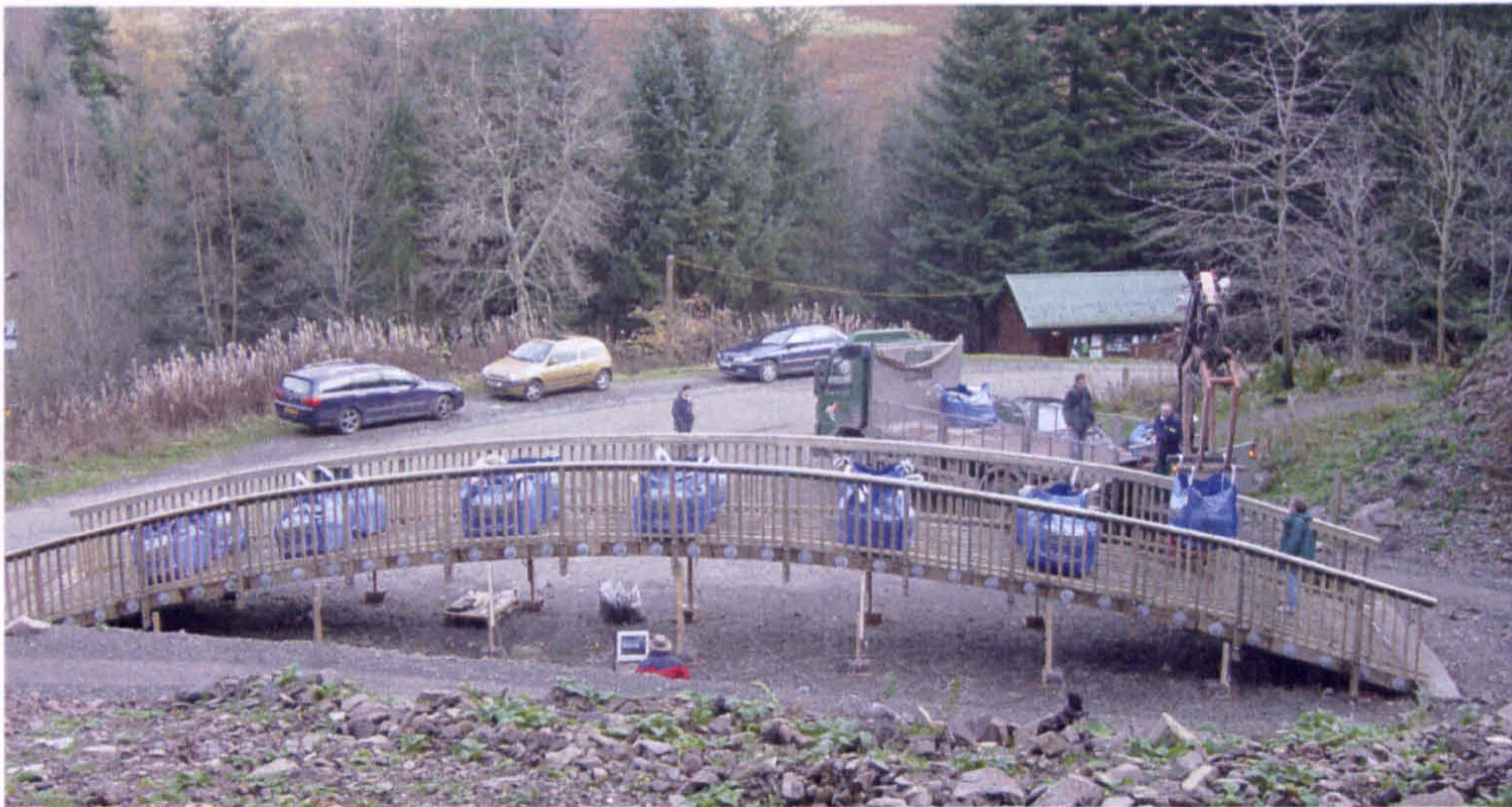
Fig 6.7 – 20m span bridge with kentledge loading
