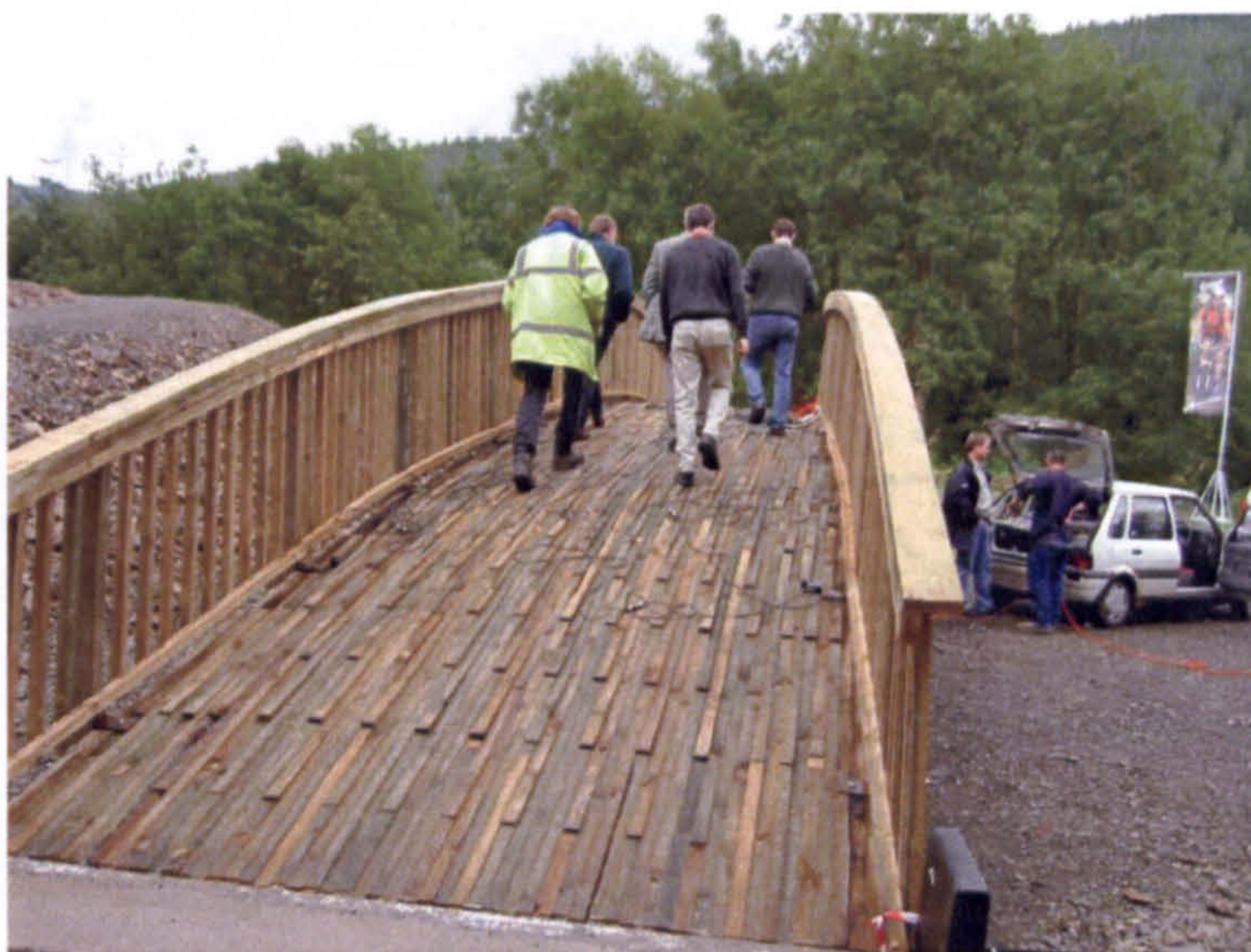
Fig 6.52 - Bridge at Glentress during dynamic testing – excitation by crowd walking. vibration tests
