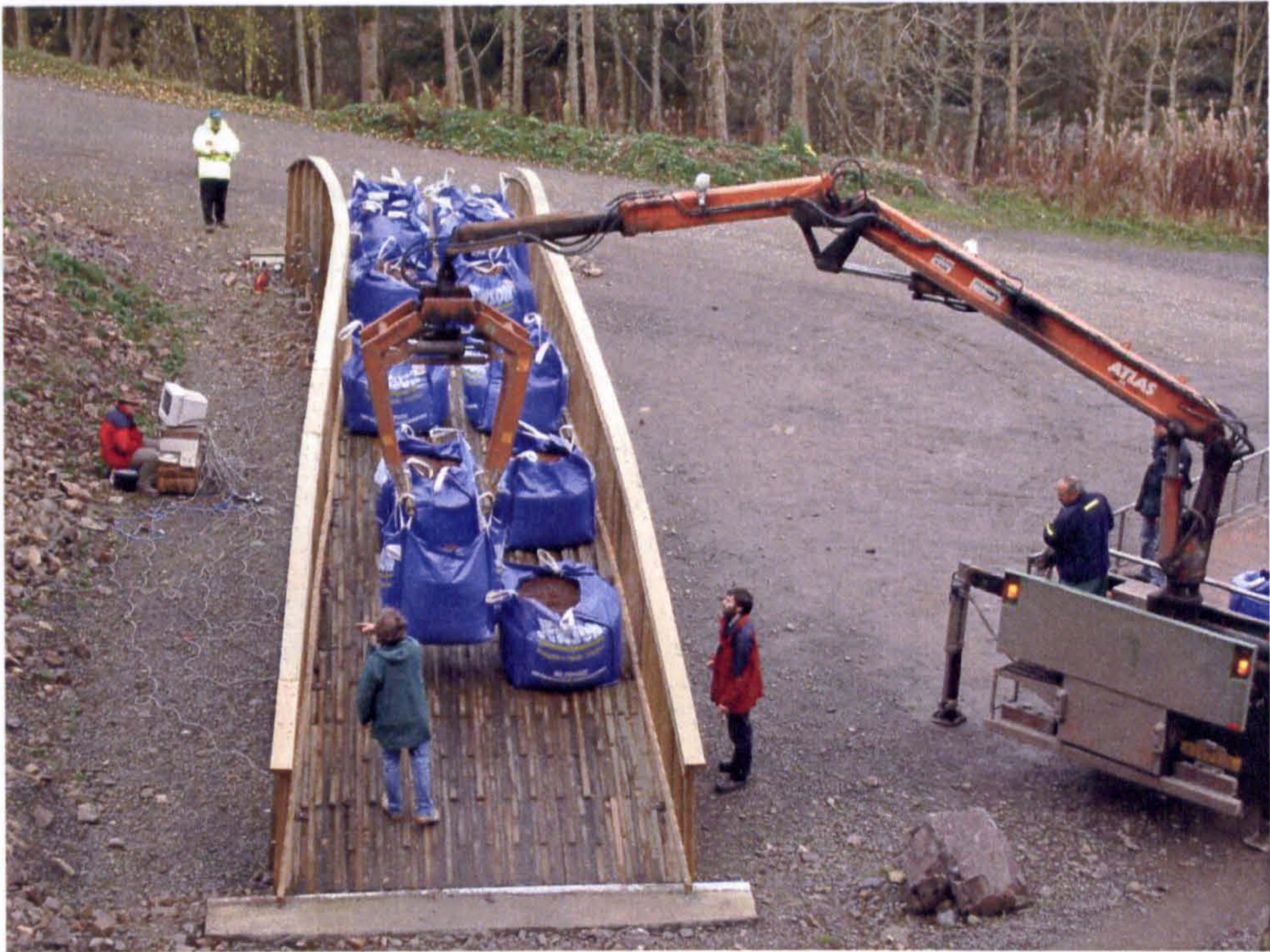
Fig 6.44(b) – 20m span UDL loading
