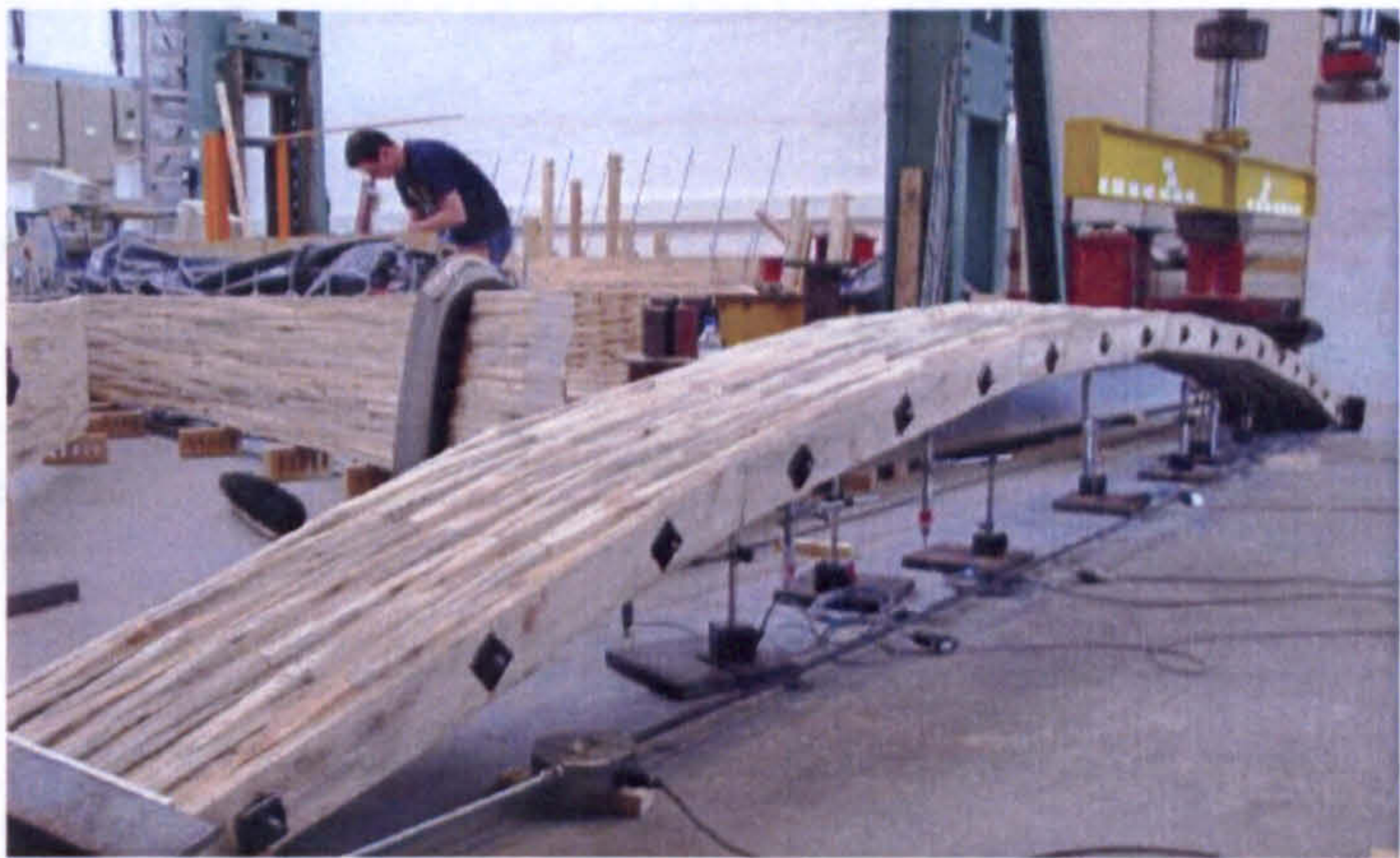
Fig 8.10(a) – 6m span arch tested for varying lateral tensions
