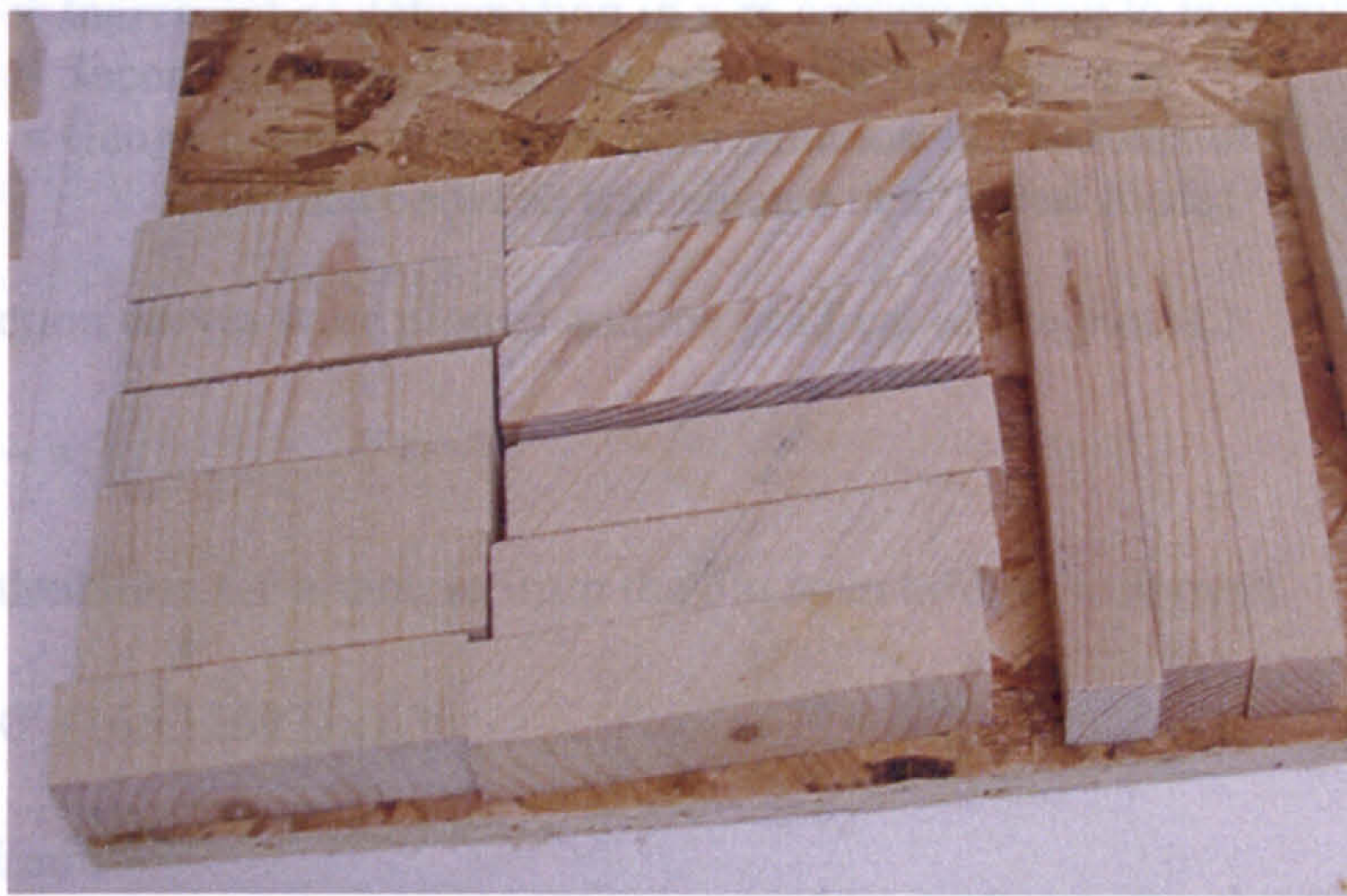
Samples cut with varying grain orientation for compression testing
