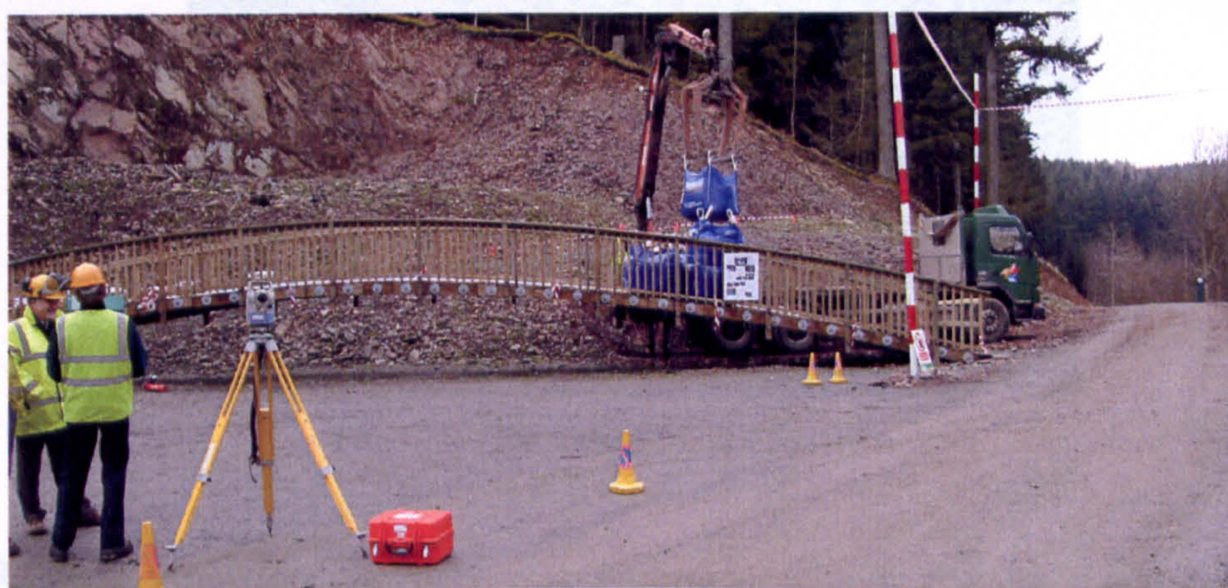
Fig 6.10 – Sokkia Total Station – Remote deflection measurements
