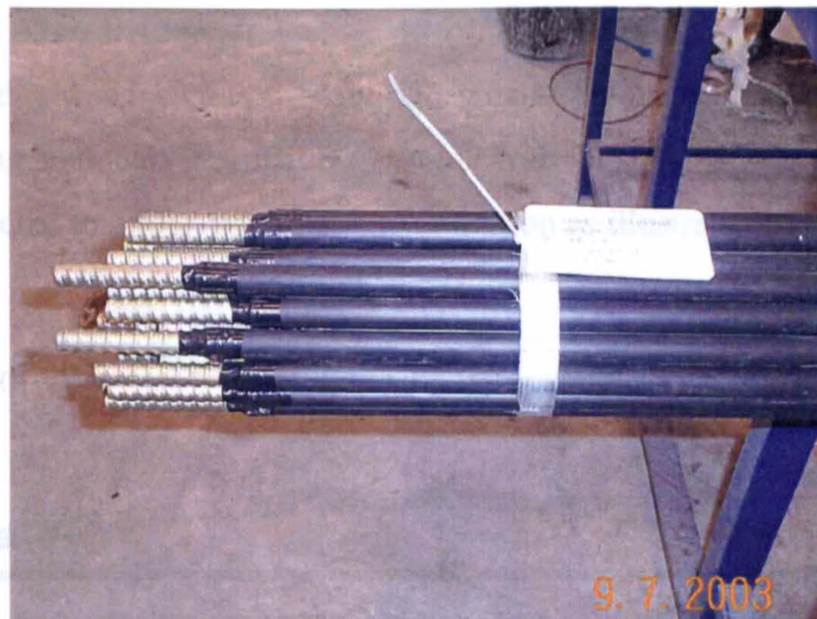
Fig 6.20 – Stressing bars, greased and sleeved
