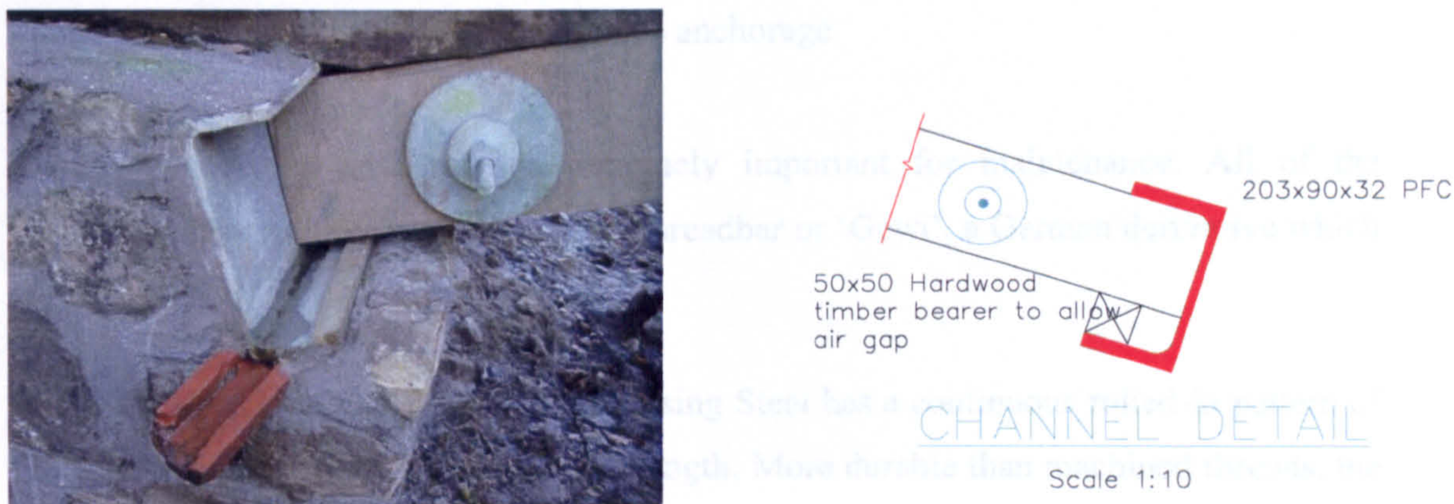
Fig 5.6 - End bearing detail - Carribber bridge
