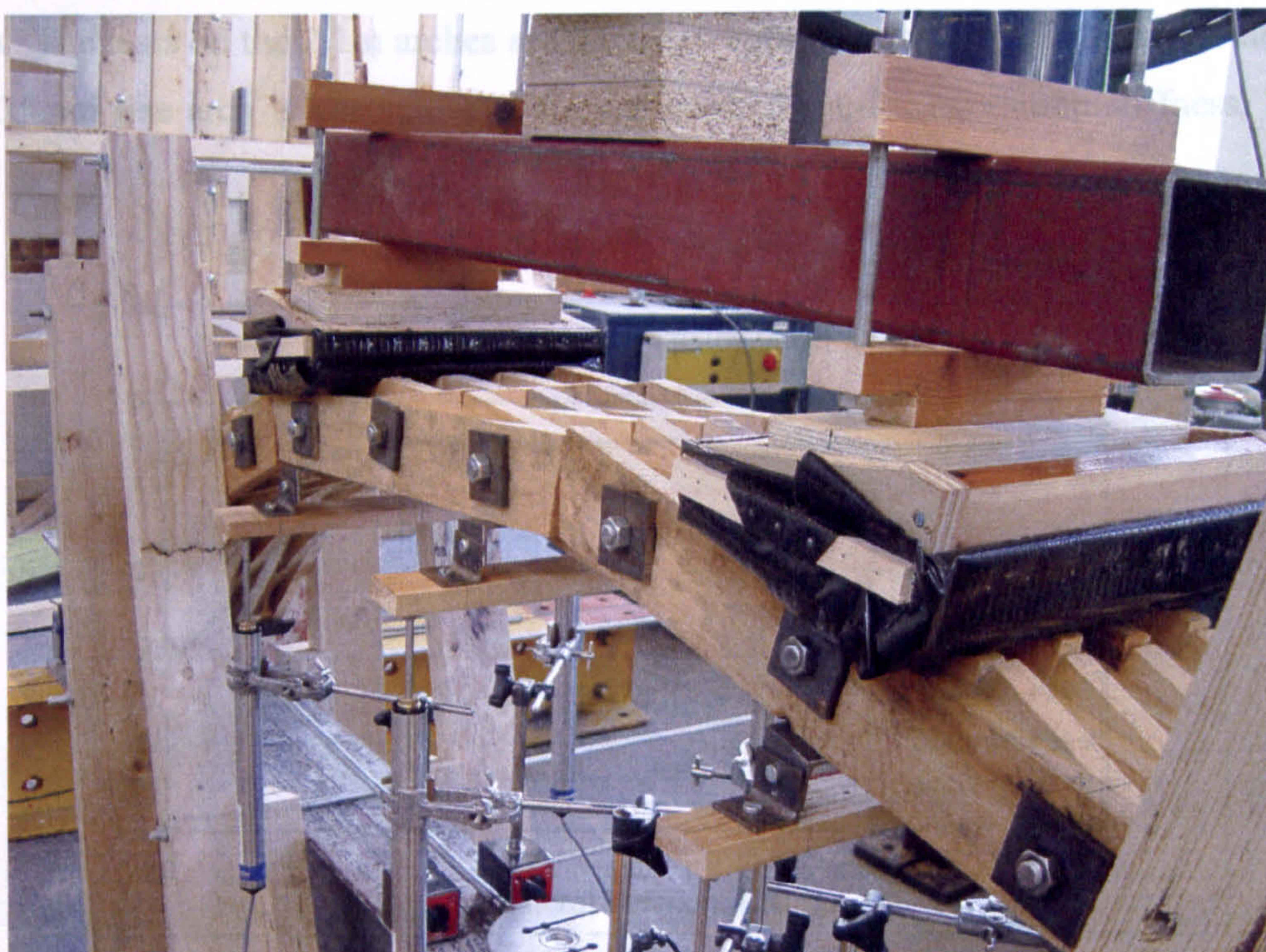
7.14b – Threaded bar and nut fixing – 2.1m span, 447mm rise
