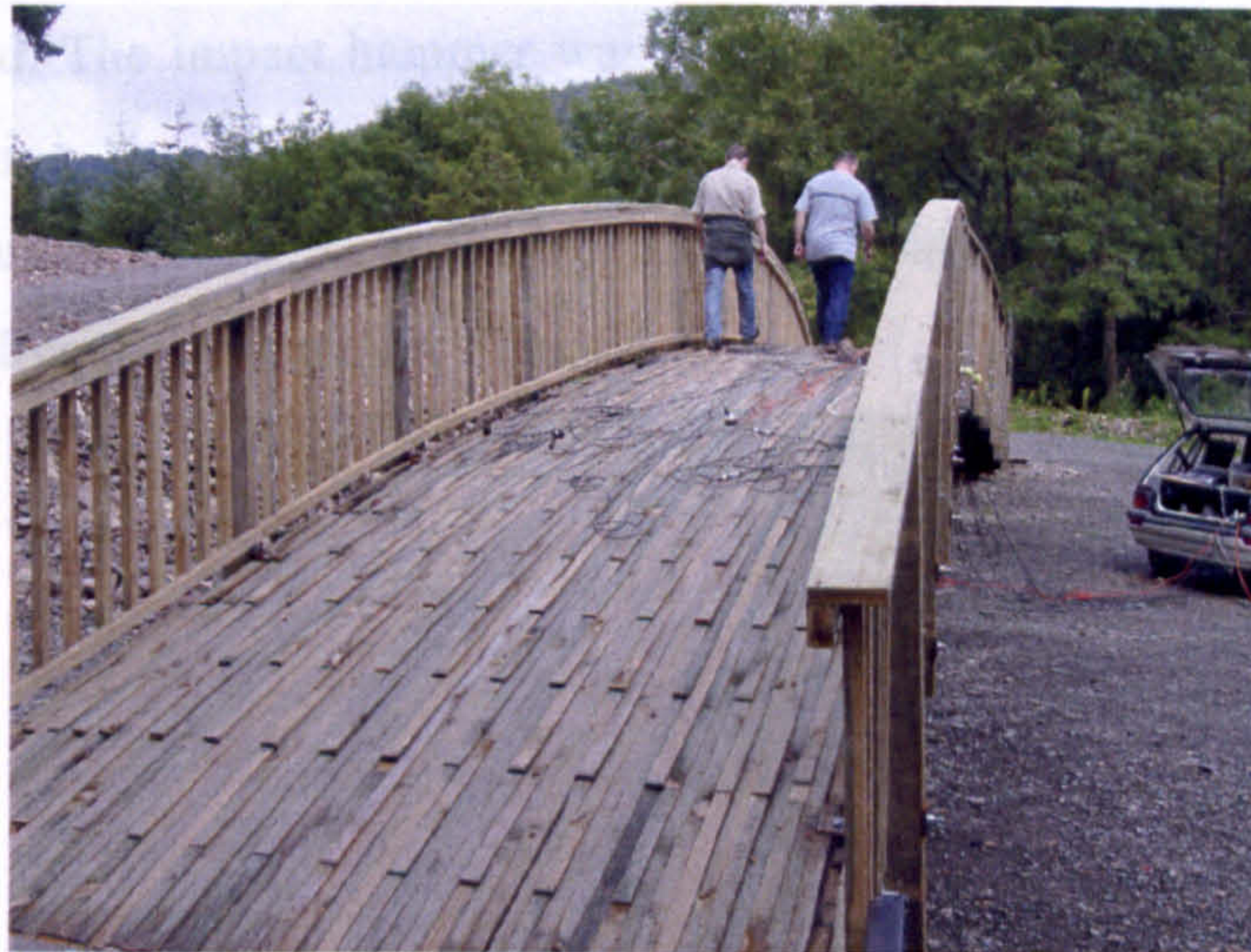
Fig 6.11 – Excitation for ARTeMIS test
