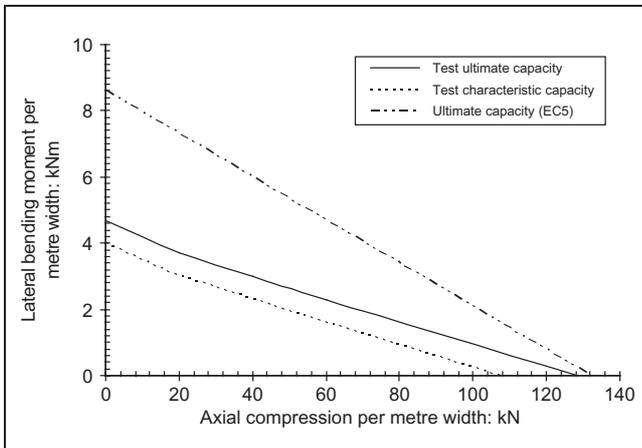
Fig. 8. Comparison of combined bending and axial compression capacity of SIP wall panels of 2.4 m high with 117 mm overall thickness and 11 mm thick OSB facings
