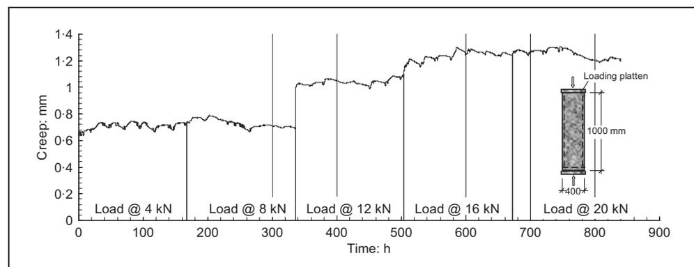
Fig. 12. Creep characteristics of the panel subject to axial compression load of 4, 8, 12, 16 and 20 kN over 840 h
