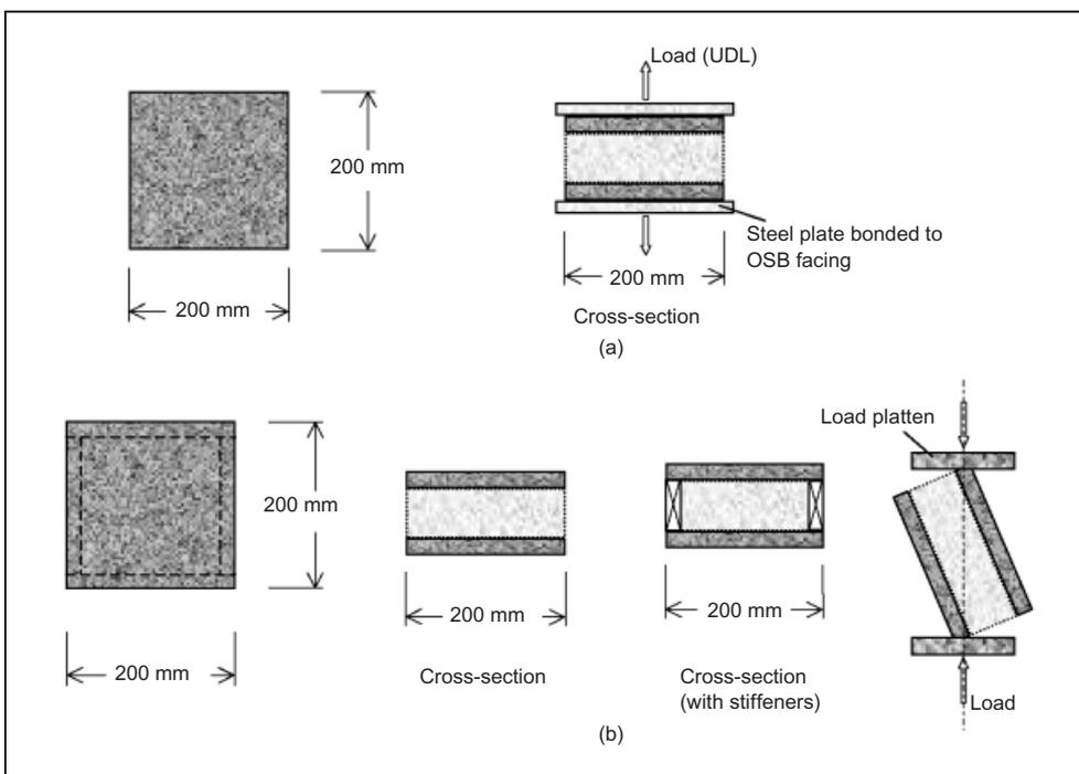
Fig. 9. Tension and shear tests: specimens and details. (a) Tension perpendicular to the plane of the panel; (b) shear/skewed loading
