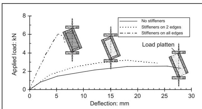
Fig. 11. Load-deformation behaviours of panels under in-plane shear/skewed loading
