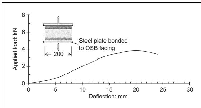
Fig. 10. Tension perpendicular to the plane of the panel
