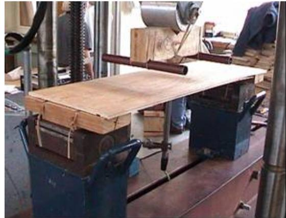
b) Testing modulus of elasticity
