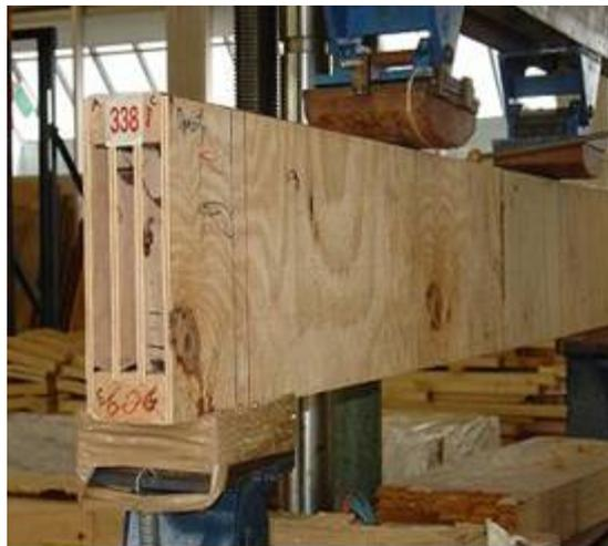
c) Boxed Double I-beam under four-point-bending
