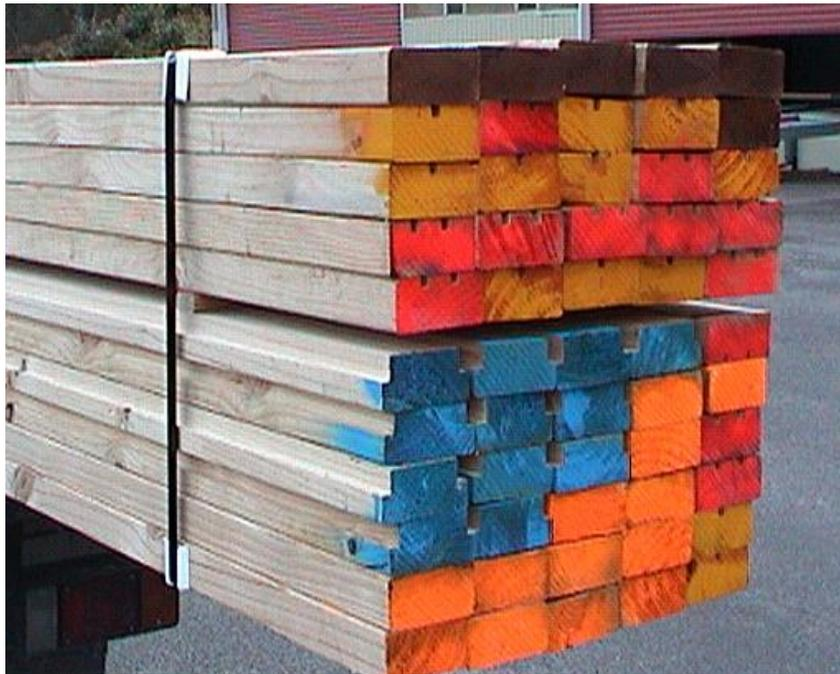
**Figure 3.6 Colour-coded flanges after machining, ready for assembly**
