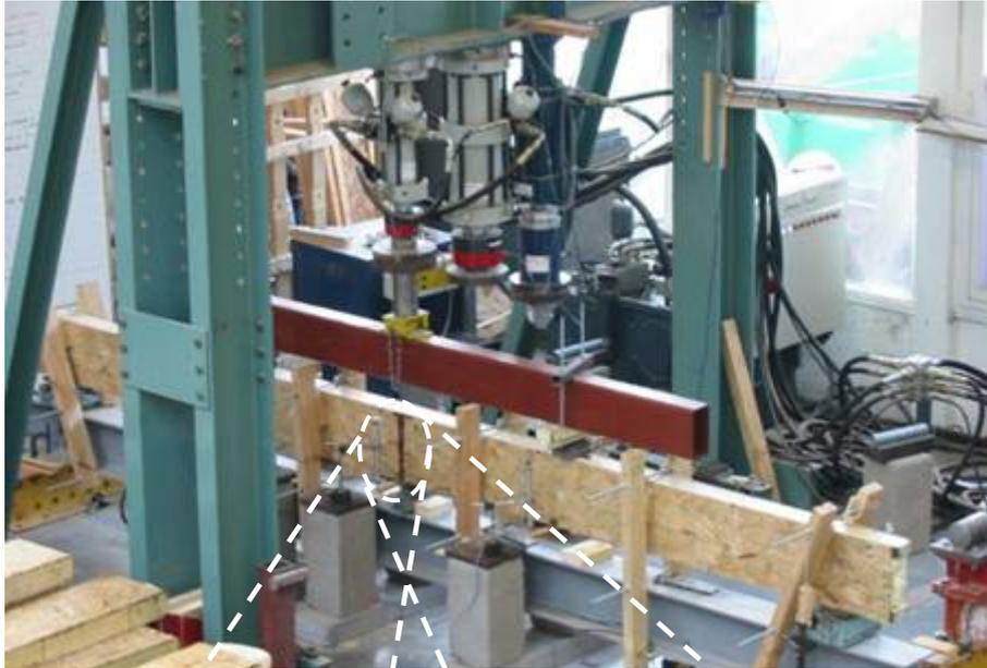
a) Destructive test, four point bending
