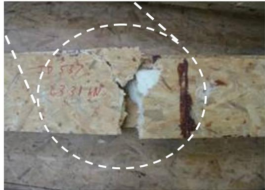
b) Flexural failure in Box I-beam
