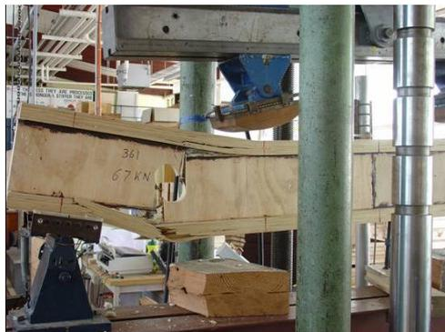
e) Filled LVL Double I-beam with web opening of 76 mm
