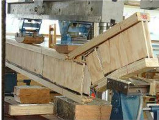
(a) A short span double I-beam
