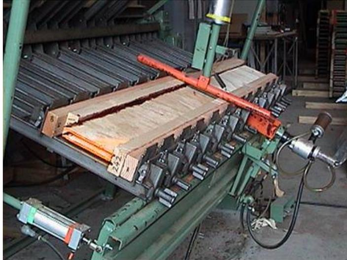
**Figure 3.10 Pneumatic press clamp (Taylor clamp)**
