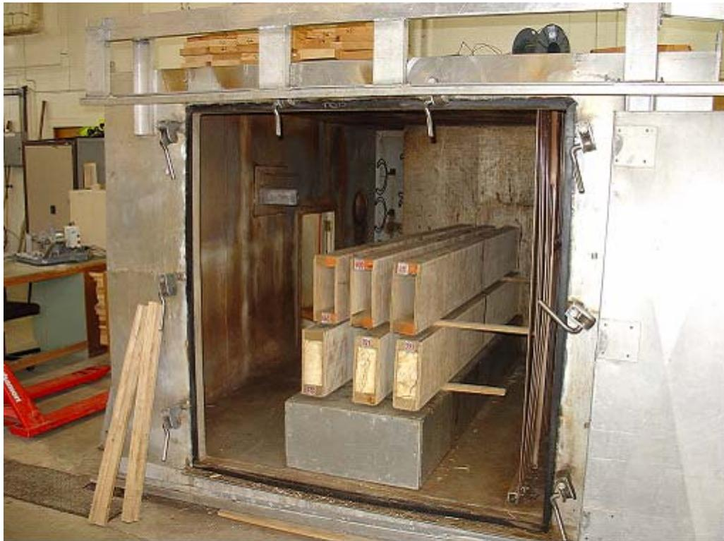
Figure 4.15 Durability tests- Box beams inside the kiln
