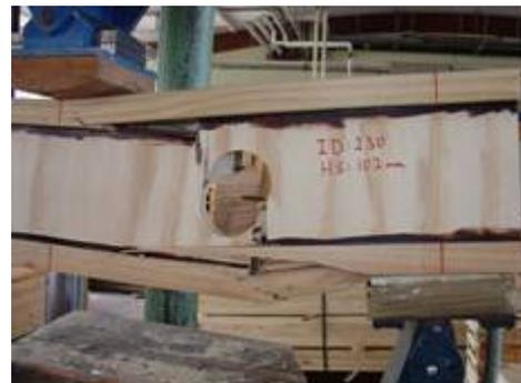
d) Double I-beam with web opening of 102 mm after failure
