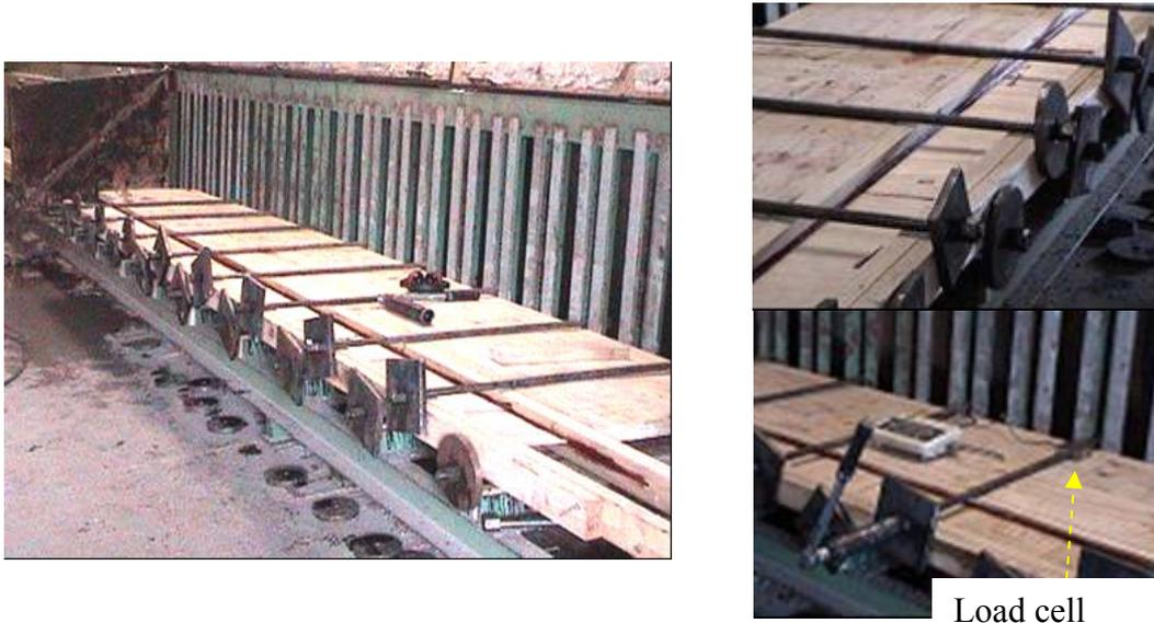
**Figure 3.11 Clamping system used for long I-beams and Double I-beams**
