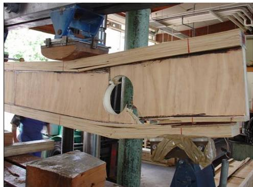
f) Filled LVL Double I-beam with web opening of 102 mm
