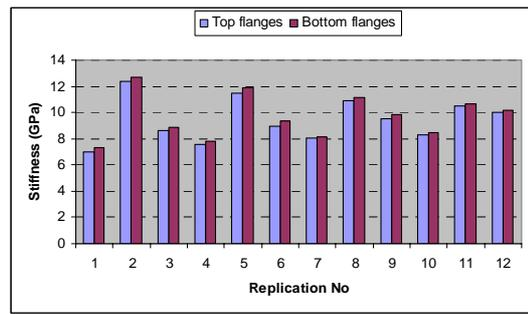
Filled Box beam-Distribution of MoE within top and bottom flanges
