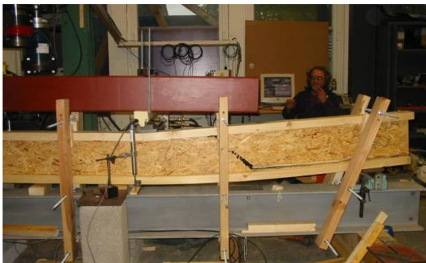
**Figure 9.15 Failure in an I-beam**
