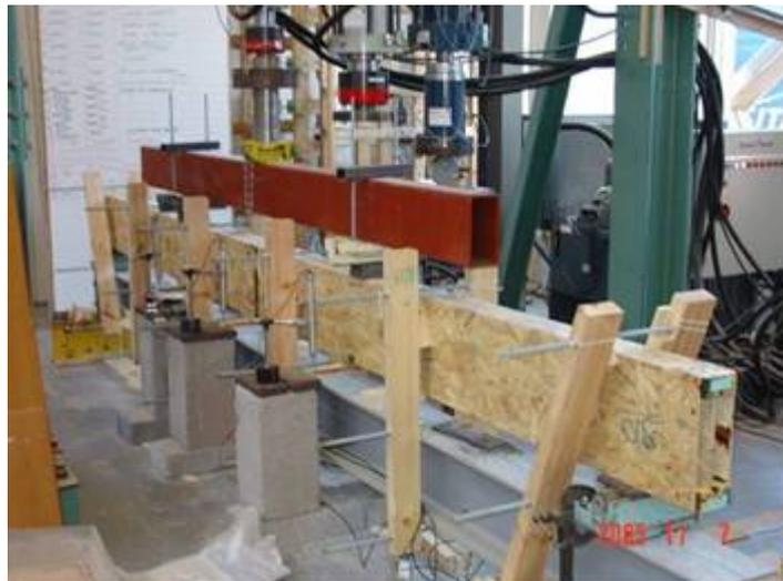
**Figure 4.17** Test rig for long span beams undergoing four-point-bending
