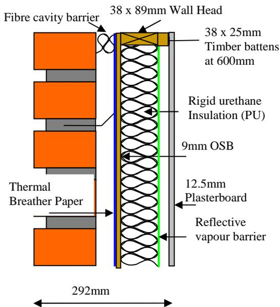
Detail 3: Polyurethane insulation installed within the frame
