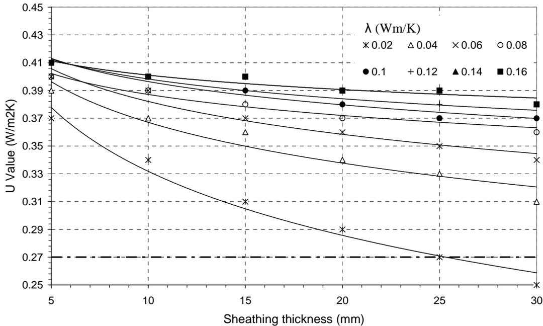
Figure 3: Relationship of wall detail U-value with changing sheathing thickness and λ value
