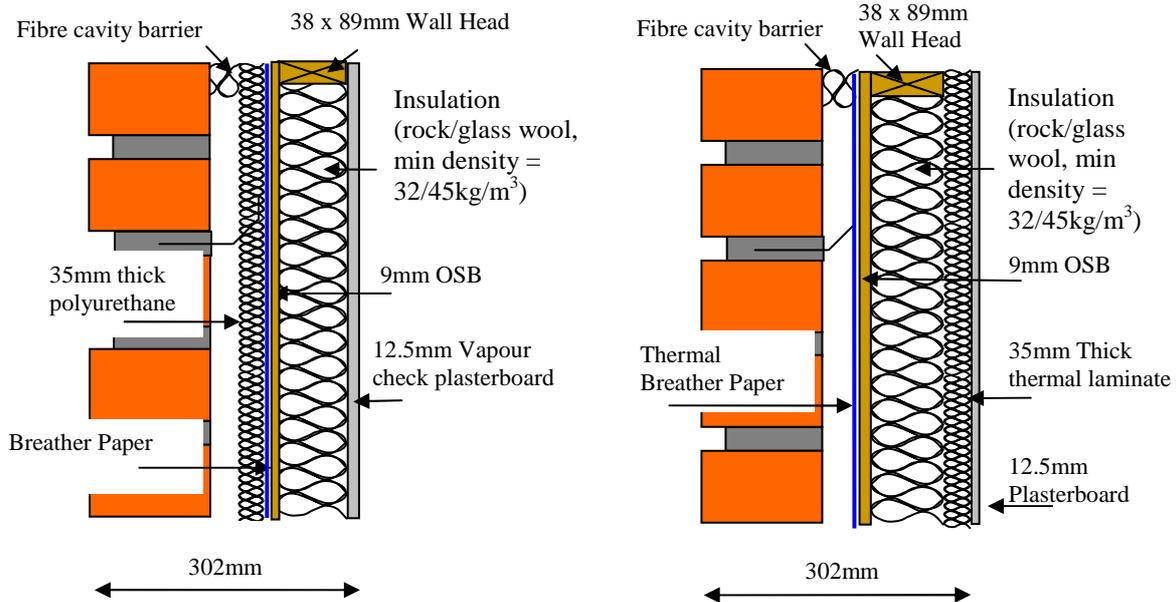
Detail 1: Cavity installed polyurethane insulation board
