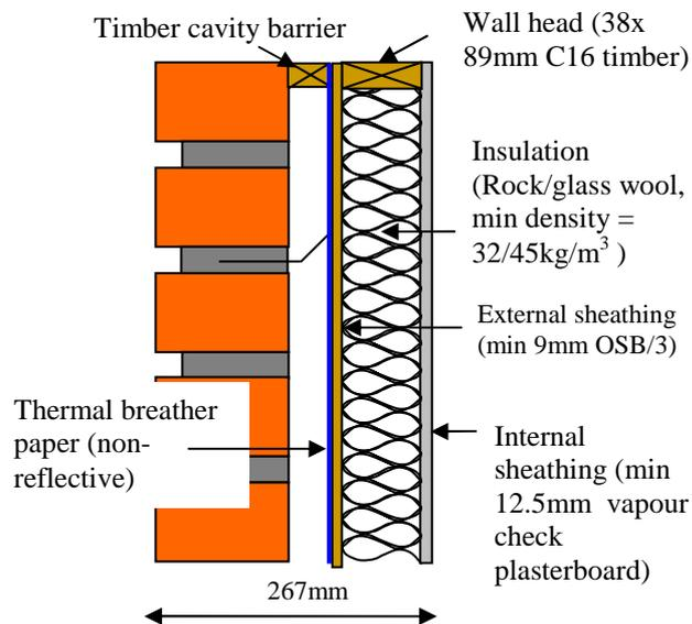
Figure 2: Standard timber frame wall detail
