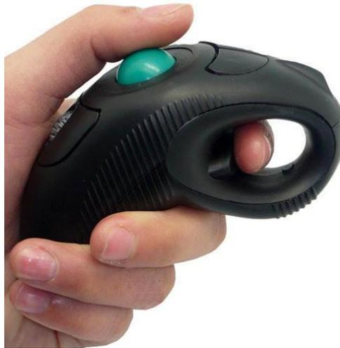
Figure 2-20: Hand-held finger ball input device (Infmetry, 2018)
