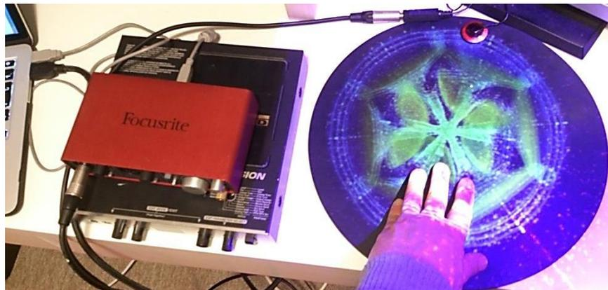
Figure 5-20: Prototype interactive rubber surface detecting vibration through a contact microphone. The signal is routed through CymaSense and projected back onto the surface.
