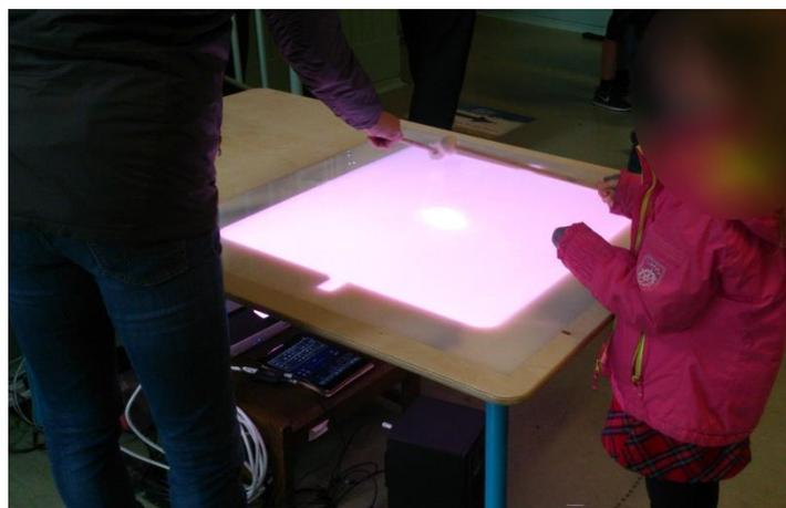
Figure 5-25: The interactive table played using beaters and showing *CymaSense* version two back-projected on the Perspex surface
