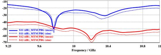
(a) Simulated and measured S-parameter response of the MTM-PBG structure.
