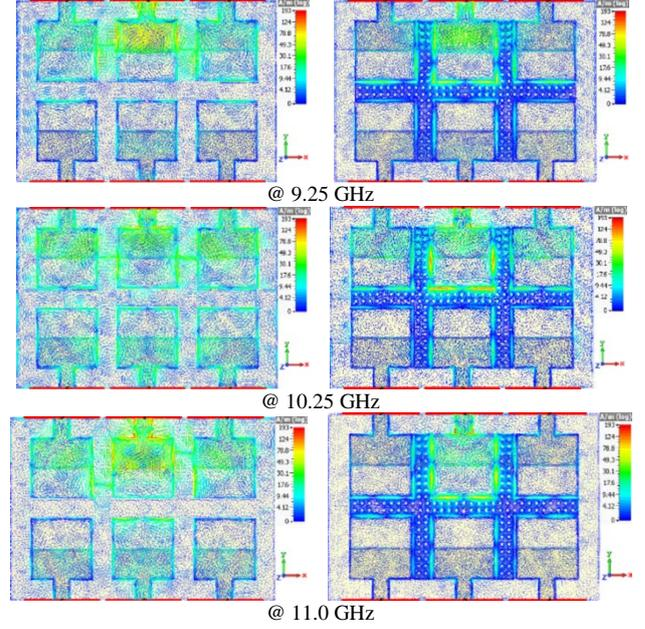
Fig.5. Surface current density distributions over the array antennas without (left side) and with (right side) MTM PBG at working frequencies. It is worth to comment that here to save space, we have only shown the surface current distributions stimulated by port #1.
