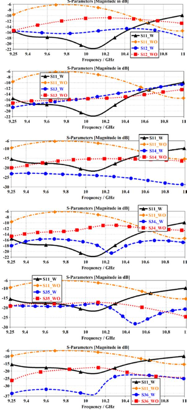
(b) Measured S-parameter of the array antenna
