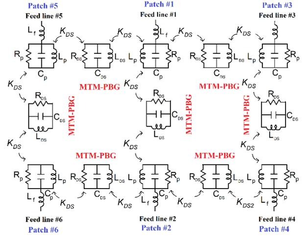
Fig.3. Simplified equivalent electrical circuit model of the proposed 3x2 array antennas loaded with MTM-PBG decoupling slab.
