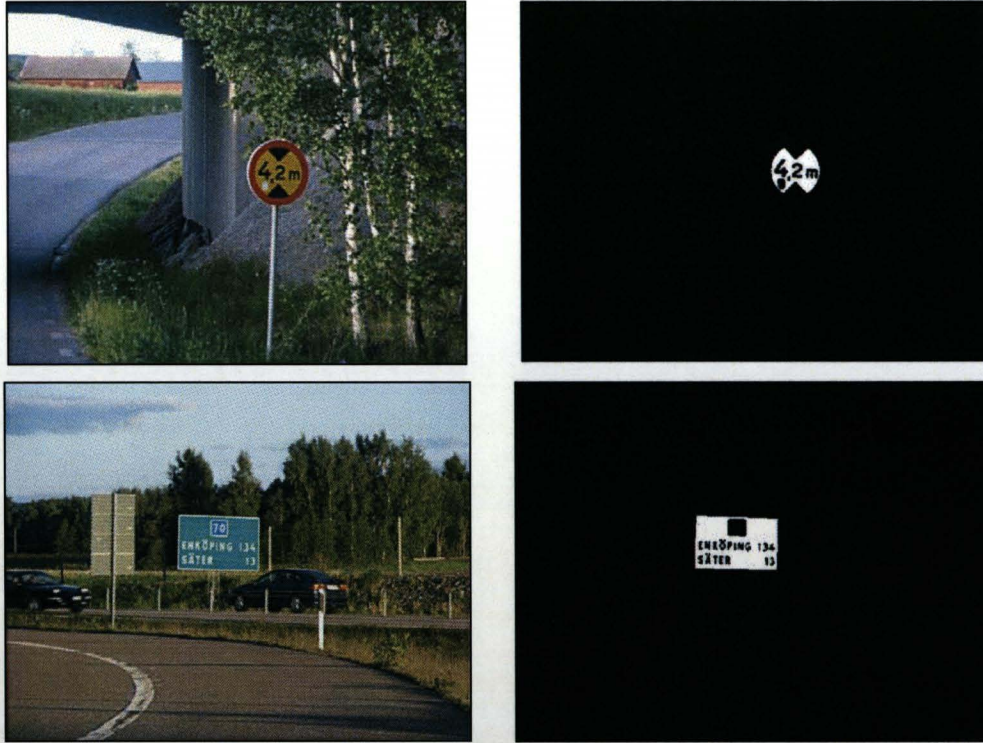
Figure 5.4: Results of colour segmentation using dynamic threshold algorithm applied for Red, Yellow and Green signs.
