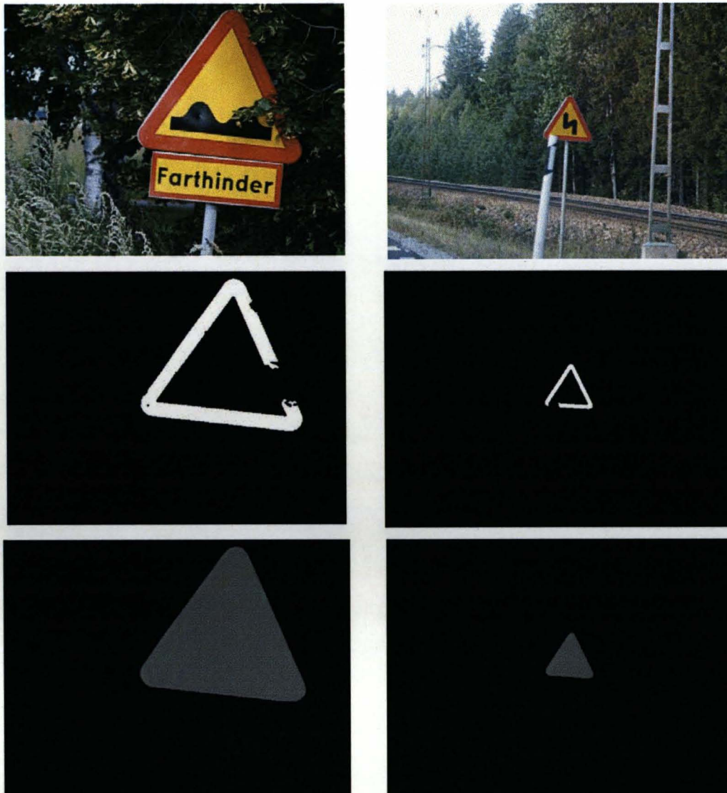
Figure 5.22: Occlusions and Convex hull. First row: Occluded objects. Second row: Results of Segmentation and Extraction. Third row: Convex hull.
