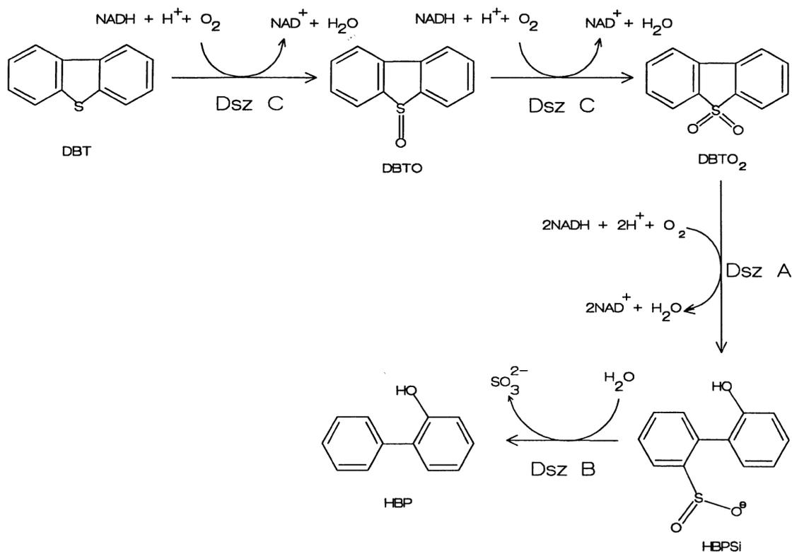
**Figure 1.1. Desulphurisation of DBT into HBP by *R. erythropolis* IGTS8.** Reproduced from Oldfield *et al.* (1997). DBT, dibenzothiophene; DBTO, dibenzothiophene 5-oxide; DBTO<sub>2</sub>, dibenzothiophene 5,5-dioxide; HBPSi, 2-(2'-hydroxyphenyl)benzene sulphinic acid; HBP, 2-hydroxybiphenyl.
