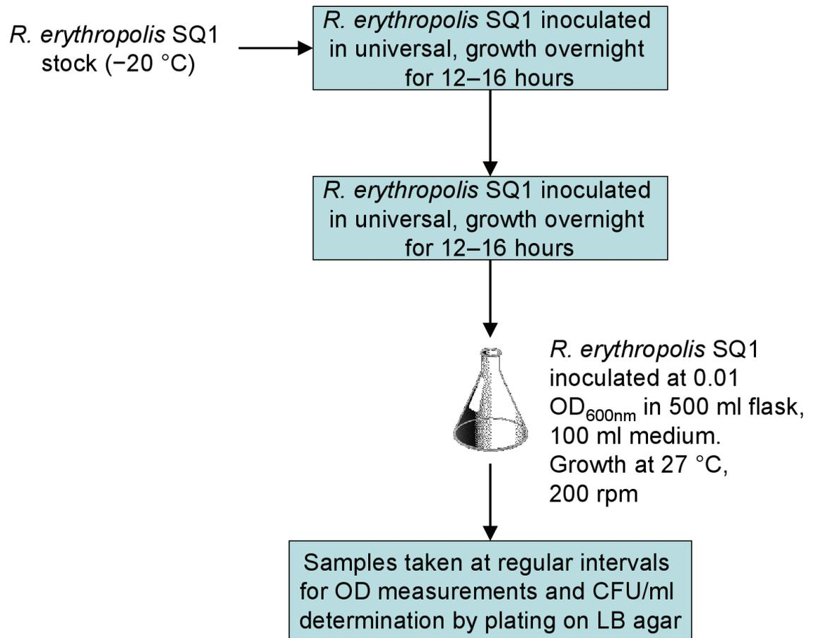
**Figure 2.1. Schematic overview of the growth experiments methodology.**
