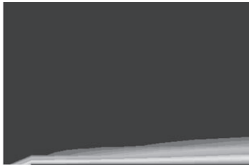
Fig. 6 Velocity boundary layer over a flat plate.
