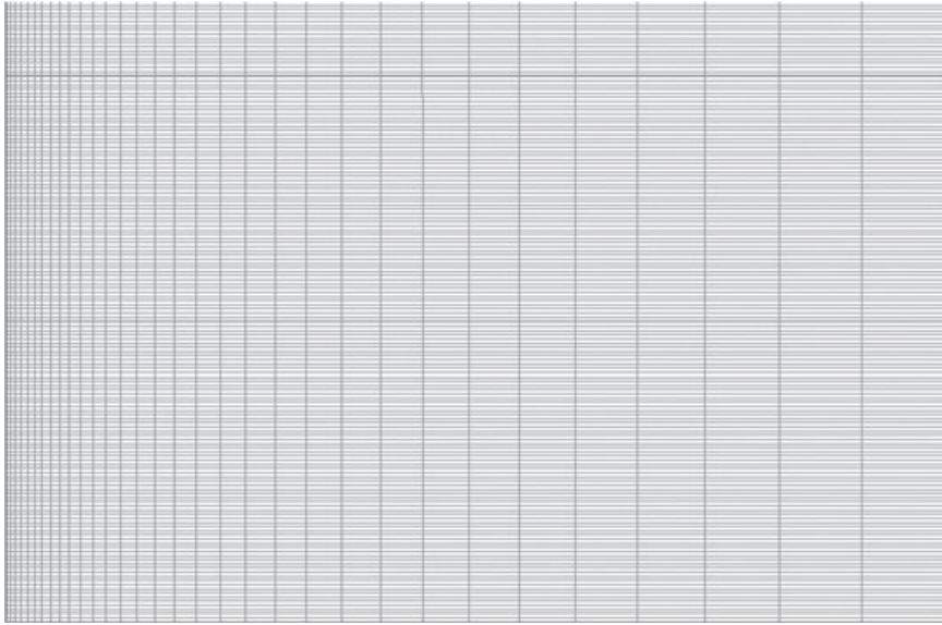
Fig. 14 Cell size can be seen to increase from left to right in the vertical plate test case.
