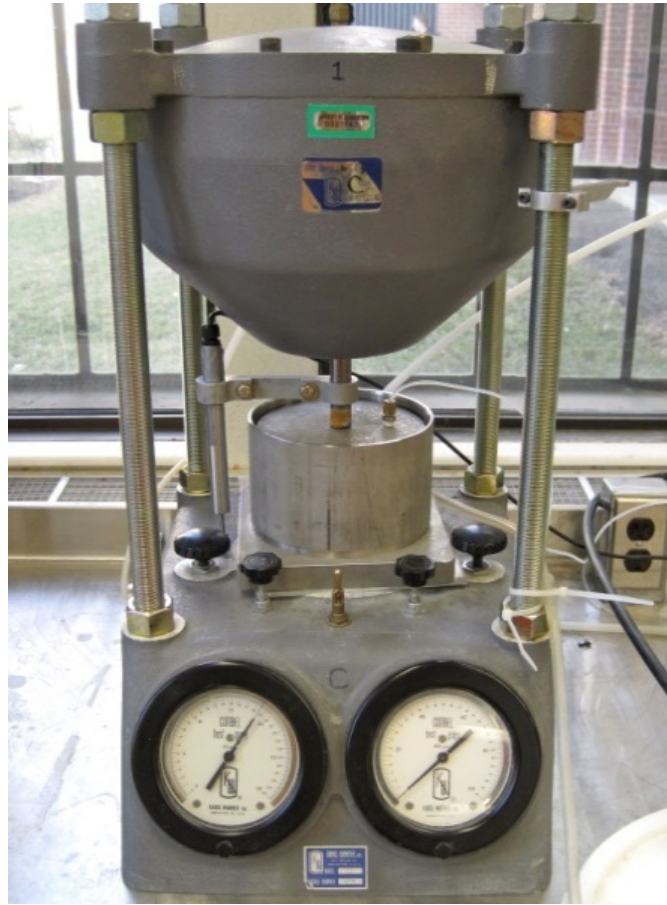
Fig. 5. Sample cell seated in pneumatic consolidation cell at University of Saskatchewan
