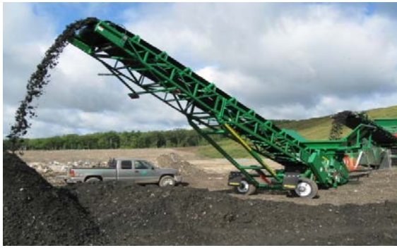
Fig. 1. Photographs showing the landfill soil reclamation process: material post screening (left) and screening plant (right).
