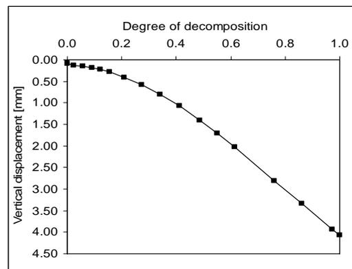
Figure 4. Vertical displacement with degree of decomposition.
