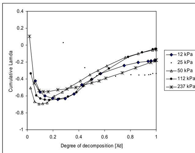
Figure 6. Cumulative  $\Lambda$  for all tests, at loadings 12, 25, 50, 112, 237 kPa.
