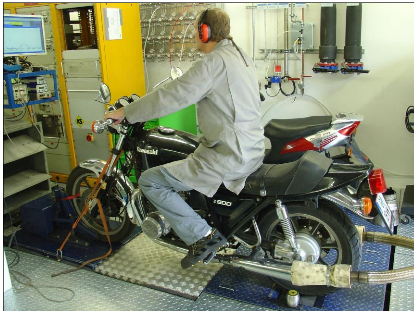
Figure 8.4 Laboratory testing on chassis dynamometer test setup with online data monitoring and conditioned system with CVS
