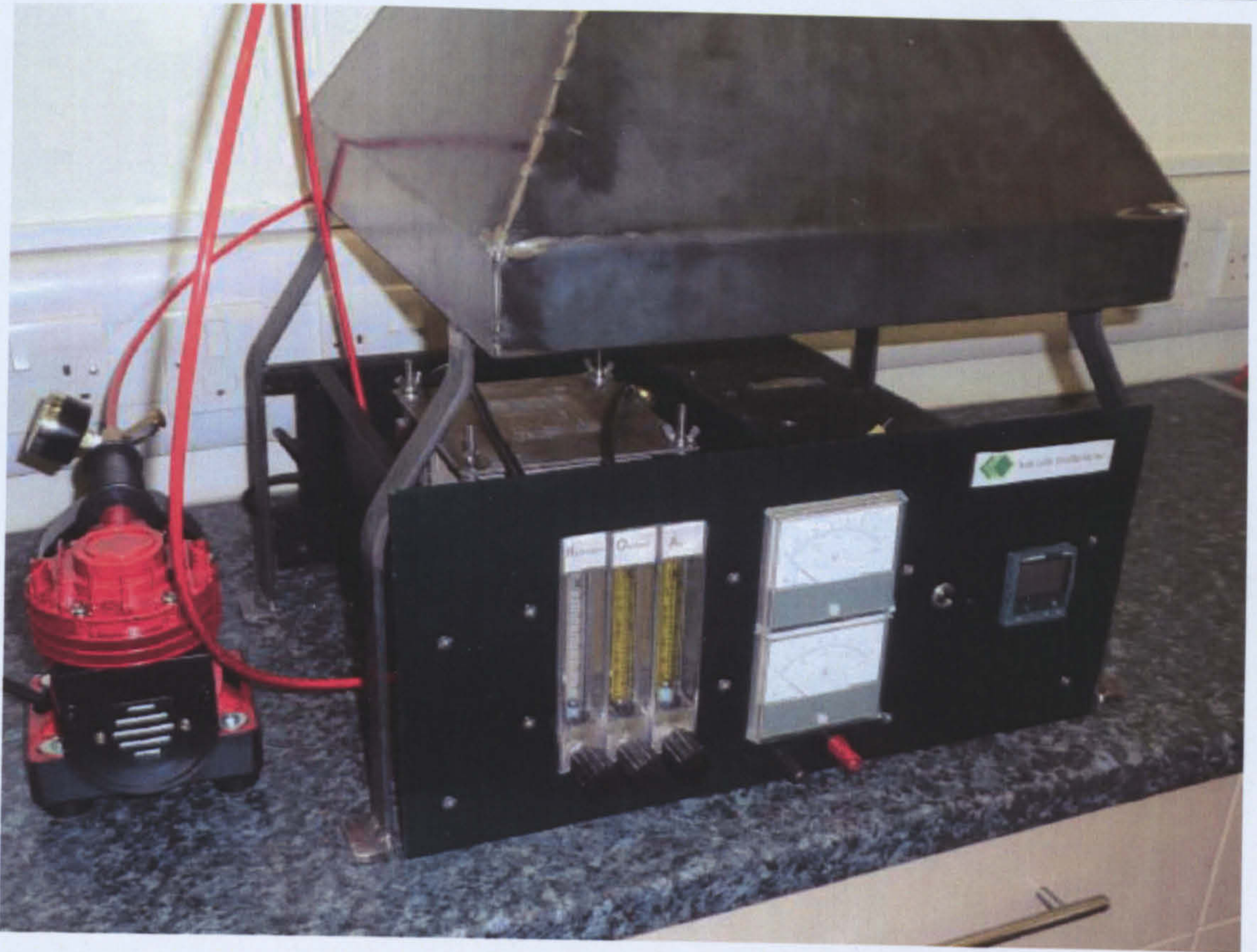
Figure A.15.6 Prototype solid oxide fuel cell used for research work and air compressor to supply air to fuel cell stack.
