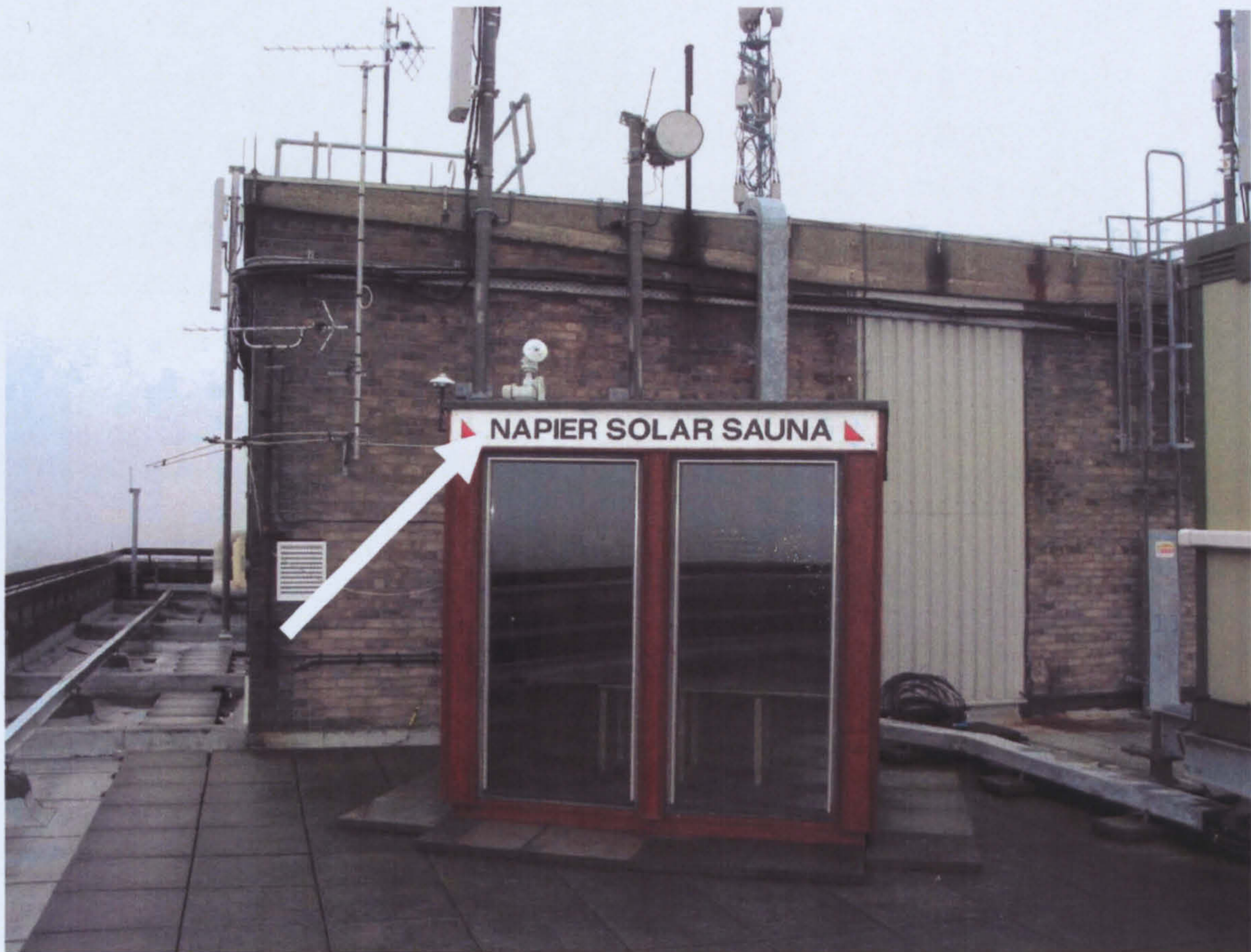
Figure. 3.4.1 Edinburgh Napier University solar measurement station on the rooftop of Edinburgh Napier University. Note the building behind the measurement station, found to cause errors in measuring the diffuse component of some global irradiance.
