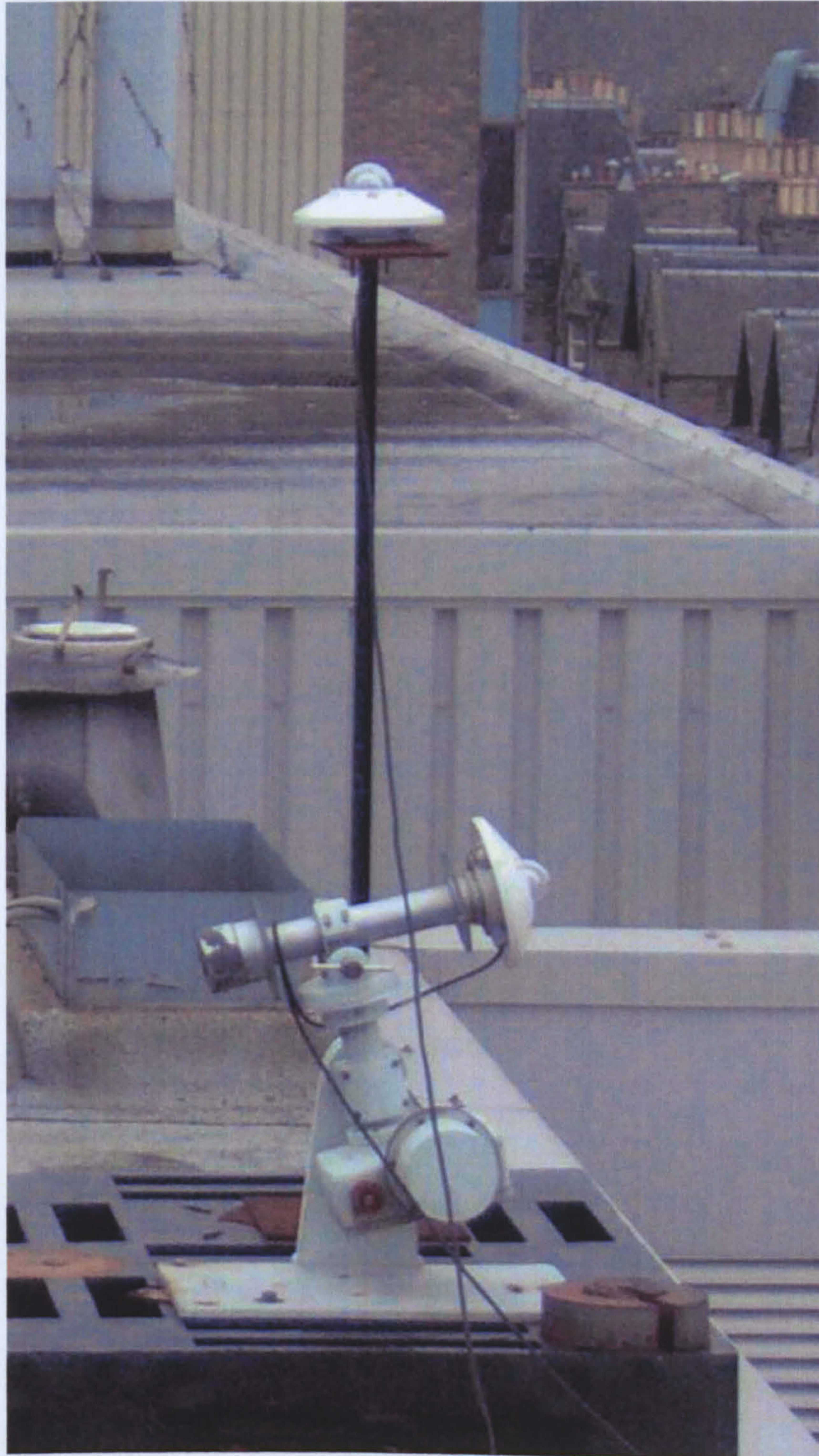
Figure 2.8.1 Horizontal and inclined pyranometers at Edinburgh Napier University test site.
