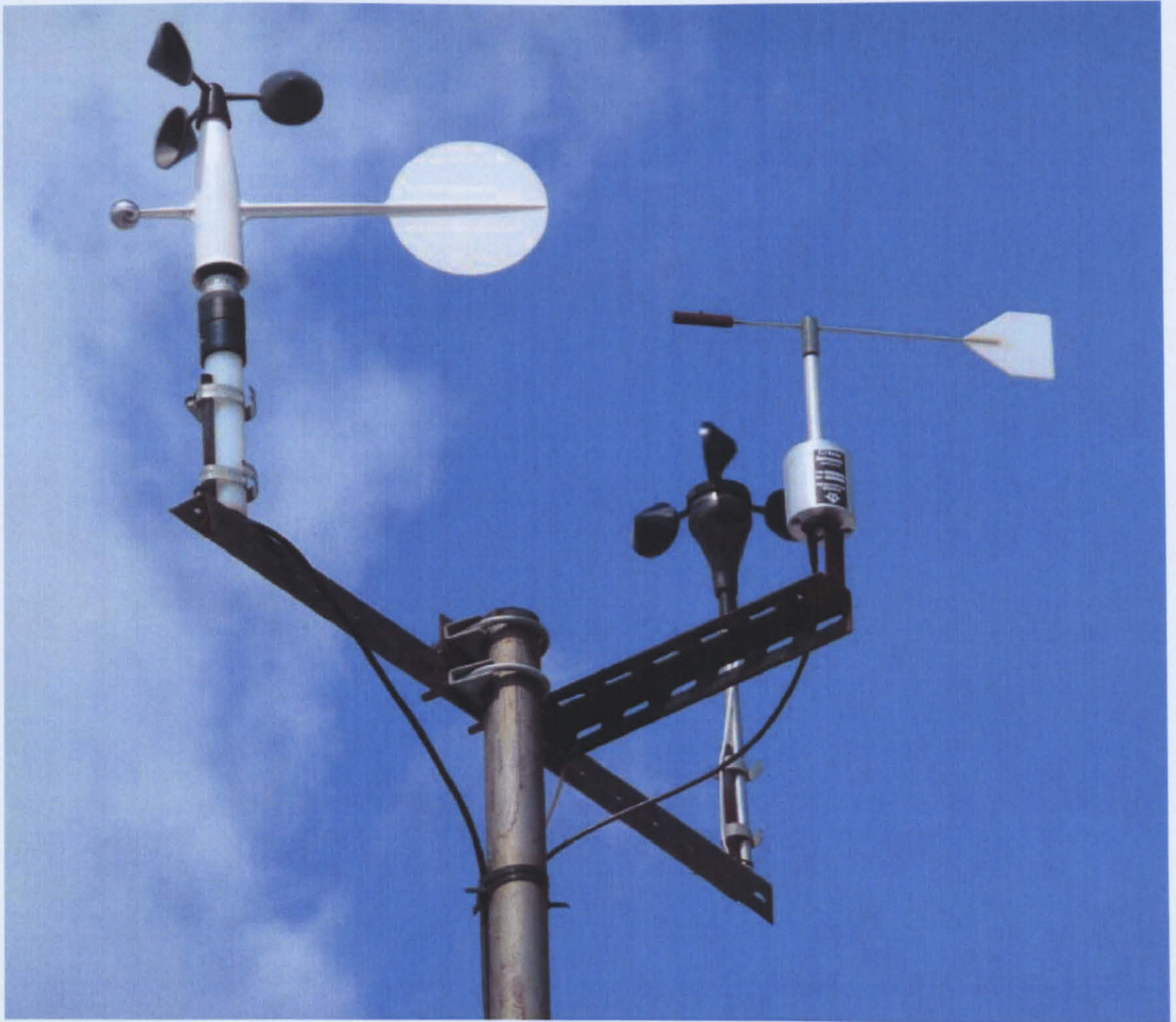
Figure 2.22.1 Two wind velocity anemometers and two wind direction vanes (Wind monitoring station, Edinburgh Napier University).
