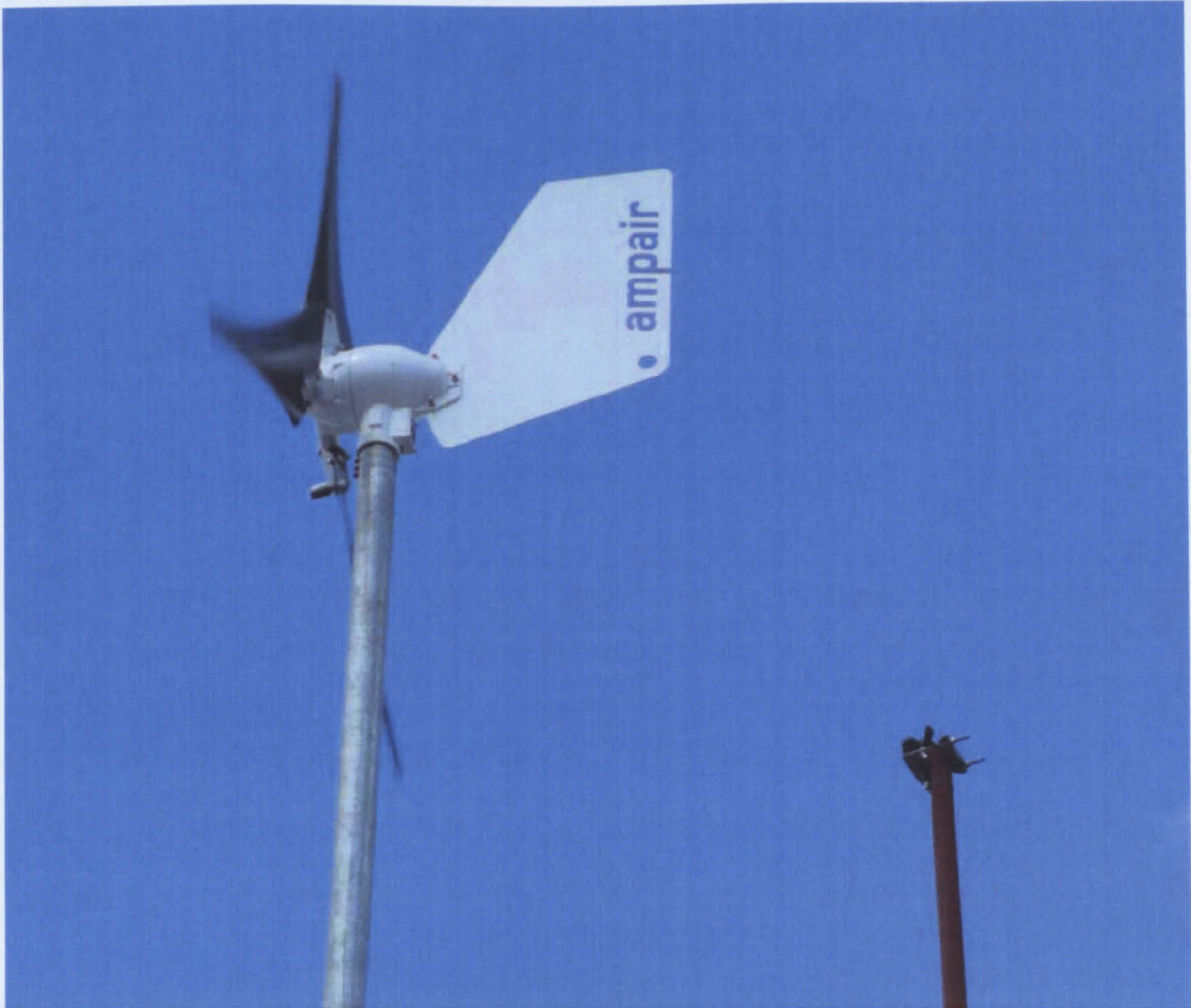
Figure 6.2.2.1 Ampair 600-230 V, anemometer can be seen to the right (Edinburgh Napier University).
