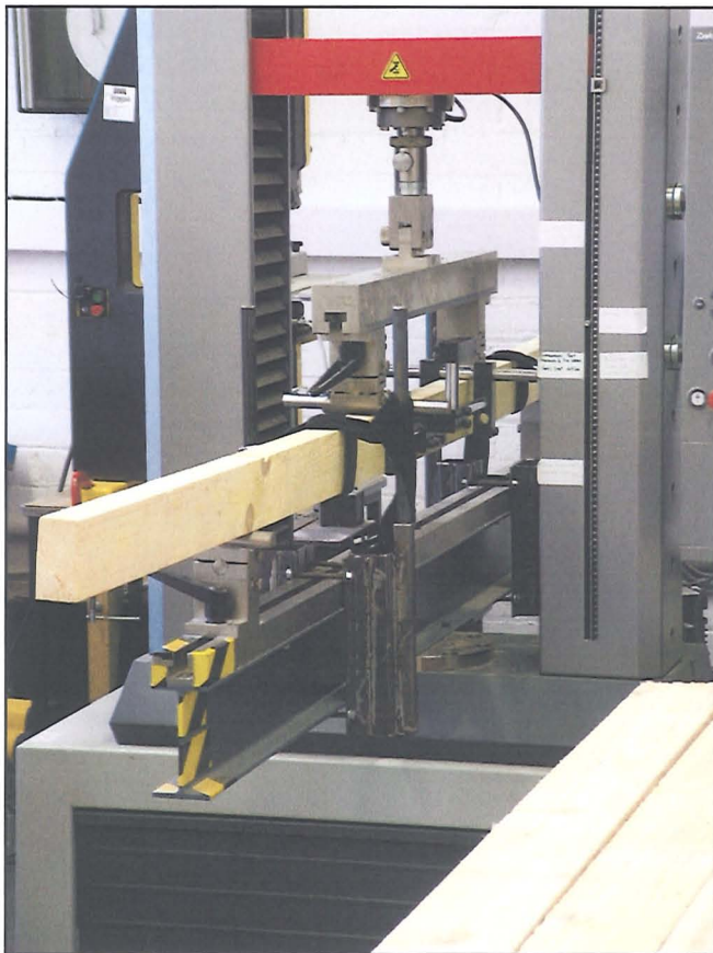
Figure 6.10 Zwick 205D universal testing machine set up for four-point bending test
