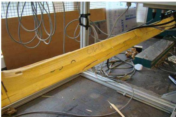
*Figure 9: A typical NSC16 batten ruptured under torsion loading with horizontal shear crack*
