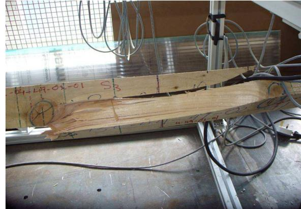
*Figure 7: A typical combined tension shear failure occurred in 2.8m specimen due to top and bottom edge knots*
