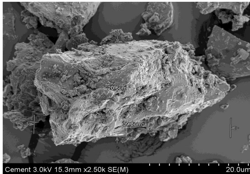
**Fig. 4.10** SEM image of cement specimen
