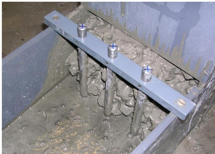
**Fig 8.6** Blockages behind reinforcing bars
