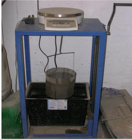
**Fig. 4.6** Density testing apparatus (weight-in-air, weight-in-water method)
