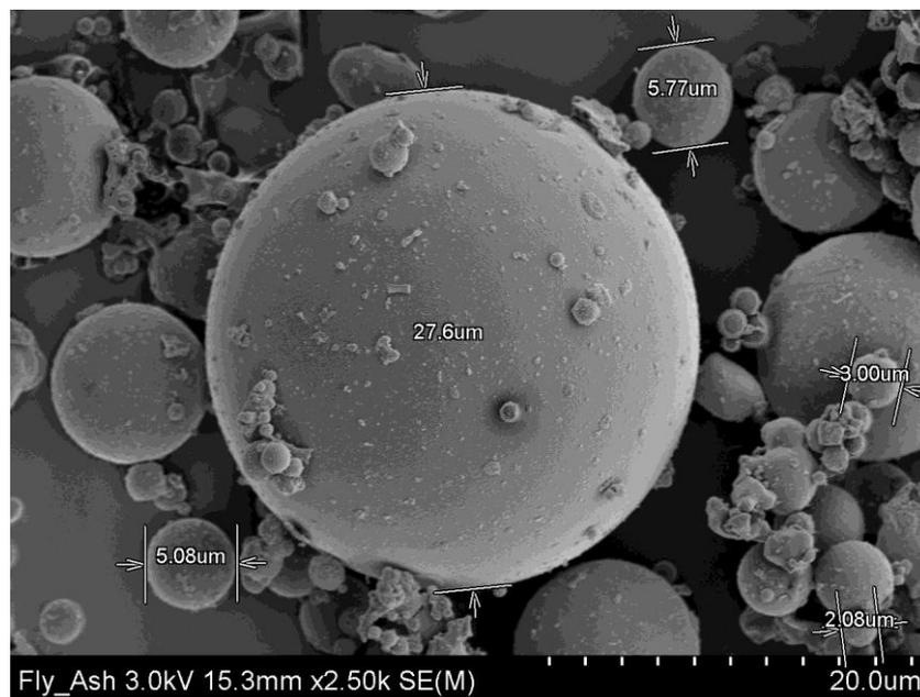
**Fig. 4.12** SEM image of PFA specimen
