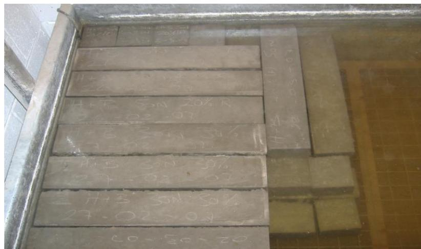
**Fig. 7.1** Beams and cubes kept in water tank at  $20 \pm 2^\circ\text{C}$
