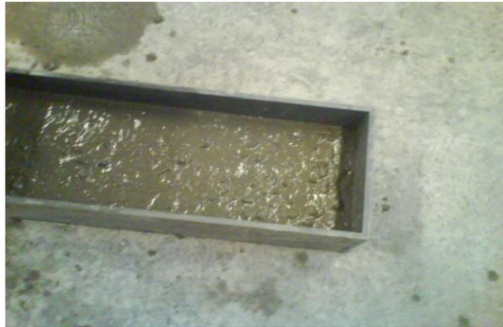
**Fig. 8.5** Concrete flow into the bottom tank of the L-box
