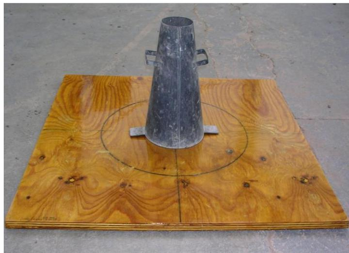
**Fig. 8.2** Slump cone located on the inner circle above the base plate
