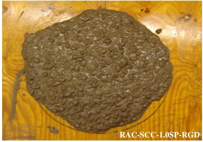
**Fig. 8.7** Concrete failing the flow test
