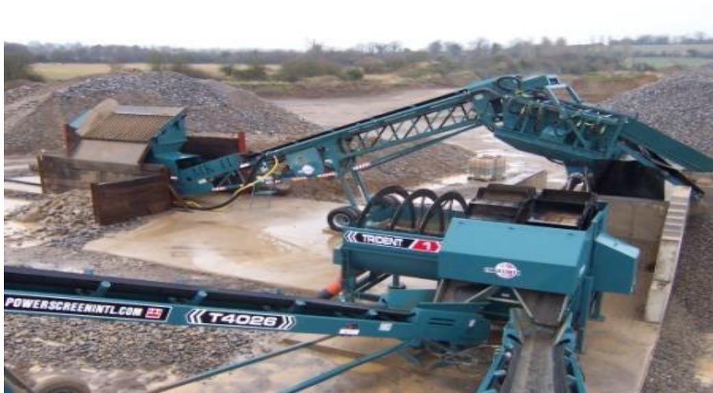
**Fig. 2.12** Aggregate screen
