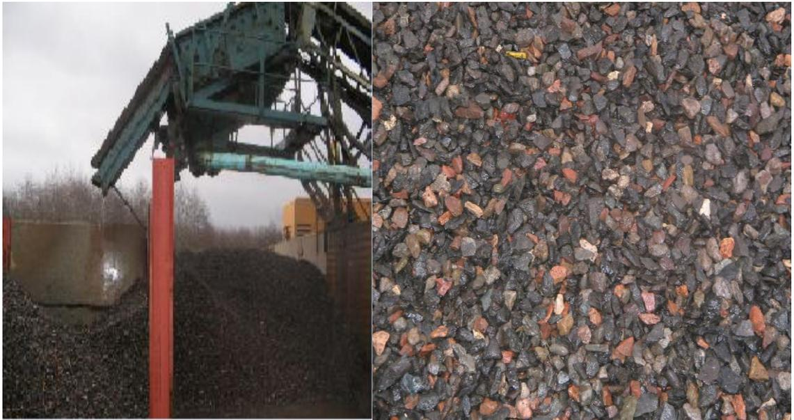
**Fig. 2.14** Removing fines by washing with water
