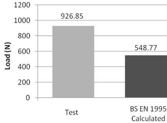
**Figure 8** Characteristic headside pull through of 2.65x60mm annular shank nail through 21.5x120mm Scots pine cladding
