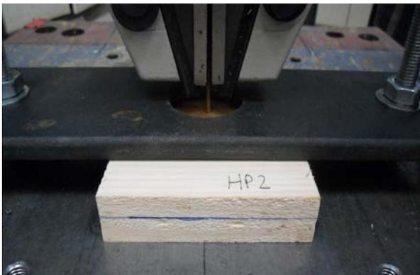
**Figure 3** Pull through scots pine cladding test
