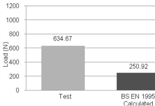
**Figure 7** Characteristic pointside withdrawal of 2.65x60mm annular shank nail from 38.5mm penetration into a timber cross batten
