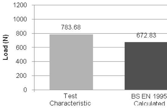
**Figure 5** Characteristic pointside withdrawal of 3.1x90mm smooth shank nail from 25x50mm vertical timber batten, 9mm OSB and 45x145mm timber stud
