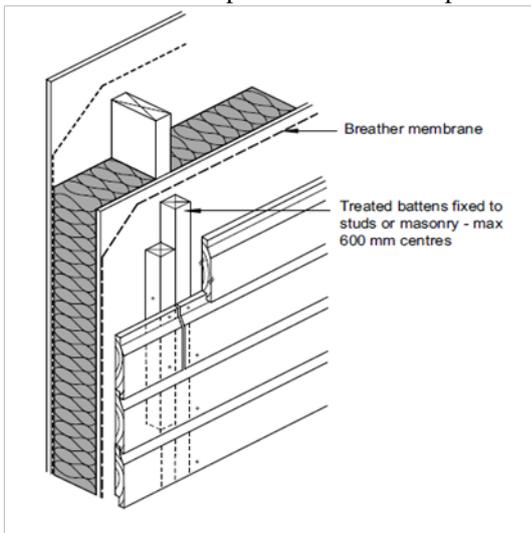
**Figure 1** Horizontal cladding boards (3)
