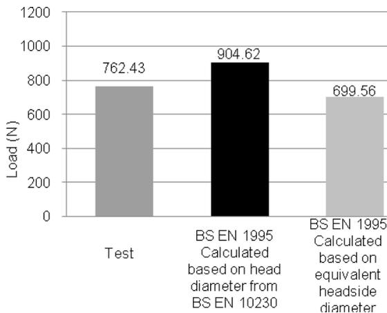
**Figure 6** Characteristic headside pull through of 3.1x90mm smooth shank nail through 38x50mm counter timber batten
