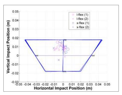
Figure 44: Typical example for impact positions recorded for one player. Club number (1) and (2) refer to the first and second data set recorded.
