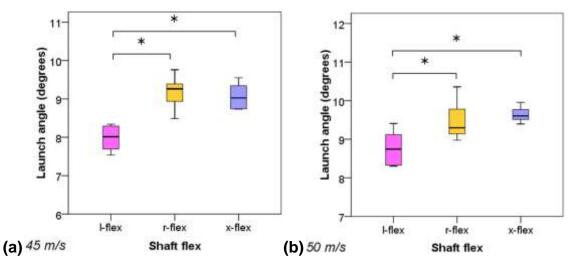
Figure 63: Launch angles measured for club head speeds of 45 m/s (a) and 50 m/s (b). Shaft pairs with significant differences are marked with '\*'.
