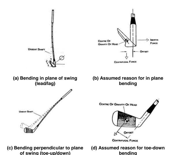
Figure 2: Definition of bending planes and suggested reasons for bending (adapted from Horwood, 1994, p. 249 and 251).
