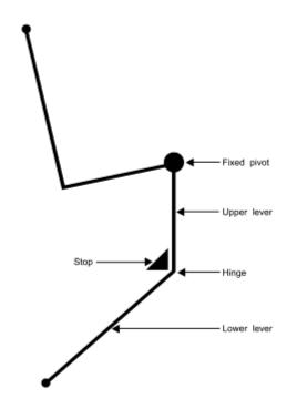
Figure 13: Double-pendulum model of the golf swing (adapted from Cochran & Stobbs, 1968).
