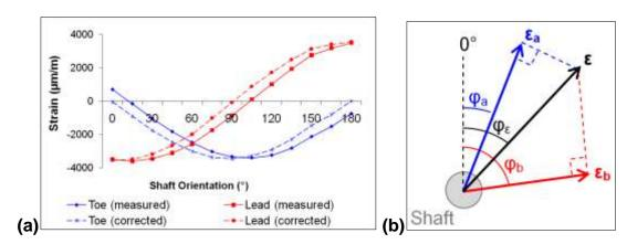
Figure 25: (a) Example results from strain gauge calibration. (b) Shaft cross section with nomenclature for calibration procedure.
