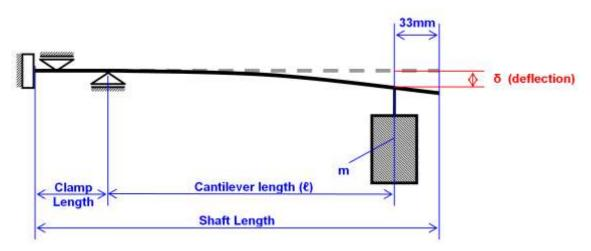
Figure 20: Set-up of rigidity test.
