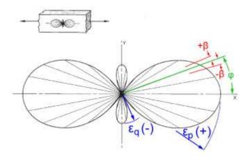
Figure 24: Strain field created by a uniaxial stress field.  $\varepsilon_p$  and  $\varepsilon_q$  denote the maximum and minimum principal strains,  $\varphi$  is the intended alignment angle of the strain gauge and  $\beta$  is the alignment error (mod. from Vishay, 2007).
