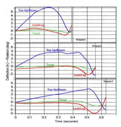
Figure 16: Three different shaft deflection profiles. 'One-peak' (top), 'double-peak' (middle) and 'ramp-like' (bottom) (mod. from Butler & Winfield, 1994, pp. 261-262). Positive values correspond to toe-up, lead and face-close deflection, negative values to toe-down, lag and face-open deflection<sup>7</sup>.
