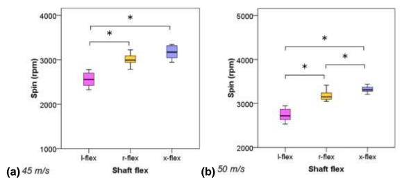
Figure 64: Spin rates measured for club head speeds of 45 m/s (a) and 50 m/s (b). Shaft pairs with significant differences are marked with '\*'.
