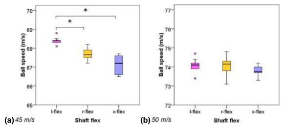
Figure 62: Ball speeds measured for club head speeds of 45 m/s (a) and 50 m/s (b). Shaft pairs with significant differences are marked with '\*'.
