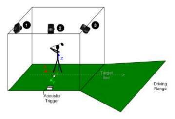
Figure 27: Setup of custom club head tracking system (cameras: **0-8**).
