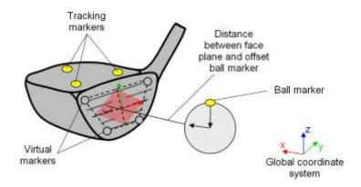
Figure 28: Definition of face plane and distance to offset ball maker.
