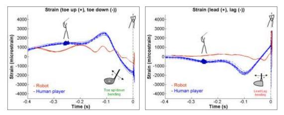
Figure 57: Comparison of human and robotic shaft loading for two clubs with identical stiffness ratings (x-flex). Stick figures indicate the time of the transition from backswing to downswing and impact for the human player.
