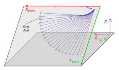
Figure 41: Planar projection of the club path to determine grip angle and angular velocity at impact.
