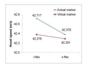
Figure 47: Interaction of speed difference and shaft stiffness factors.
