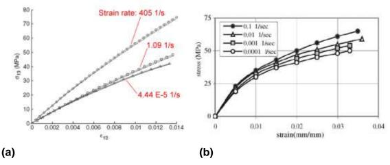
Figure 5: Stress(σ)-strain(ε) graphs for composites loaded at different strain rates: (a) based on micromechanical modelling (Zhu, Chattopadhyay, & Goldberg, 2006, p. 1810); (b) based on experimental results (Fereshteh-Saniee, Majzoobi, & Bahrami, 2005, p. 46).
