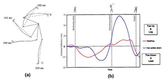
Figure 1: Shaft behaviour during a typical golf swing: (a) simulation of shaft bending according to Milne & Davis' (1992) measurements (bending exaggerated by a factor of 5) (adapted from Penner, 2003, p. 158); (b) bending of the shaft during a typical golf swing (adapted from Newman, Clay, & Strickland, 1997, p. 369).
