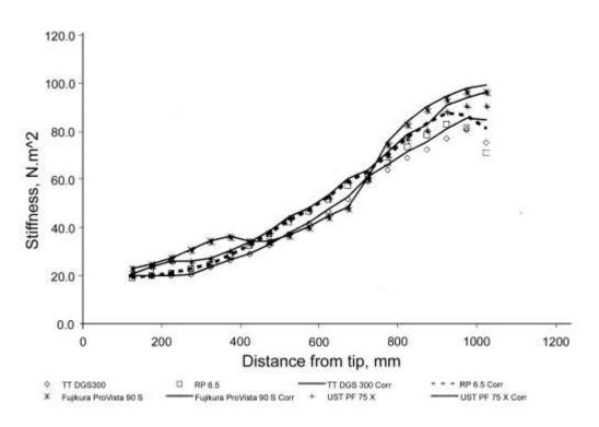
Figure 8: Stiffness profiles for four different golf shafts before and after applying a correction for measurement errors. It can be seen that each shaft has characteristic stiffness variations between tip and butt end (adapted from Mase, 2004, p. 520).
