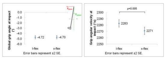
Figure 52: Estimated marginal means for the planar club angle and angular velocity. This angle was calculated after projecting the longitudinal axis of the grip on the x-z-plane (vertical) and is relative to the z-axis.
