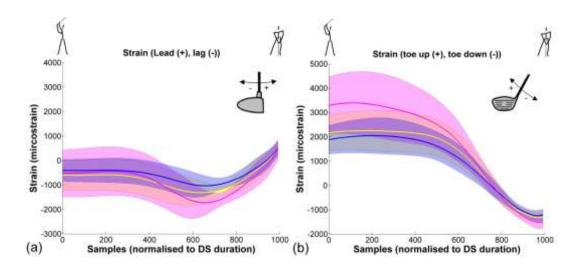
Figure 36: Mean strain patterns in lead/lag direction (a) and toe up/down direction (b). Lines represent mean strain for all subjects for the I-flex (pink), r-flex (yellow) and x-stiff (blue) shaft. Shaded areas indicate ±1 SD.
