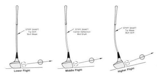
Figure 14: Expected effect of shaft stiffness distribution on launch angle (adapted from Maltby, 1995, p. 416).
