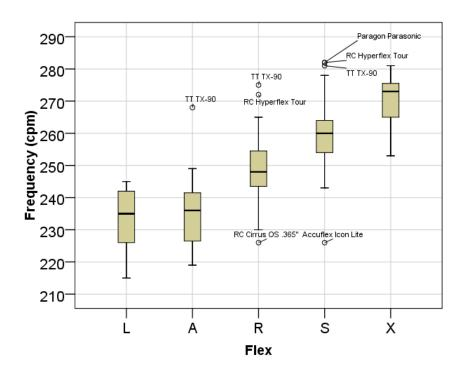
Figure 18: Boxplot showing driver shaft frequency ranges for different flex codes (based on data for 300 driver shafts presented by Summitt, 2000)
