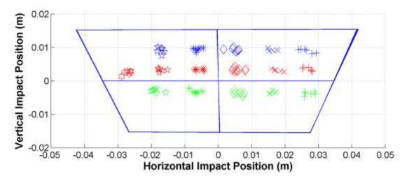
Figure 30: Face mapping results. The rows of grid points (blue, red, green) were separated by 6 mm, columns by 11 mm.
