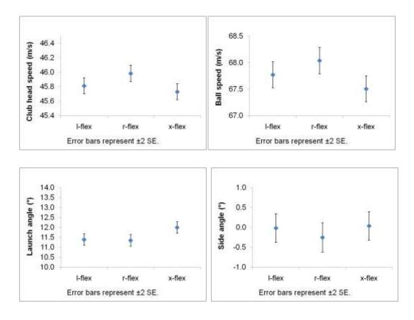
Figure 35: Estimated marginal means for different shaft conditions for the variables club head and ball speed, launch angle and side angle.
