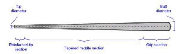
Figure 6: Typical shaft geometry (cross section). Shaft diameter is exaggerated relative to length for clarity (based on data presented in Huntley, 2007).
