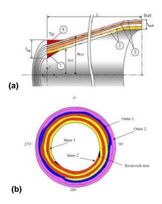
Figure 4: (a) Typical composition of a sheet-laminated shaft from a number of layers<sup>2</sup> of carbon/epoxy pre-pregs (adapted from Cheong, Kang, & Jeong, 2006, p. 469). (b) Resulting lay-up of carbon/epoxy layers. Fibres of the inner layer are typically oriented at ±45°, fibres of the outer layer at 0° (adapted from Huntley, 2007, p. 140).
