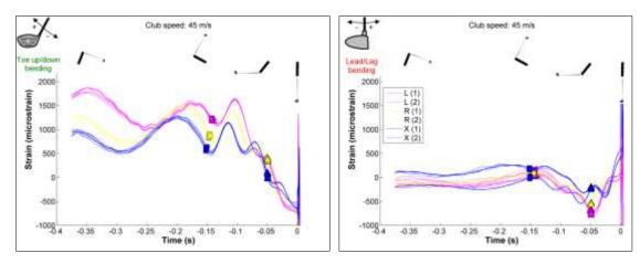
Figure 58: Strain patterns recorded for robot swings performed with an impact speed of approximately 45 m/s. Symbols indicate wrist release (□) and grip-horizontal event (△).Club numbers (1) and (2) refer to the first and second club replicate, respectively,
