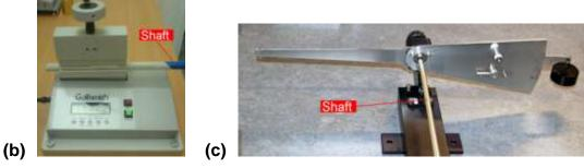
Figure 10: Commercial shaft test equipment. (a) Deflection board (Maltby Design, USA), (b) Frequency analyser (Golfsmith, USA), (c) Torsion test (Golfmechanix, Taiwan ROC).
