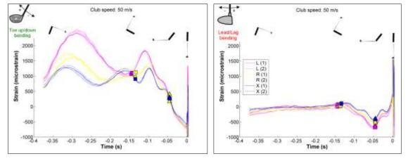
Figure 59: Strain patterns recorded for robot swings performed with an impact speed of approximately 50 m/s. See previous figure for details.
