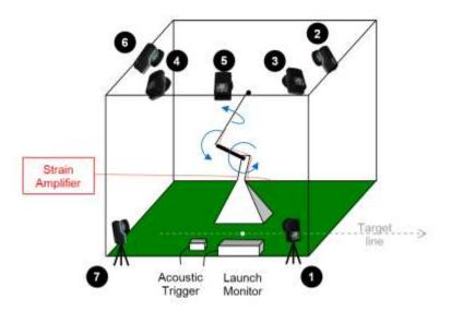
Figure 53: Setup for robot testing. **0-6** denote motion capture cameras.
