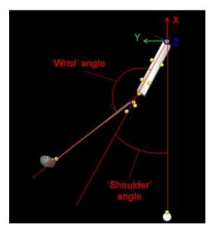
Figure 55: Definition of shoulder and wrist angle for the golf robot. The z-axis of the global coordinate system runs perpendicular to the arm.
