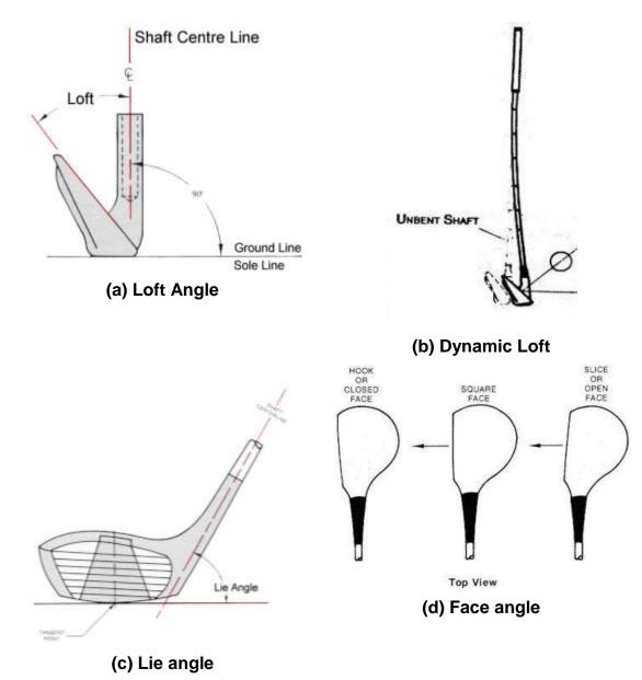
Figure A-1: Definitions of basic club head parameters: (a) loft angle (Maltby, 1995, p. 406), (b) effect of shaft bending on dynamic loft (Horwood, 1994, p. 249), (c) lie angle (Maltby, 1995, p. 418), (d) face angle (Maltby, 1995, p. 434).
