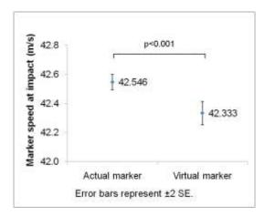
Figure 46: Estimated marginal mean speed for the hosel marker as measured directly with the motion capture system and as calculated for a virtual marker.
