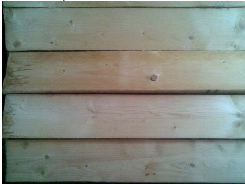
Figure 15. The results of 3.0 cm x 15.0 cm pine boards ( Pinus L. ) drying process using gas-steam mixture (fractures and colour changes of wood).
