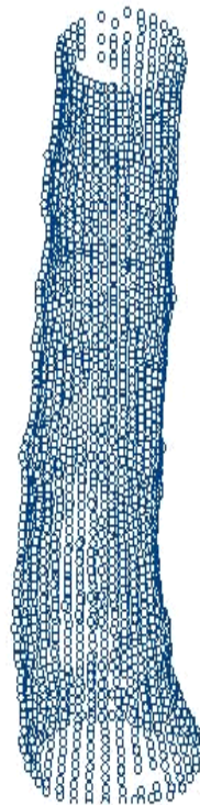
Figure 1: Log shape data obtained from industrial 3D laser scanner, from which variables such as Log taper were obtained.
