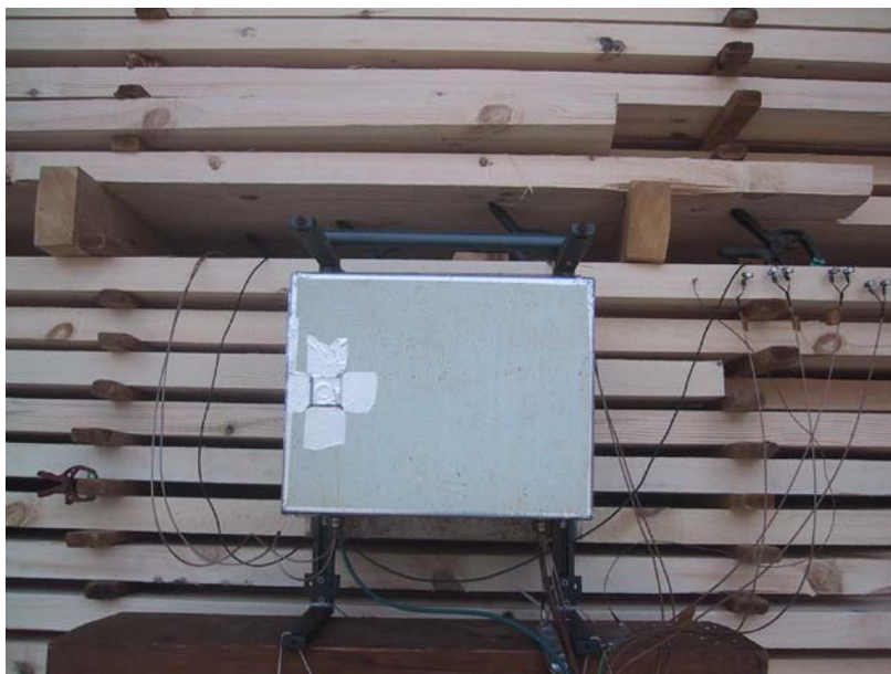
Figure 2. The combined AE and EIS measurement system was installed in an industrial drying kiln. The heat insulated and cooled box contains AE preamplifiers and the impedance modules. The pin electrodes were used for reference MG measurement using commercial resistance moisture meter.
