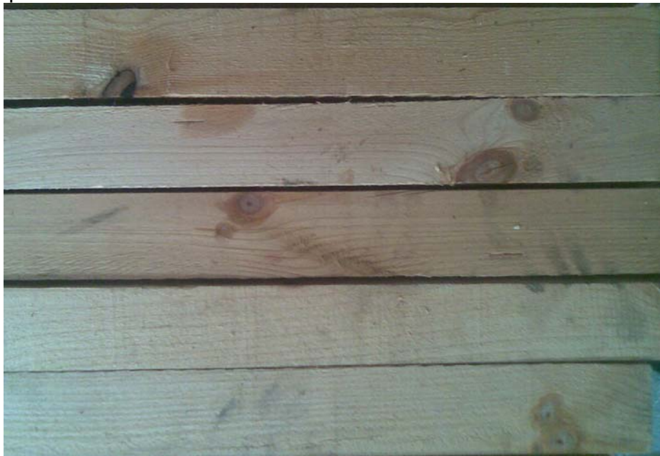
Figure 13. The results of 7.0 cm x 7.0 cm pine lumber ( Pinus L. ) drying process using gas-steam mixture (fractures and colour changes of wood).
