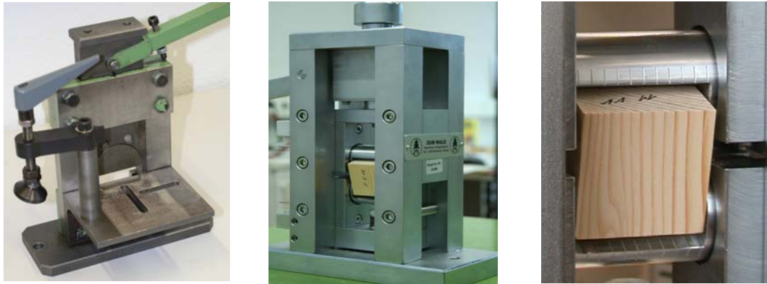
Figure 6: EN 392 type shearing tool (left), new test apparatus (center), close view of a specimen during testing with the new apparatus (right)
