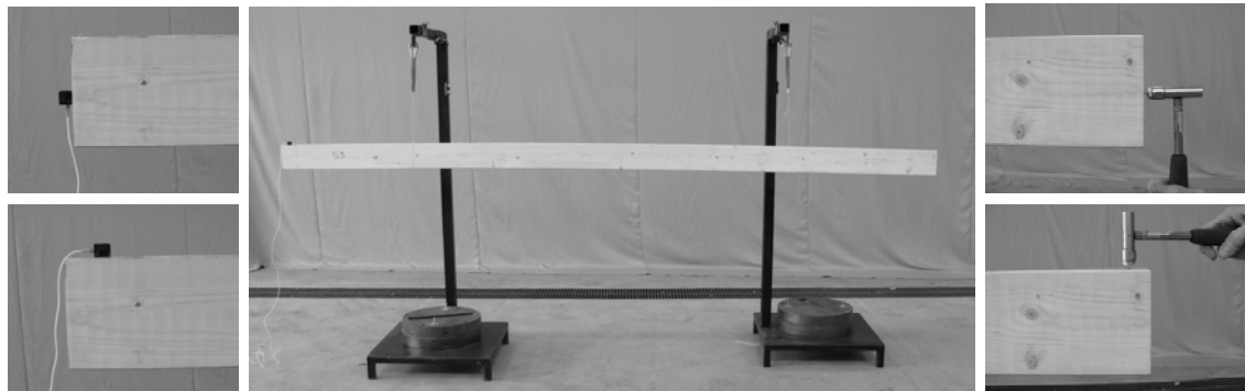
Figure 1: Test setup for assessment of dynamic MOE.
