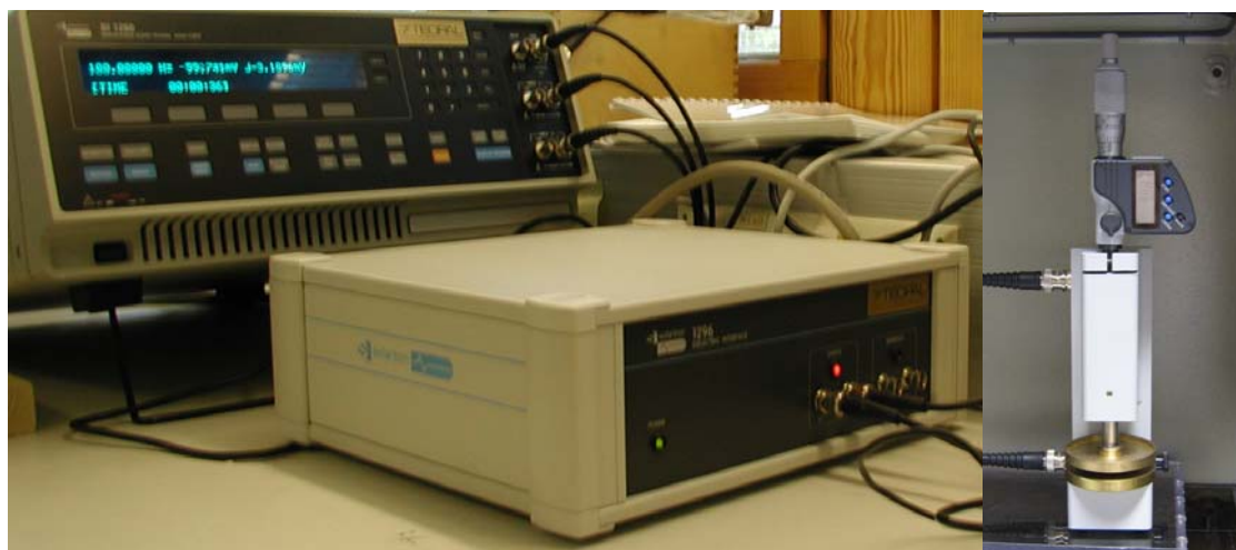
Figure 2. The impedance analyser with the dielectric interface (a) and the sample holder (b).
