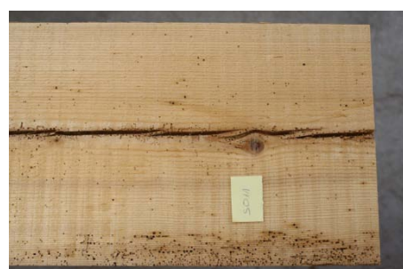
Figure 3: Damage due to insect attack
