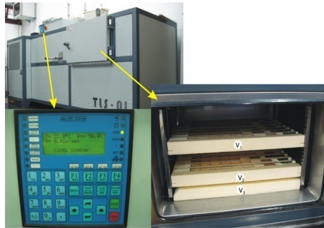
Figure 2: Conventional drying tunnel TLS-01 (top-left) with PLC controller (bottom-left) and experimental chamber with holding isolative shelves and drying specimens (bottom-right).
