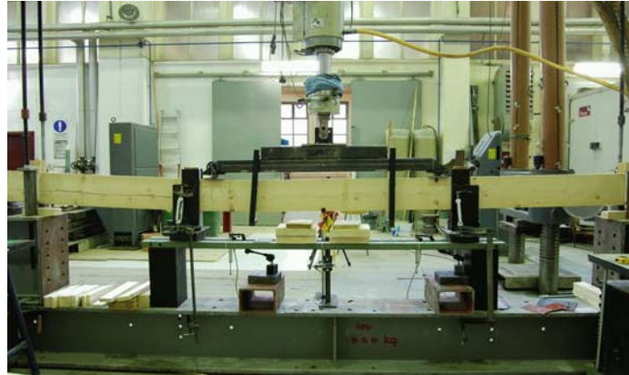
Figure 4: Destructive tests of boards 44 x 210 mm with lateral restraints
