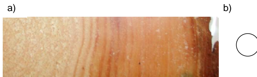
Figure 1. A crosscut sample before separating the heartwood and sapwood (a). The circle (b) represents the size of the electrode ( \varnothing 10 mm) compared to the specimen (from pith to bark about 95 mm).
