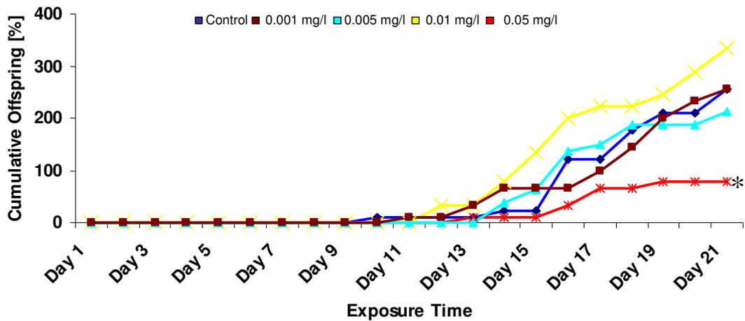
Figure 3.47: Cumulative offspring during a 21 day exposure to micro sized (average size 600-1600 nm) silver ( $n = 10$ ) (\* indicates a result with  $p \leq 0.05$ ).
