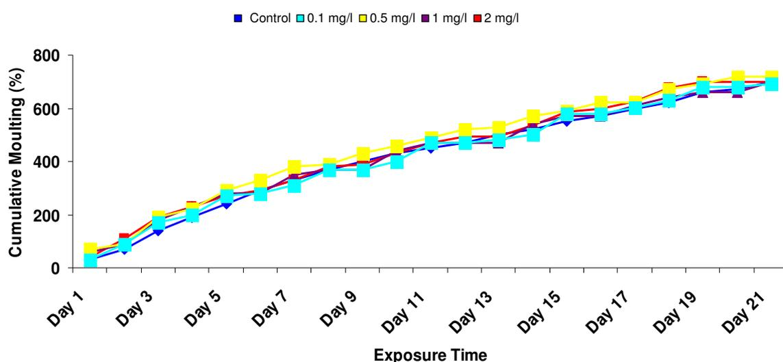
Figure 3.26: Cumulative moulting in a 21 day exposure to micro sized (average size 260 nm) carbon black (n= 10 per treatment). No significant reduction in the cumulative moulting between treatments was observed.
