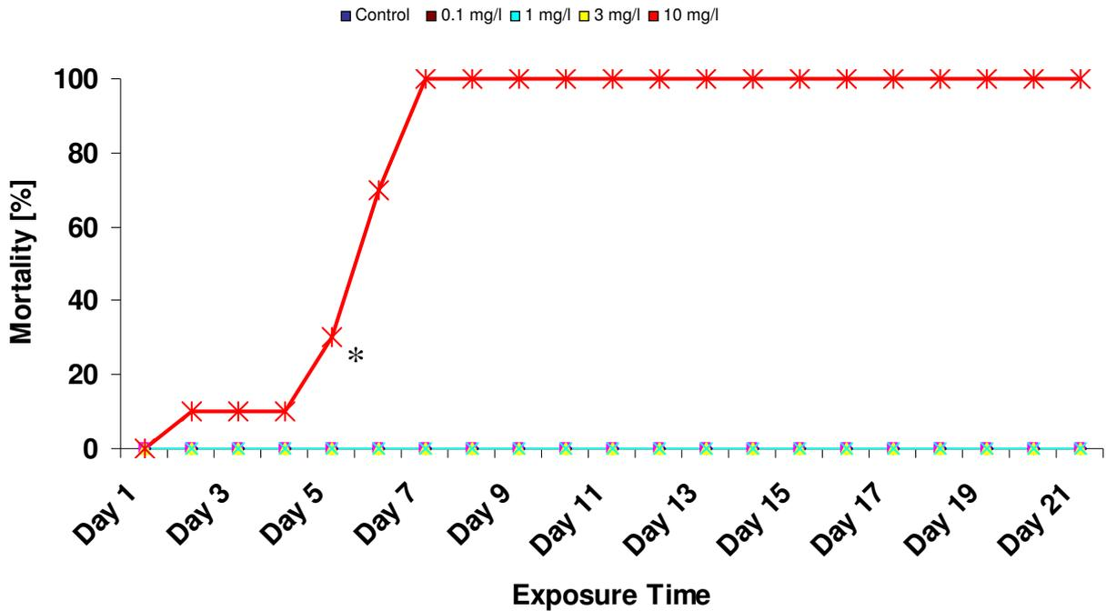
Figure 3.33: Mortality in a 21 day exposure to nano sized (average size <25 nm) cerium dioxide (n= 10) (\* indicates a result with  $p \leq 0.05$ ).
