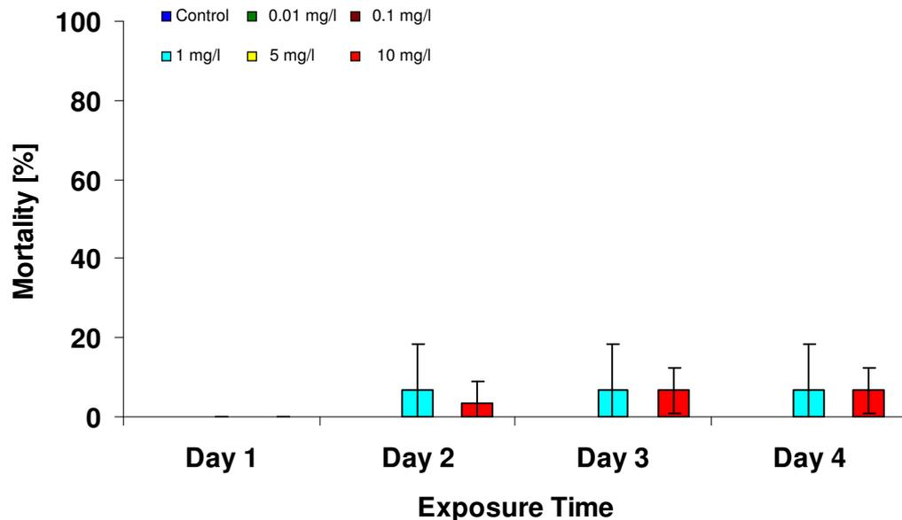
Figure 3.11: Mortality in a 96 h exposure to micro sized (average size 260 nm) carbon black (0.01 mg/L n= 10; 5 mg/L n= 20; otherwise n= 30, values are means +/- standard error). No significant mortality was observed.
