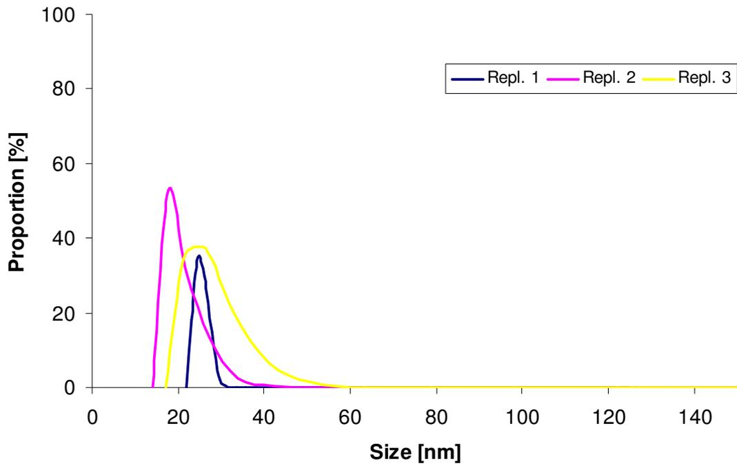
Figure 4.1: Size distribution of 20 nm polystyrene beads in water (2  $\mu\text{g/L}$ ) after 0 h. Shown are the three different replicates that were measured independently at each time point
