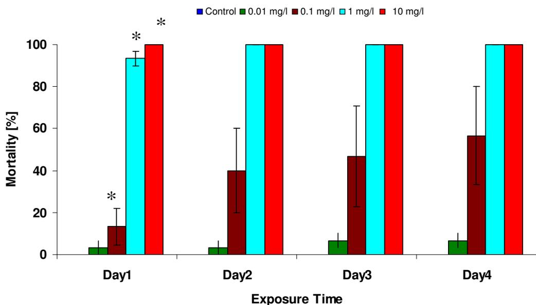
Figure 3.22: Mortality in a 96 h exposure to nano sized (average size 35 nm) silver (n=30, values are means +/- standard error, \* indicates a result with  $p \leq 0.05$ ). Since the data had no homogenous variances, a non parametric post hoc test was used.
