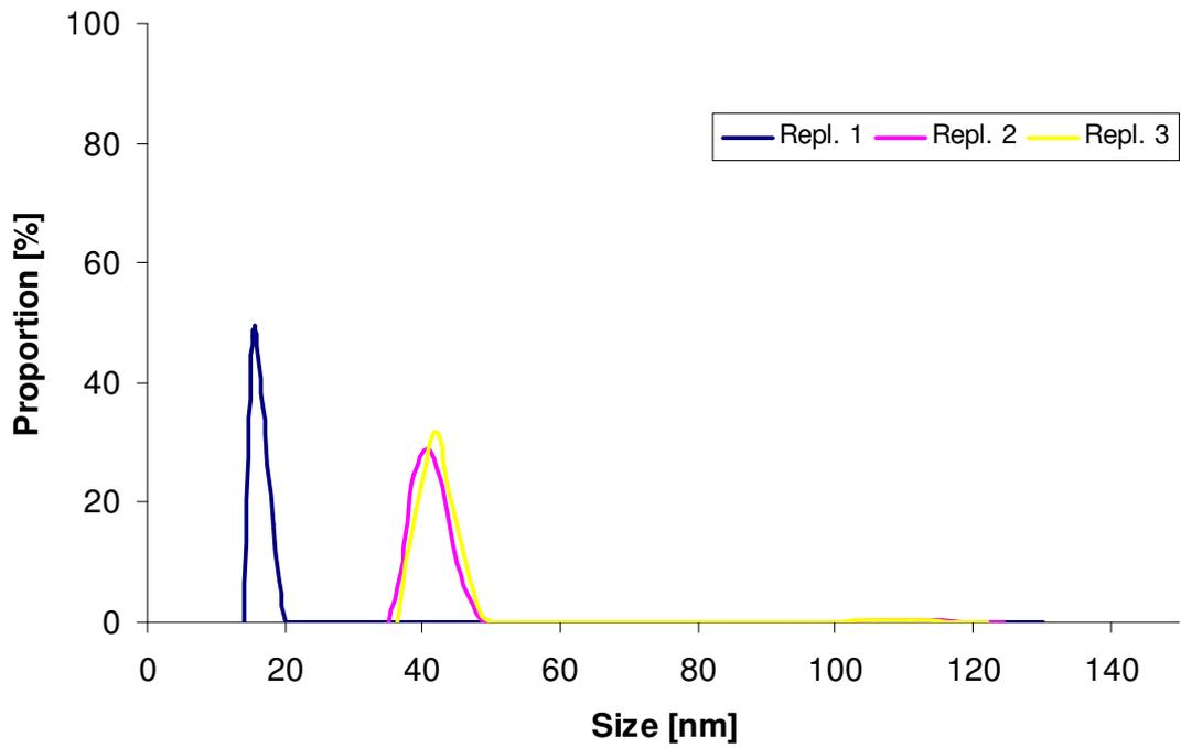
Figure 4.3: Size distribution of 20 nm polystyrene beads in water (2  $\mu\text{g/L}$ ) after 2 h. Shown are the three different replicates that were measured independently at each time point.
