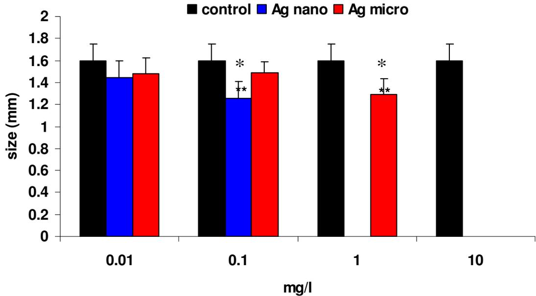
Figure 3.25: Size measurement to determine growth after a 96 h exposure to nano (average size 35 nm) and micro (average size 600-1600 nm) sized silver (micro 0.01 mg/L n= 27; 0.1 mg/L n= 26; 1 mg/L n= 6 and nano 0.1 mg/L n= 12; 0.01 mg/L n= 28; pooled control from nano and micro exposure n= 34; values are means +/- standard error, \* indicates a result with  $p \leq 0.05$ ).
