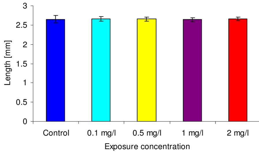
Figure 3.28: Size measurement to determine growth after a 21 day exposure to micro (average size 260 nm) sized carbon black (control, 1 mg/L and 0.5 mg/L n= 10; 0.1 mg/L, 2 mg/L n= 8; values are means +/- standard error).
