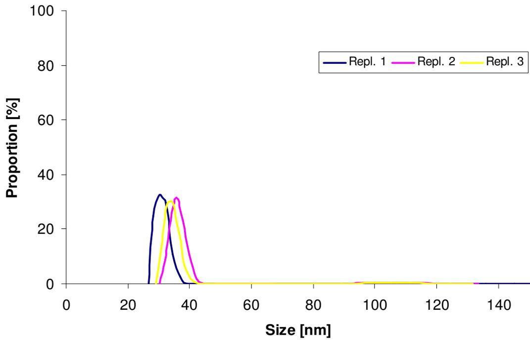
Figure 4.5: Size distribution of 20 nm polystyrene beads in water (2 µg/L) after 4 h. Shown are the three different replicates that were measured independently at each time point.
