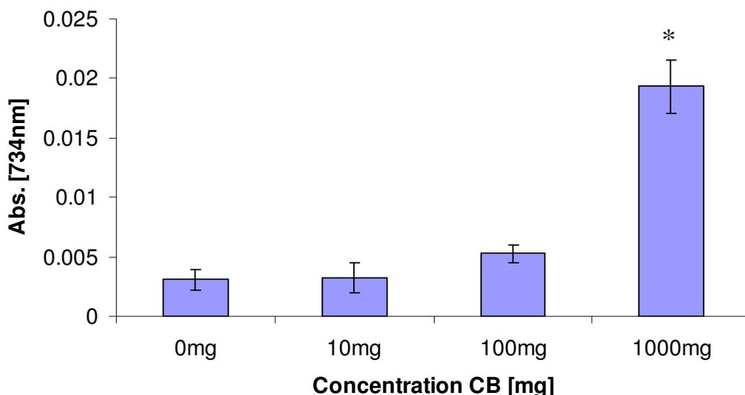
Figure 5.3: Absorbance comparison of several carbon black concentrations (n =3 per treatment, values are means +/- standard error, \* indicates a result with  $p \leq 0.05$ ).
