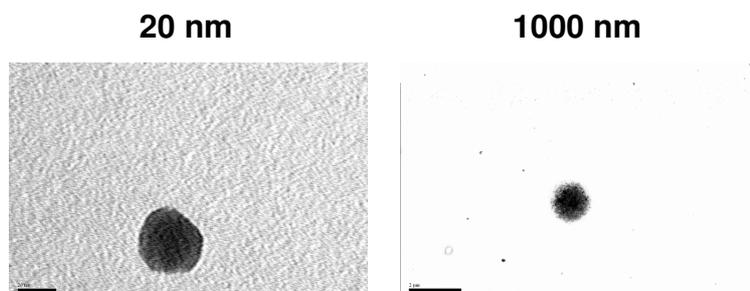
Figure 4.19: Transmission electron microscopy pictures of a 20 nm polystyrene bead (left) and a 1000 nm polystyrene bead (right). The black bar represents on the left hand side 20 nm and on the right hand side 2  $\mu\text{m}$ .
