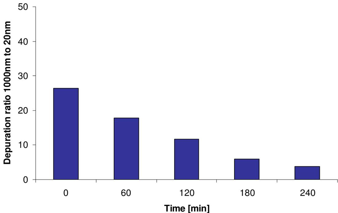
Figure 4.14: Comparison of depuration of 1000 nm polystyrene beads against the depuration of 20 nm polystyrene beads over a period of 4 h. Compared are the means of uptake at the various time points.
