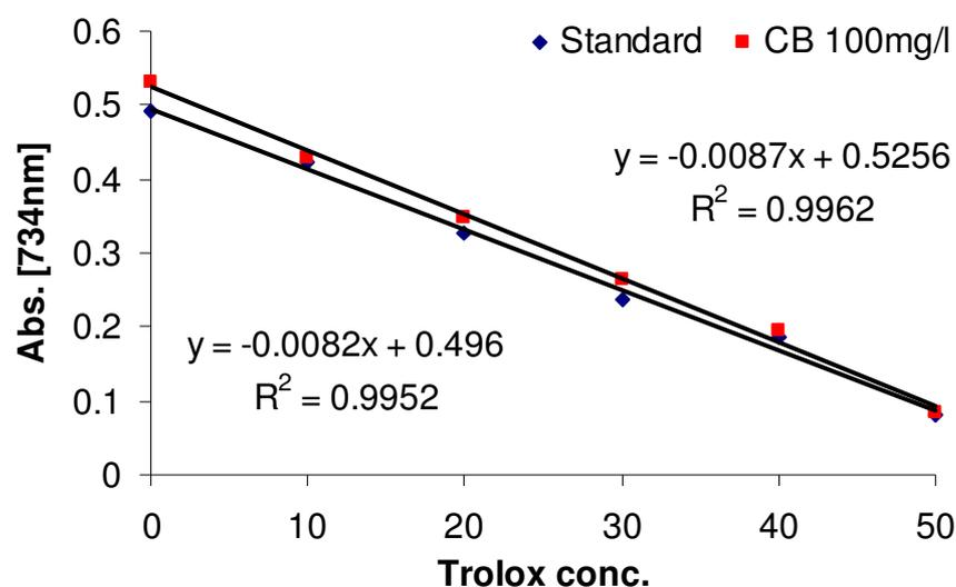
Figure 5.2: Comparison of a normal standard curve with a standard curve containing 100 mg/L carbon black. The equation of the normal standards and the R<sup>2</sup> value are below, while for the carbon black they are on top
