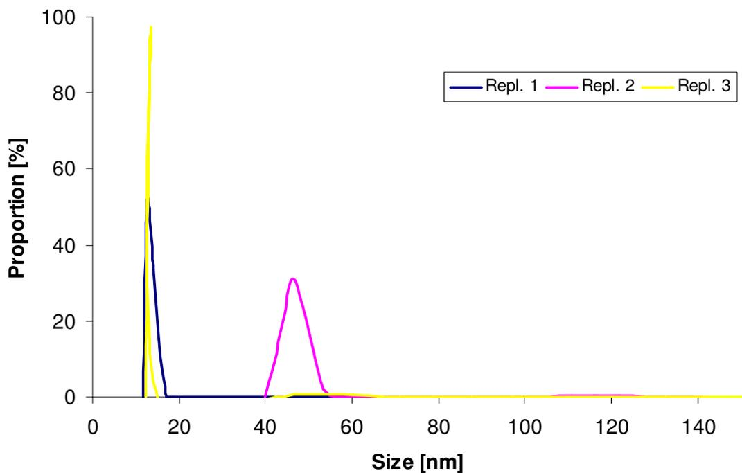
Figure 4.4: Size distribution of 20 nm polystyrene beads in water (2  $\mu\text{g/L}$ ) after 3 h. Shown are the three different replicates that were measured independently at each time point.
