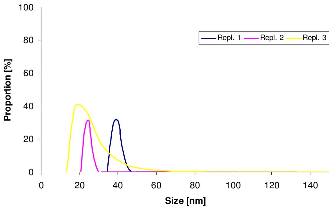
Figure 4.2: Size distribution of 20 nm polystyrene beads in water (2  $\mu\text{g/L}$ ) after 1 h. Shown are the three different replicates that were measured independently at each time point.
