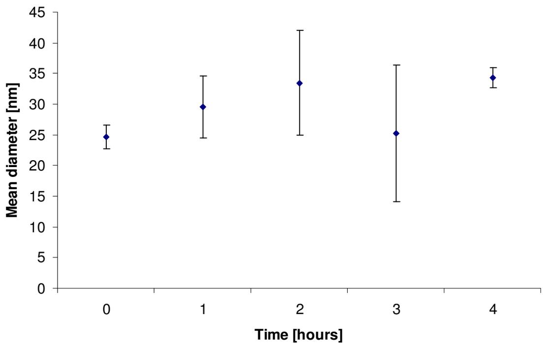
Figure 4.6: Mean diameter of 20 nm polystyrene beads in water (2 µg/L) over a time period of 4 h (values are means +/- standard error).
