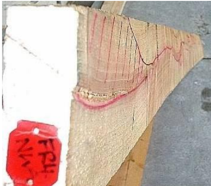
Figure 4.4: Batten FR4- NWA with wandering pith, which bowed on drying (and also twisted).
