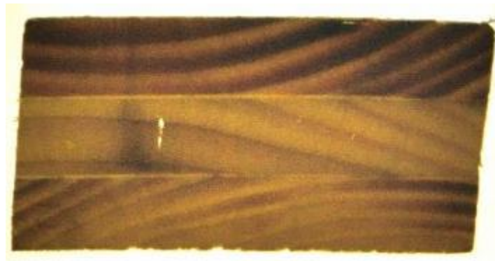
Figure 2.8: Section through distorted glue laminated timber showing compression wood in upper ply (by means of transmitted light on a thin section).
