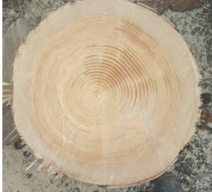
Figure 2.10: Compression wood noted in Sitka spruce foundation pile after driving.
