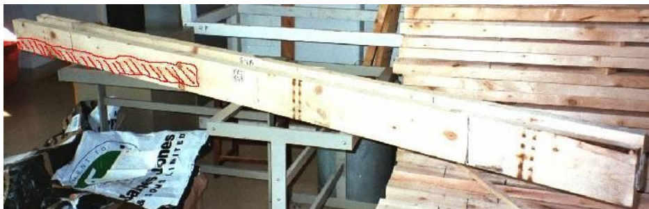
Figure 4.7: Battens reassembled, with compression wood shown hatched. (original in colour)
