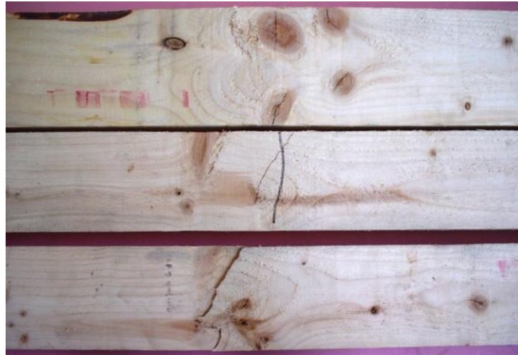
Figure 13.2: Machine grader rejects exhibiting severe cross grain with characteristic anomalous growth ring interception.
