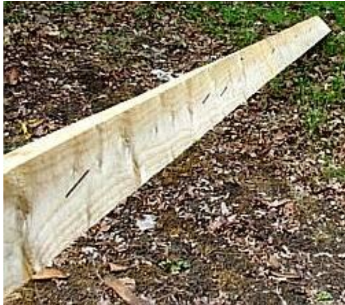
Figure 2.3: Slope of grain marked on a severely twisted batten containing pith.
