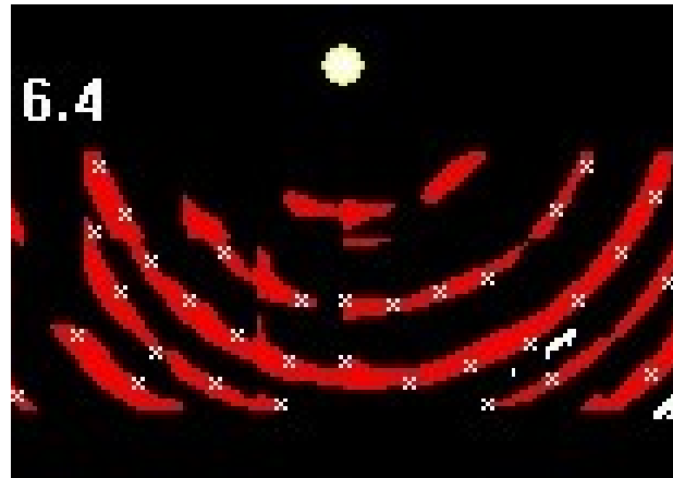
Figure 2.16: Processed image of board end showing ring width and pith position measurements.
