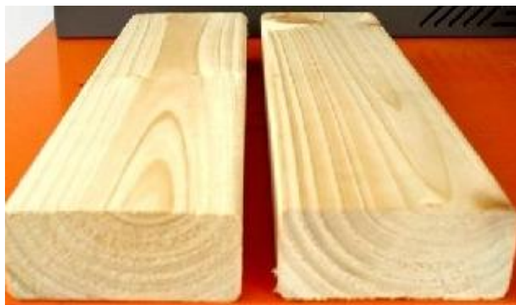
Figure 4.12: Compression wood in battens (darker bands). (original in colour).
