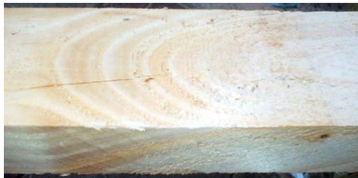
Figure 13.1: Batten with severe cross grain and associated compression wood.
