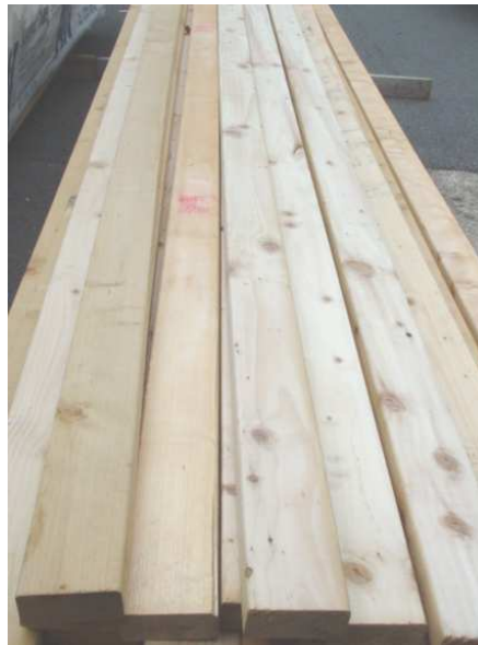
Figure 7. Battens used in timber frame panel manufacture. Imported timber (left), domestic (right).
