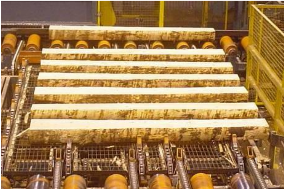
Figure 2.21: Canted logs presenting faces upon which knot content and spiral grain angle could potentially be measured.
