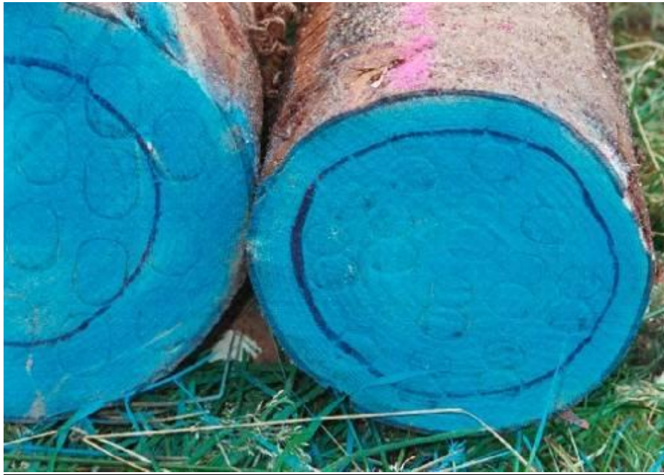
Figure 3.2: Log marking. Top (or upper end) of log is marked with an indented stamp and colour code. The 12th growth ring is also highlighted.
