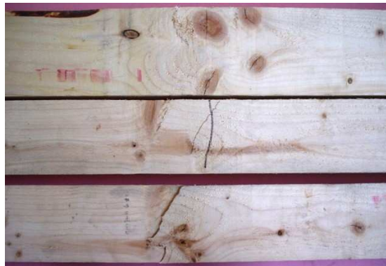
Figure 7. Machine grader rejects with severe cross grain.
