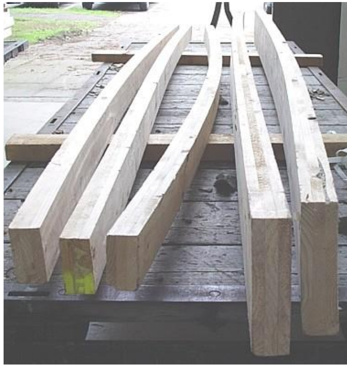
Figure 2.7: Glue laminated falling boards with pronounced bow on drying caused by compression wood in the outer plies.
