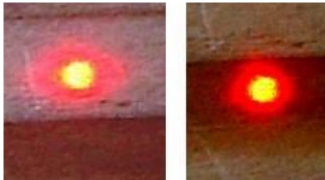
Figure 2.18: Laser tracheid effect, with normal wood (left), and compression wood (right). (original in colour)
