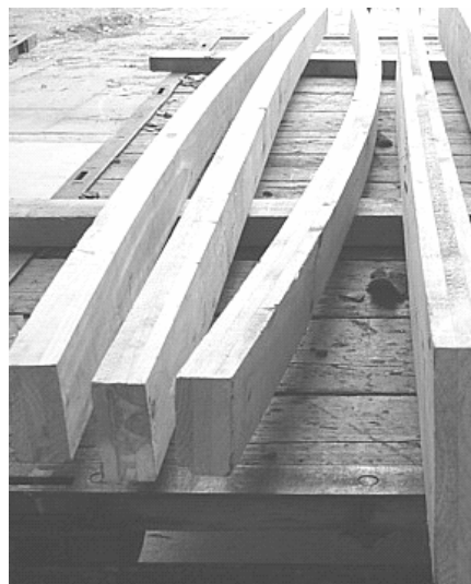
Figure 4. Bow of 3-ply glue-laminated elements caused by compression wood.
