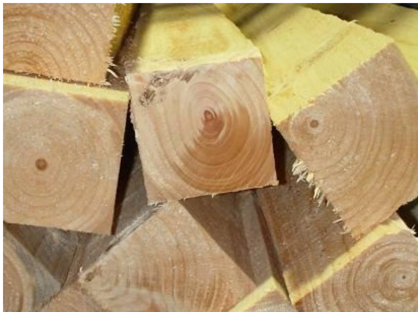
Figure 2.9: Compression wood in Sitka spruce fence post (centre). The growth ring structure suggests that the log was quite oval in section.
