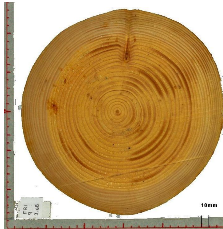
Figure 4.10: Log disc showing darker compression wood rings. (note image produced by Forest Research)
