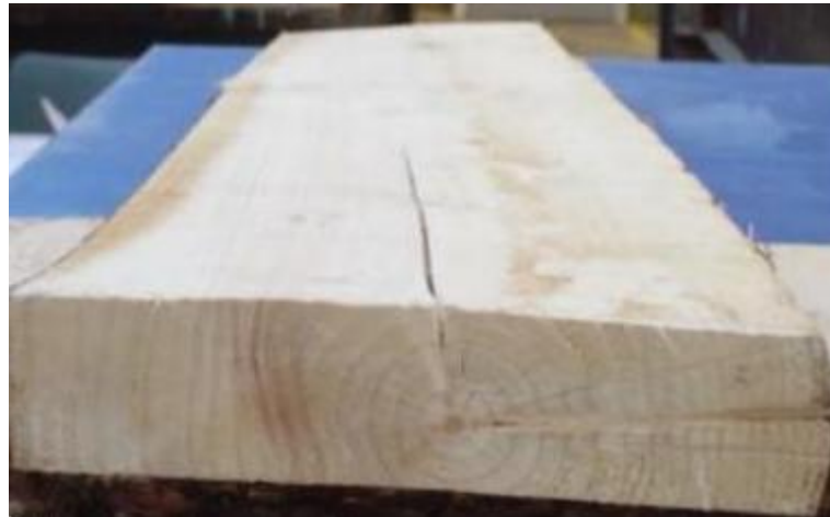
Figure 5.10: Twist of large section timber.
