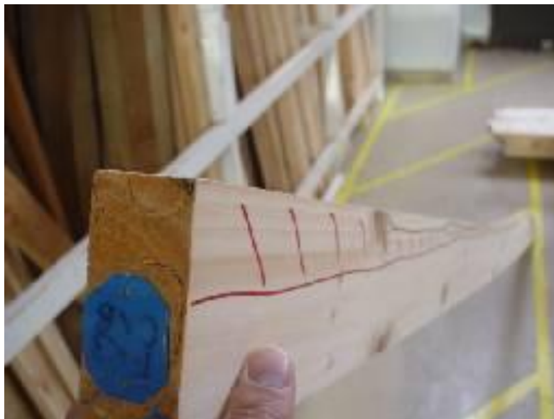
Figure 4.8: Batten FR3 ONB with compression wood consistently along one edge, which developed pronounced spring on drying.
