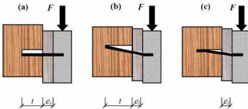
**Figure 7.13:** Failure modes of timber to thick steel connections with interlayer moving freely
