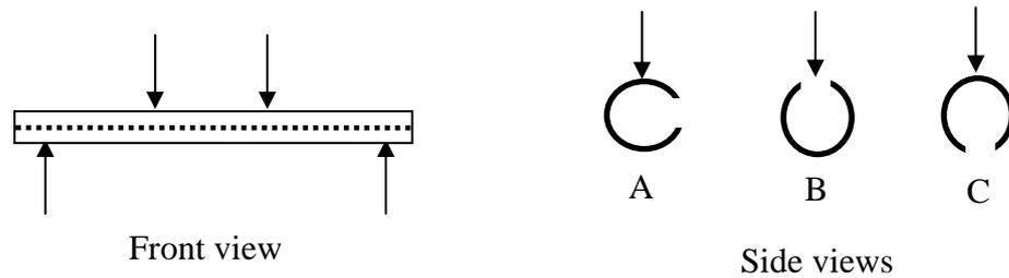
**Figure 7.6:** Yield moment tests, configuration for minimum yield moment of Express nails
