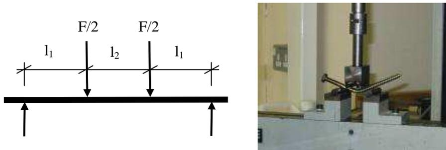
**Figure 3.3:** Four-point fastener bending test set up
