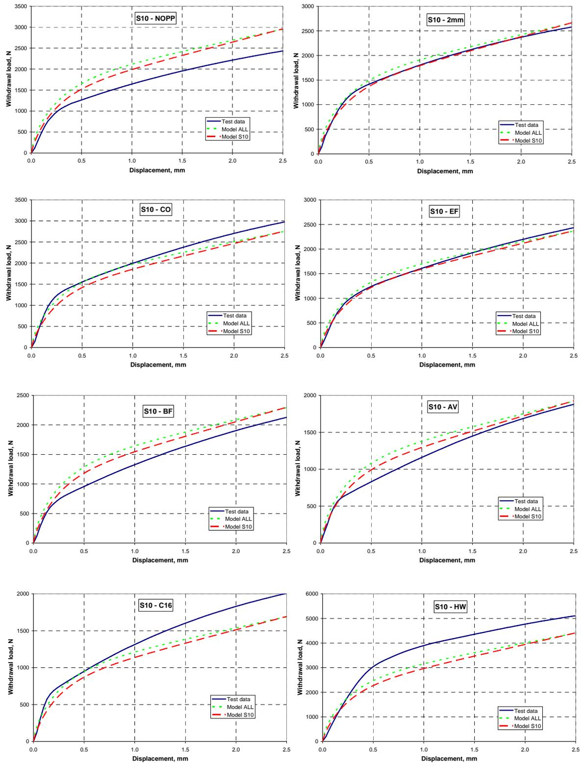
**Figure 4.16:** Withdrawal load displacement relationship from test and predicted from semi empirical models for StarTie 10 fasteners.
