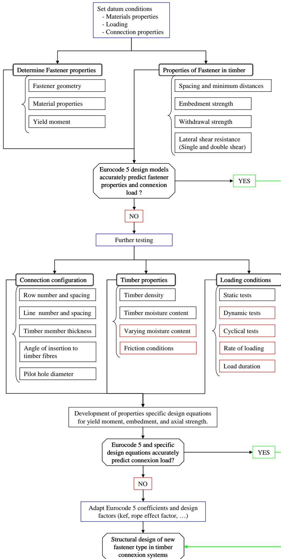
**Figure 1.4:** Schematic diagram of the experimental investigation
