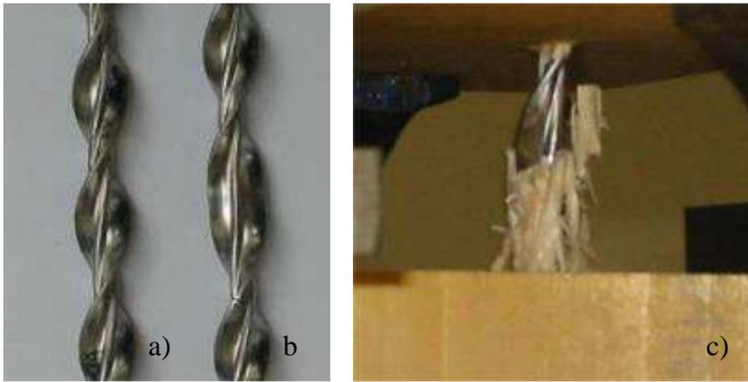
**Figure 4.6:** a) Helically shaped fastener; b) failure perpendicular to the timber grain; c) failure parallel to the timber grain.
