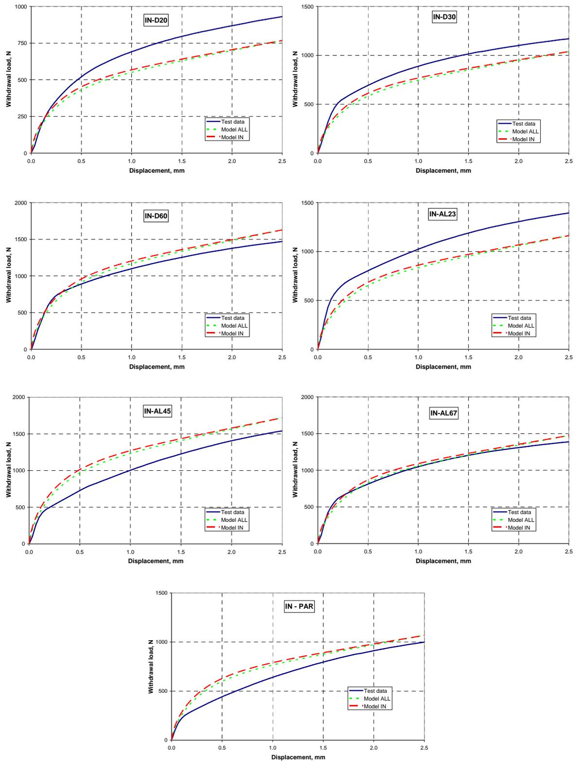
**Figure 4.18 continued:** Withdrawal load displacement relationship from test and predicted from semi empirical models for InSkew fasteners.
