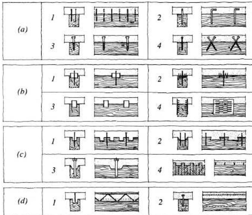
**Figure 7.1:** Examples of different timber-concrete connections systems: a) dowel type connectors; b) surface connections; c) notched connections; d) bonded connections (STEP 2, 1995)
