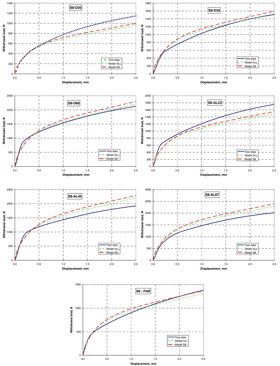
**Figure 4.17 continued:** Withdrawal load displacement relationship from test and predicted from semi empirical models for StarTie 8 fasteners.
