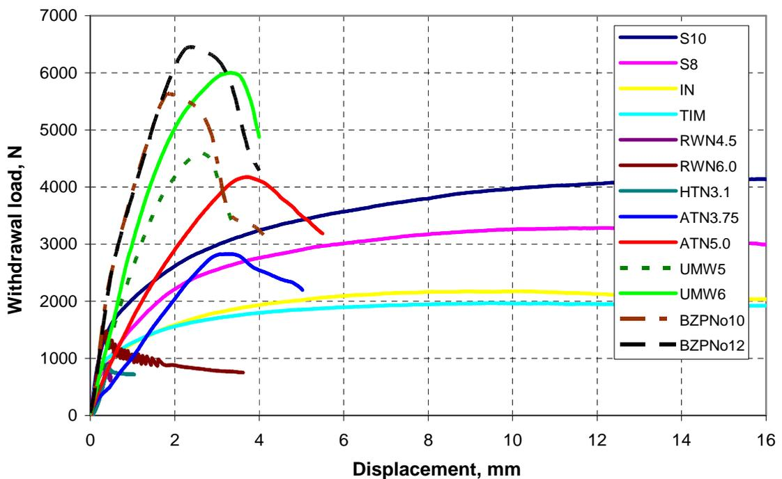
**Figure 4.4:** Typical withdrawal behaviour of timber fasteners.
