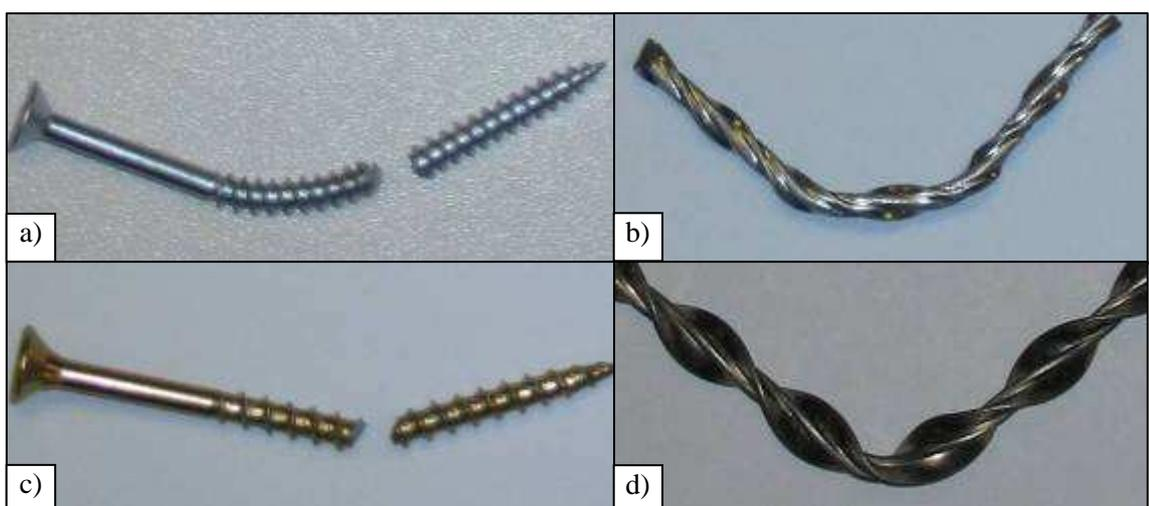
**Figure 3.9:** Bending tests a) four-point brittle failure; b) four-points ductile failure; c) three-point brittle failure and d) three-point ductile failure.
