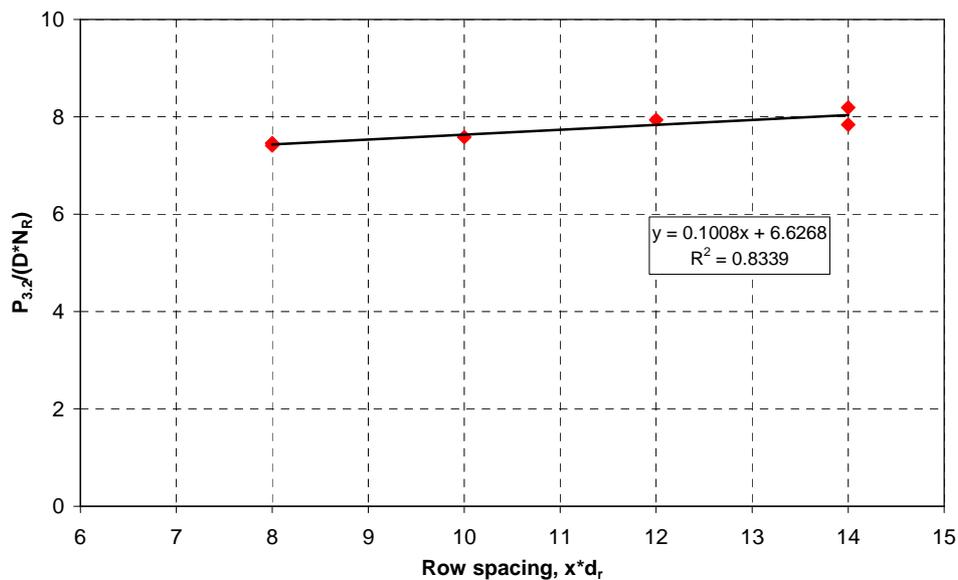
**Figure 5.20:** Effect of row spacing on joint strength
