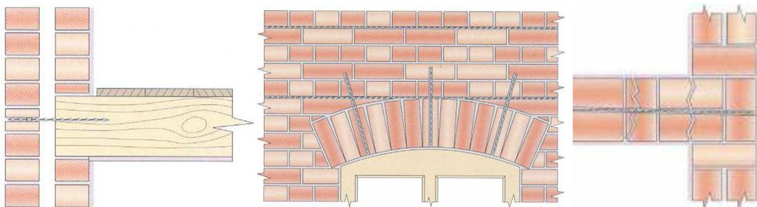
**Figure 1.1:** Examples of current uses of helically shaped fasteners.
