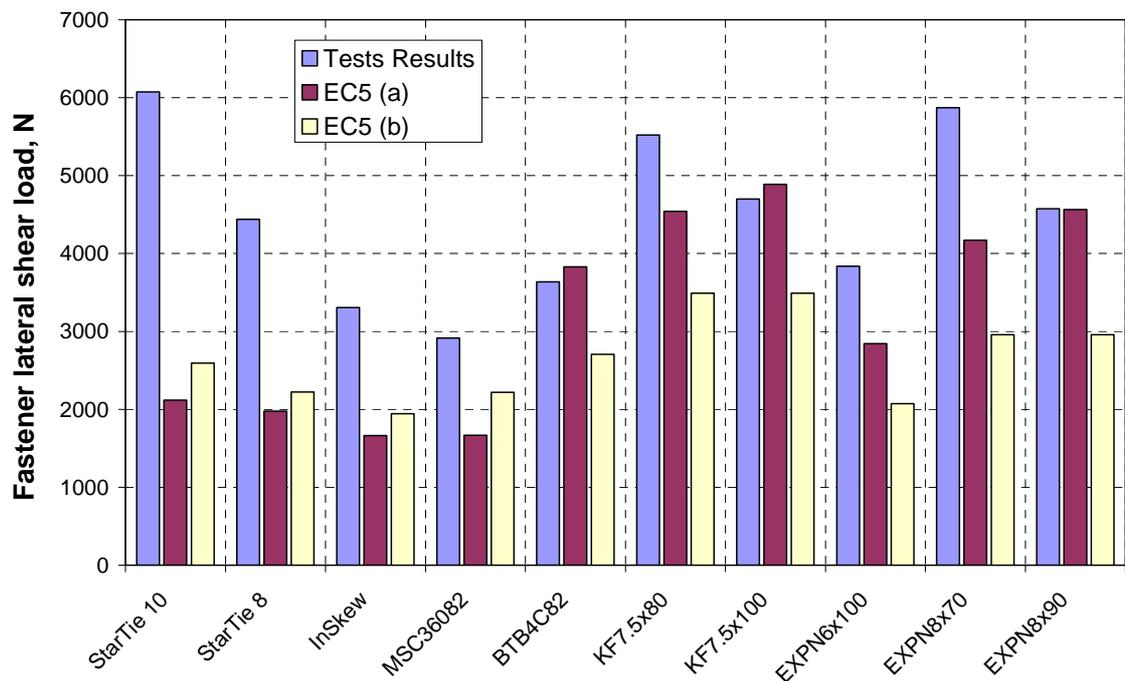
**Figure 7.7:** Timber-concrete characteristic lateral shear fixing capacity in 7N/mm<sup>2</sup> blocks
