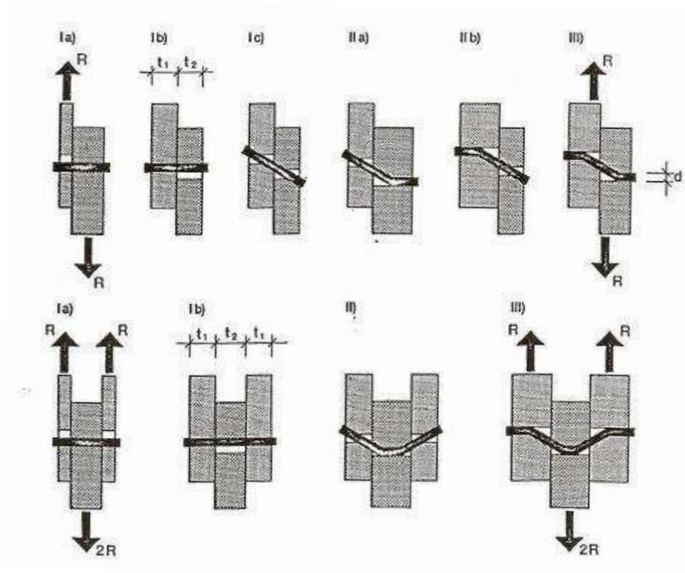
**Figure 2.10:** Modes of failure for single and double shear connections (Ehlbeck & Larsen, 1993)
