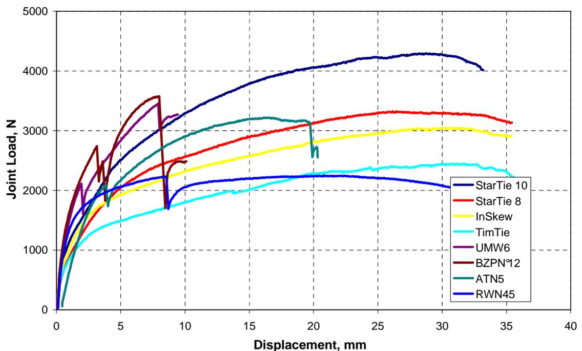
**Figure 7.12:** Typical load displacement curves of timber to concrete shear connections
