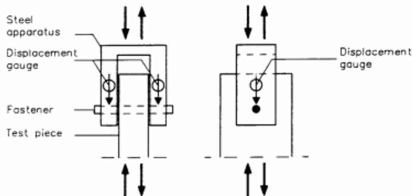
**Figure 2.6:** European embedment test setup (BSI, 2007).
