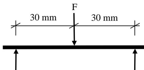
**Figure 3.5:** Three points fastener bending test set up.
