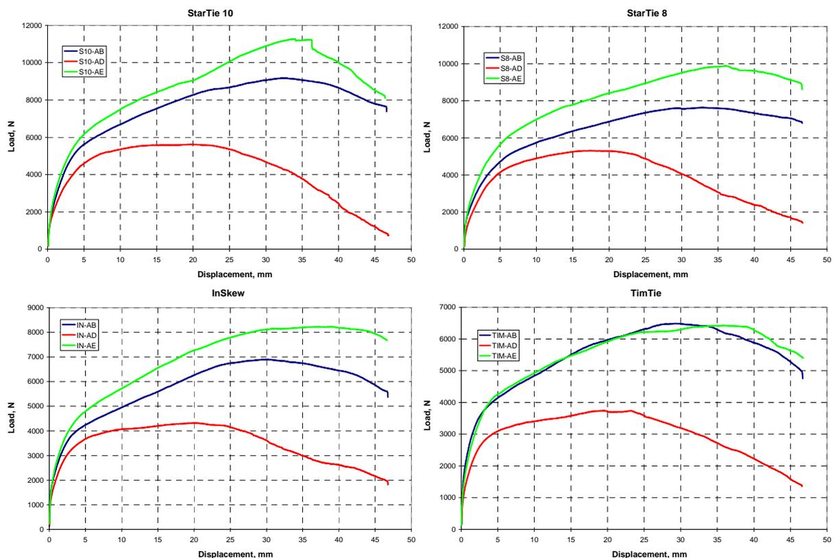
**Figure 5.9:** Effect of fastener overlap on joint behaviour
