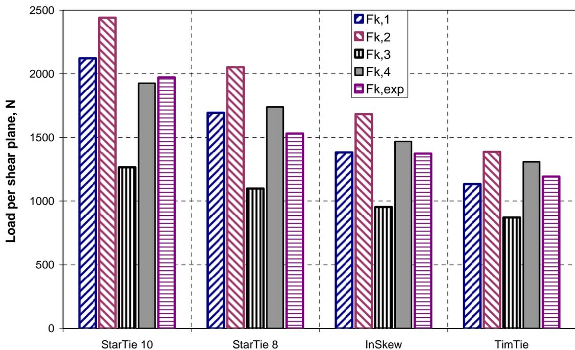
**Figure 6.2:** Characteristic load carrying capacities from Johansen, Eurocode 5 and tests
