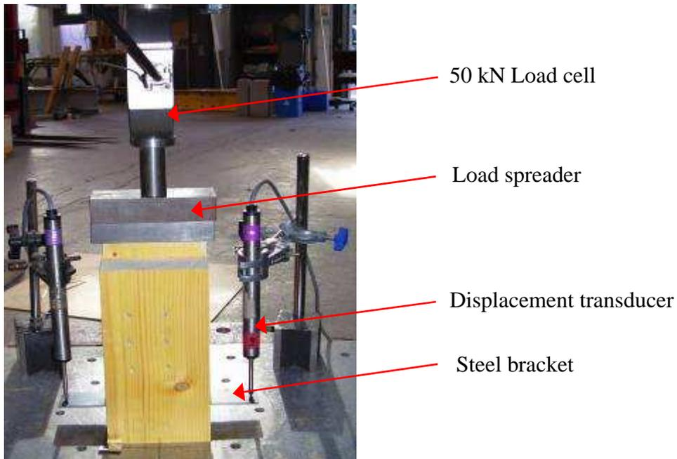
**Figure 5.3:** Lateral shear tests set up
