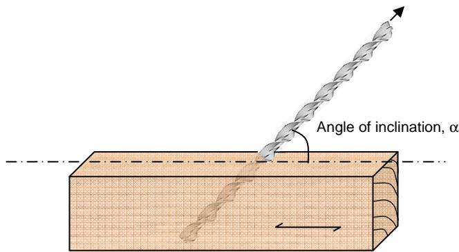
**Figure 4.8:** Fastener angle of penetration to the timber grain
