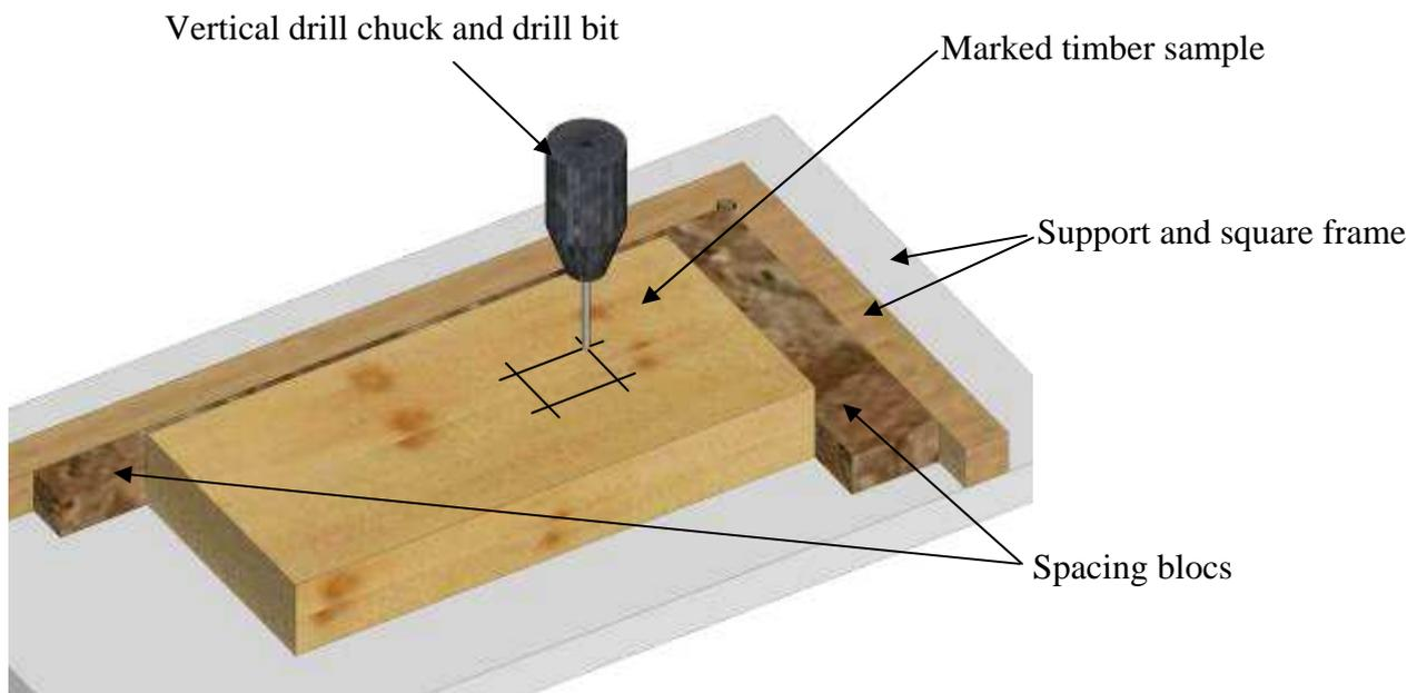
**Figure 5.1:** Drill set up of timber samples.
