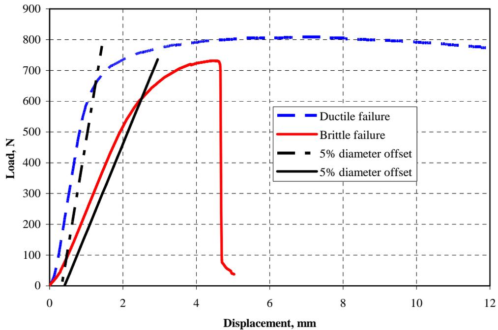
**Figure 3.8:** Typical three points bending test ductile and brittle failures
