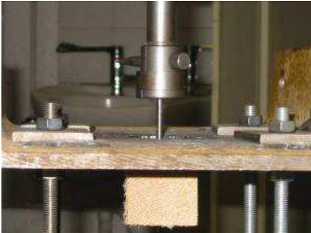
**Figure 4.1** Withdrawal test set up for common timber fasteners.
