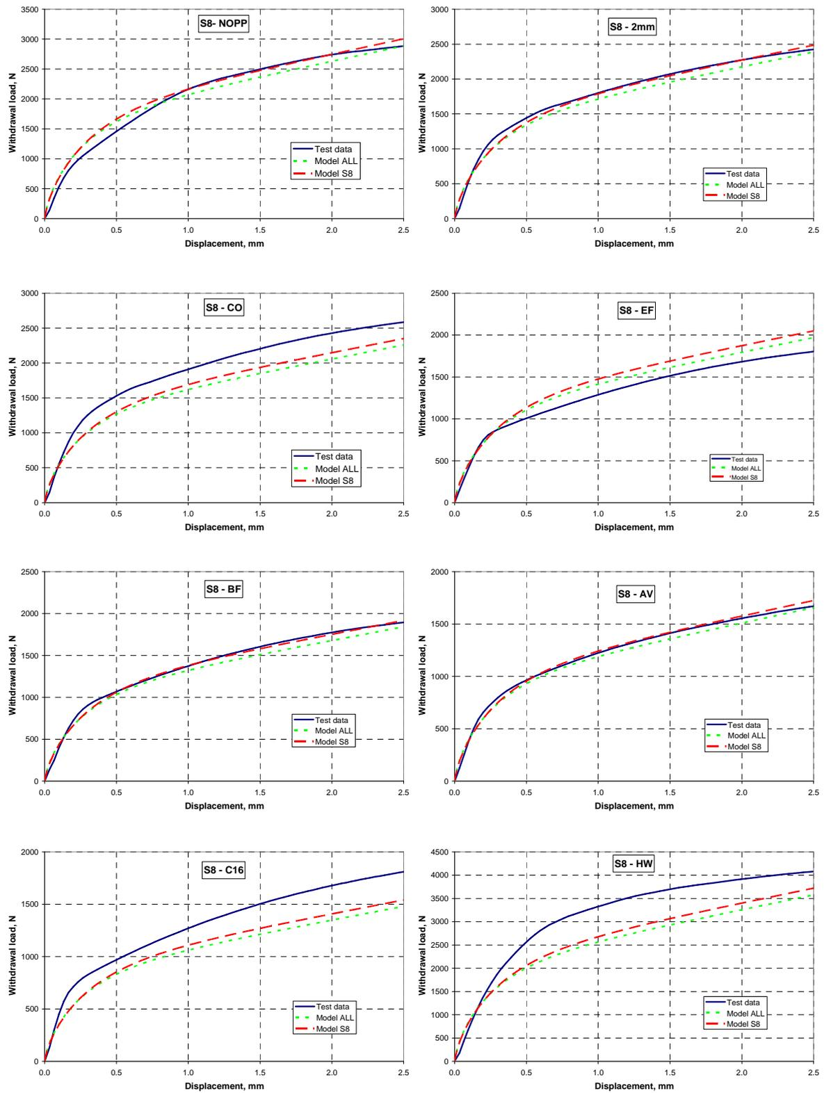
**Figure 4.17:** Withdrawal load displacement relationship from test and predicted from semi empirical models for StarTie 8 fasteners.
