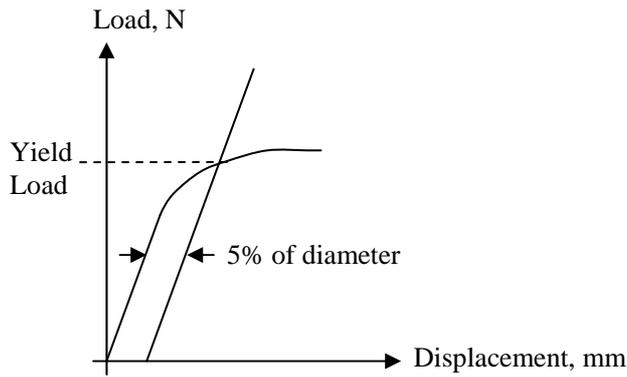
**Figure 3.6:** Typical load displacement curve and 5% offset yield moment load.
