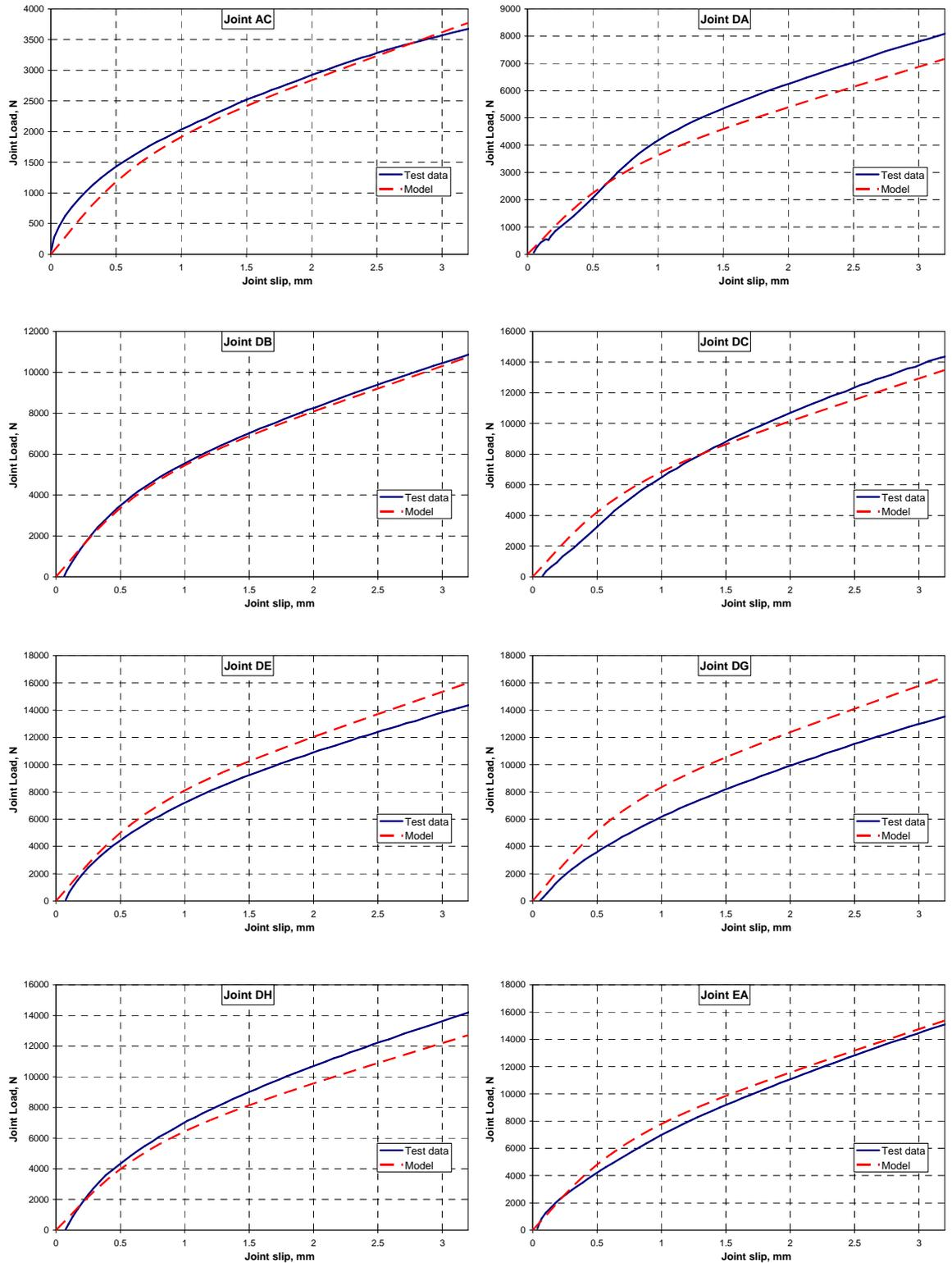
**Figure 5.22:** Comparison between load displacement behaviour of timber connections with helically shaped fasteners loaded in double shear and semi-empirical model
