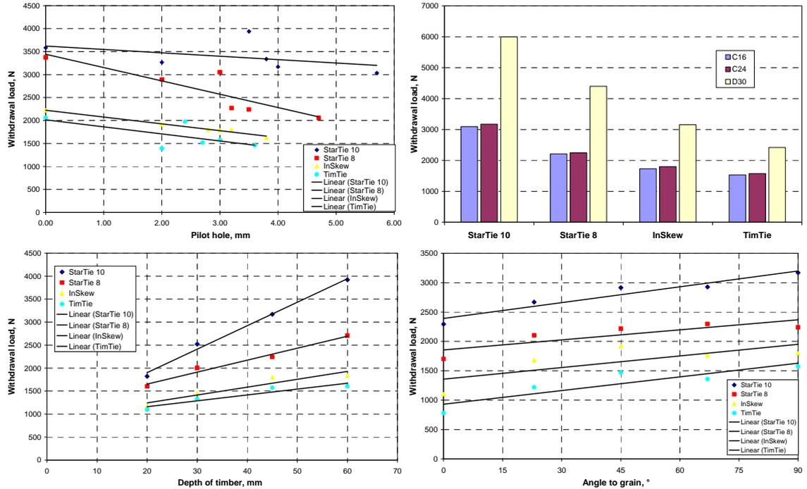
**Figure 4.9:** Effect of pilot hole, timber grade, depth of penetration and angle to grain, on the withdrawal load of helically shaped fasteners.
