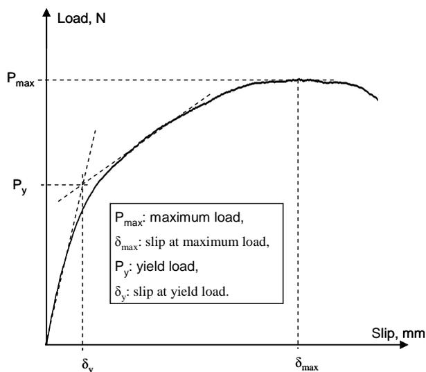
**Figure 5.6:** Test data load and displacement notation
