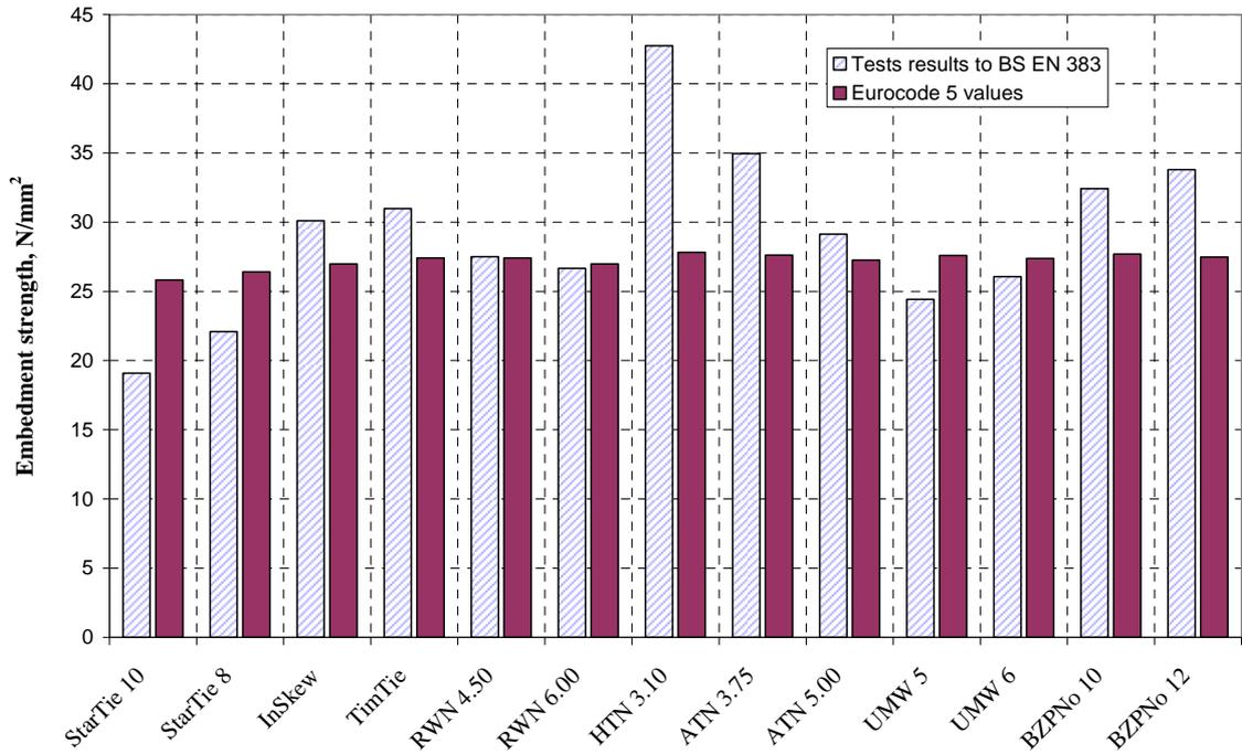
**Figure 3.15:** Embedment tests results to BS EN 383 and Eurocode 5 design values
