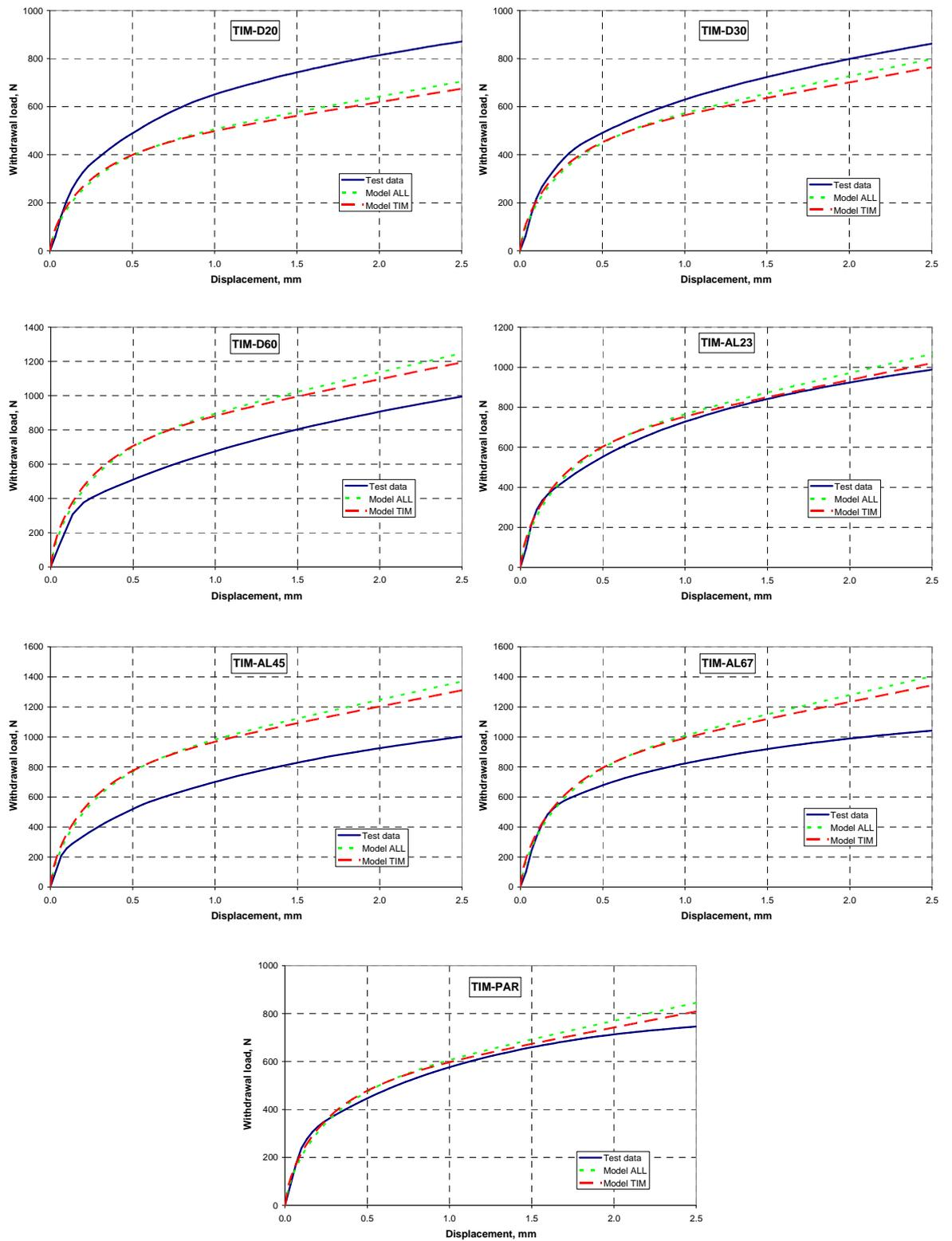
**Figure 4.19 continued:** Withdrawal load displacement relationship from test and predicted from semi empirical models for TimTie fasteners.
