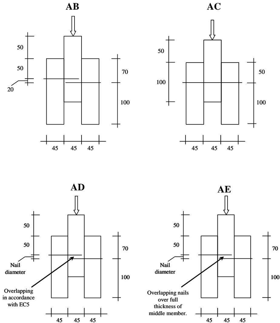
The nailing configurations above were tested with the four sizes of Helically shaped fasteners – i.e. StarTie 10, StarTie 8, InSkew and TimTie. The nailing configuration AB was used for tests with common timber fasteners such as woodscrews, smooth round and threaded nails.
