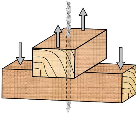
**Figure 4.3:** Withdrawal test specimen with helically shaped fastener
