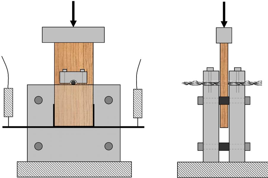
**Figure 3.12:** Embedment test set up.
