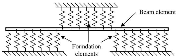
**Figure 2.11:** Elastic theory representation of a double shear connection.
