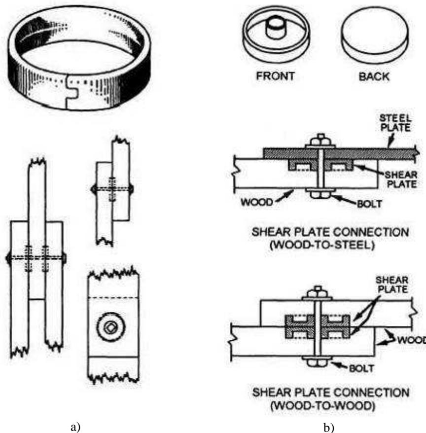
**Figure 2.3:** Bearing connectors: a) Split ring and connections, b) Shear plate and connections. (from [www.tpub.com](http://www.tpub.com))
