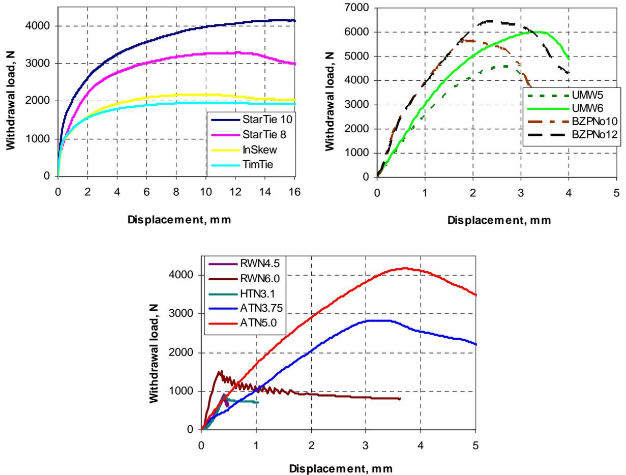
**Figure 4.5:** Withdrawal behaviour of a) Helically shaped fasteners, b) Woodscrews, and c) Nails.
