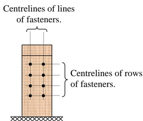
**Figure 5.12 :** Centrelines of rows and lines of fasteners in a connection
