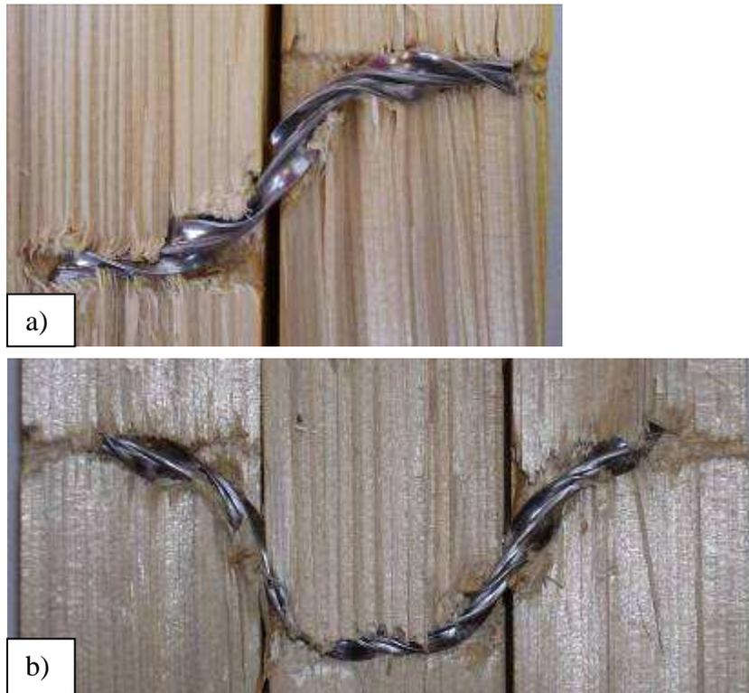
**Figure 6.3:** Typical failure modes of joints with helically shaped fasteners loaded in single (a) and double (b) shear
