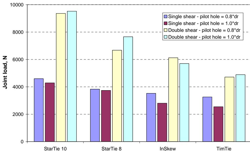
**Figure 5.10:** Effect of pilot hole on joint load
