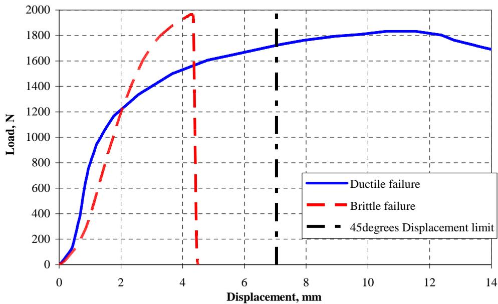
**Figure 3.7:** Typical four points bending test ductile and brittle failures, and 45° limit for 51mm span test set up.
