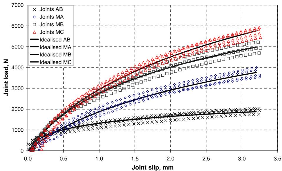
**Figure 5.18:** Joints AB, MA, MB MC test data, and idealised curves
