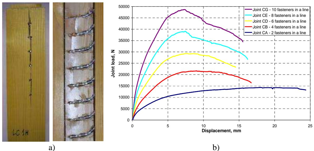
**Figure 5.15:** a) Brittle failure due to wood splitting; b) Ductile behaviour
