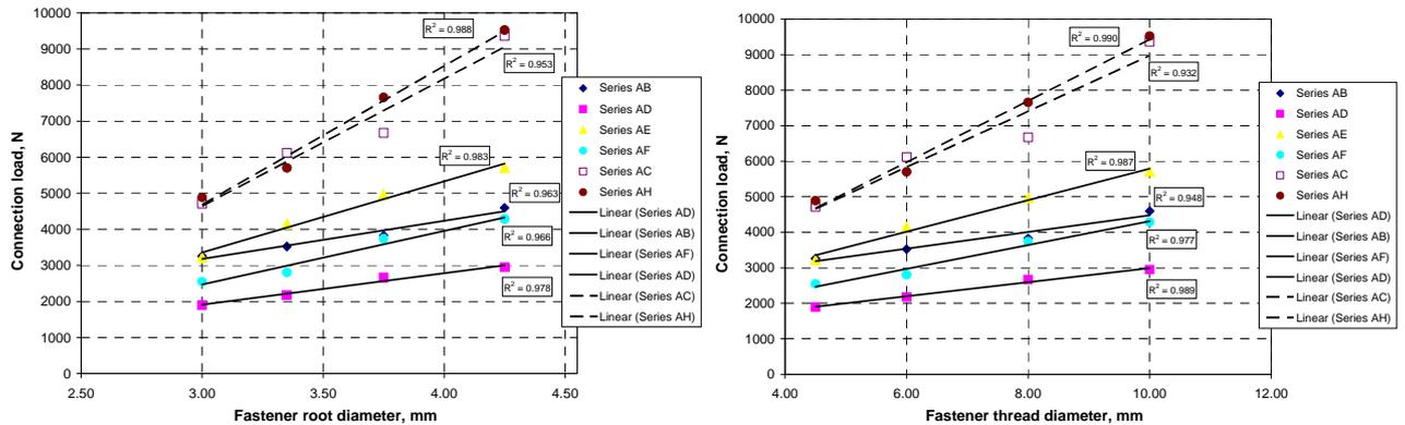
**Figure 5.11:** Load connection vs. fastener root and thread diameter
