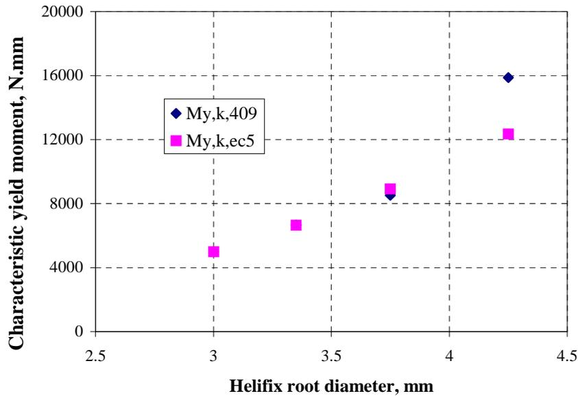
**Figure 3.11:** Relationship between Helically shaped root diameter and characteristic yield moments.
