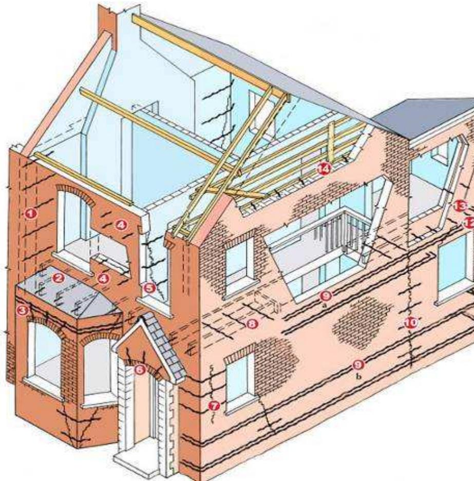
**Figure 1.3:** Typical masonry damages and repair techniques (from [www.Helicalllyshaped.co.uk](http://www.Helicalllyshaped.co.uk))
