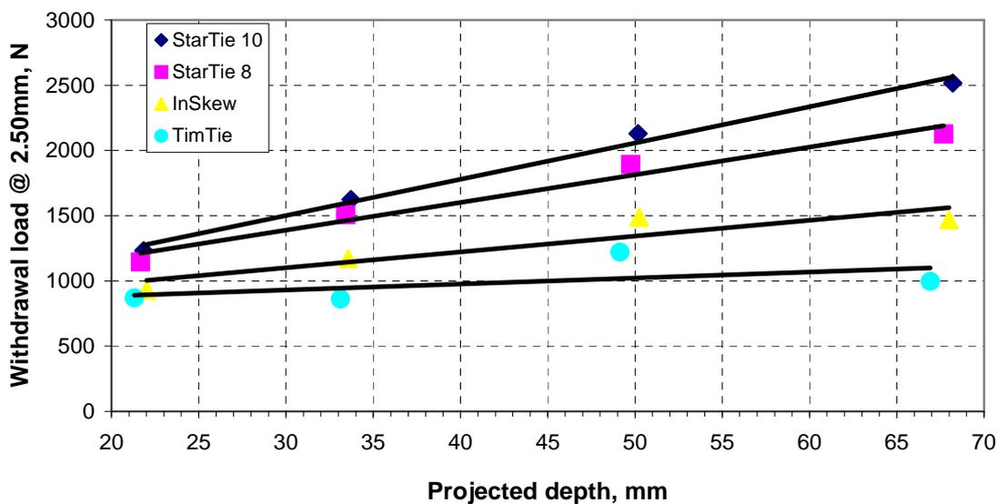
**Figure 4.12:** Withdrawal load vs projected depth of penetration
