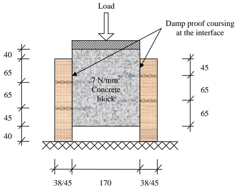
**Figure 7.4:** Typical sole plate connection test set up
