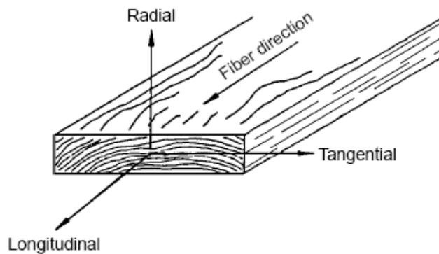
**Figure 2.5:** The three principal axes of wood (Forest Product Laboratory, 1999)
