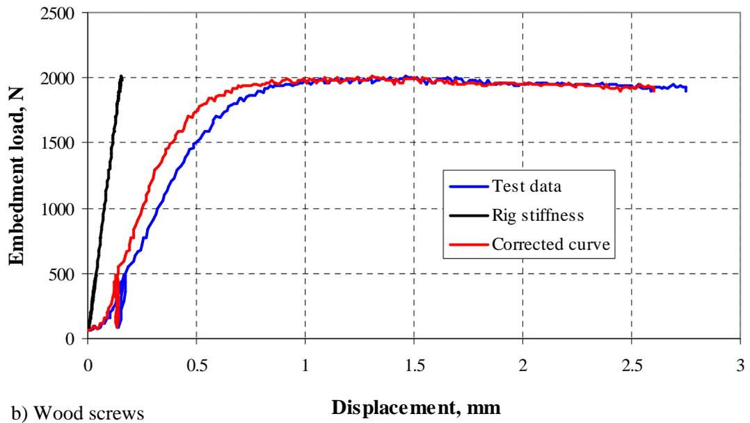
**Figure 3.14:** Typical load displacement curves from embedment test results and corrected curves for a) Helically shaped fasteners, and b) Woodscrews.
