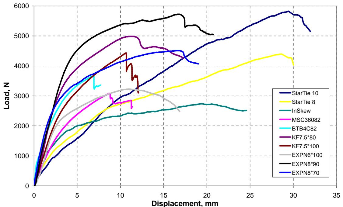
**Figure 7.8:** Fasteners typical load displacement curves in Timber-concrete connections
