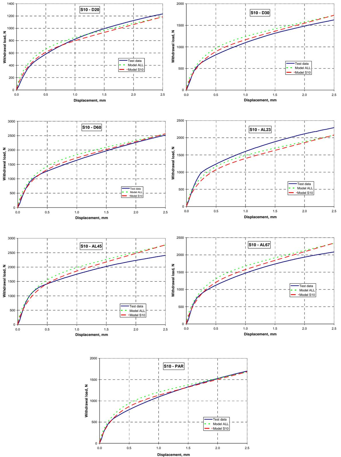
**Figure 4.16 continued:** Withdrawal load displacement relationship from test and predicted from semi empirical models for StarTie 10 fasteners.
