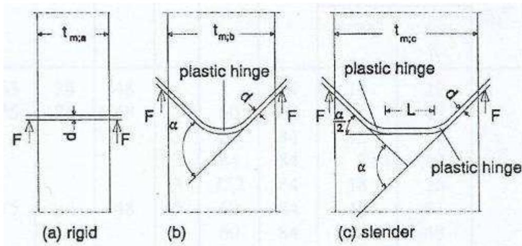
**Figure 3.4:** Deformation of dowel type fasteners depending on fastener slenderness. (Jorissen & Blass, 1998)
