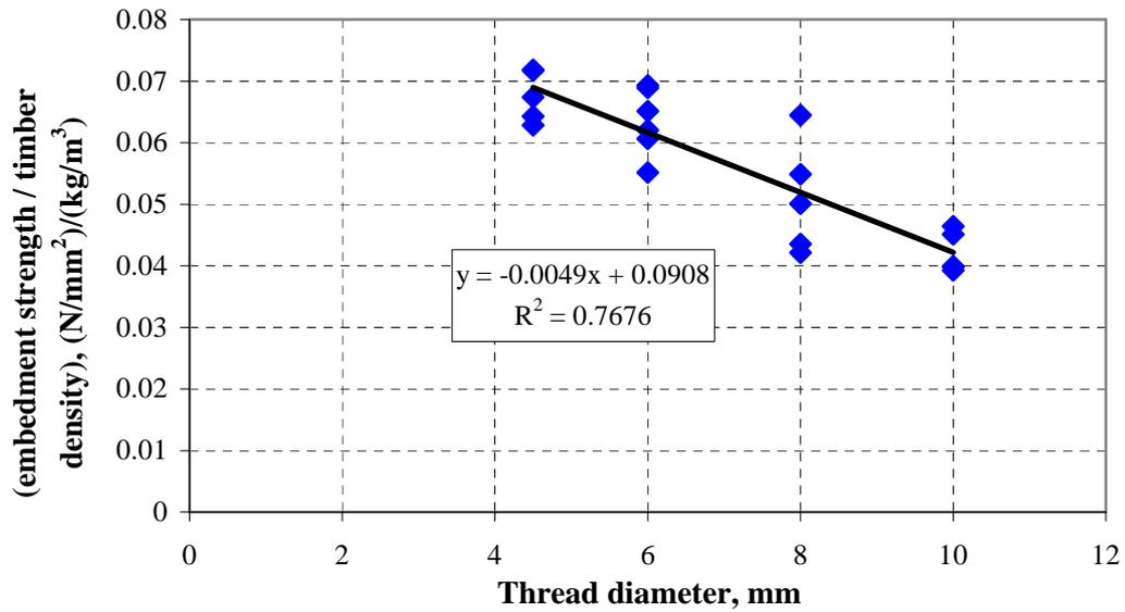
**Figure 3.17:** Influence of fastener diameter on helically shaped fasteners embedment strength
