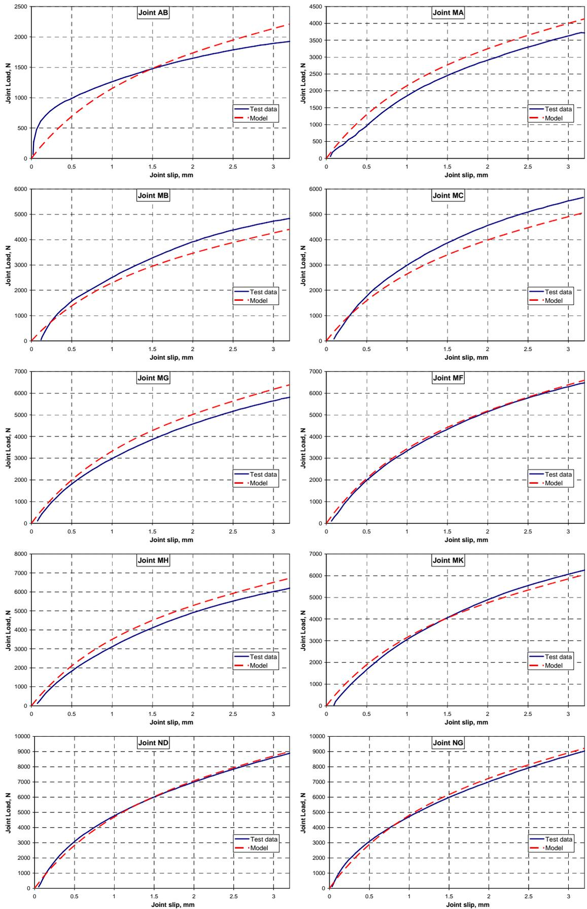
**Figure 5.21:** Comparison between load displacement behaviour of timber connections with helically shaped fasteners loaded in single shear and semi-empirical model
