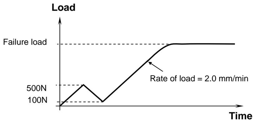
**Figure 5.2:** Loading procedure for laterally loaded joints
