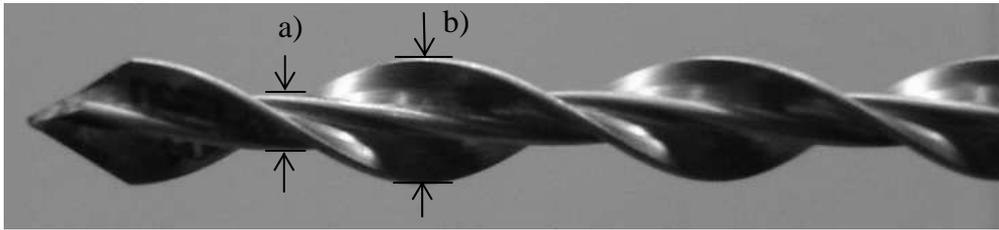
**Figure 1.2:** Helically shaped connector, a) root diameter, b) shank diameter.
