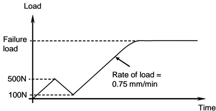
**Figure 3.13:** Rate of loading for embedment tests.
