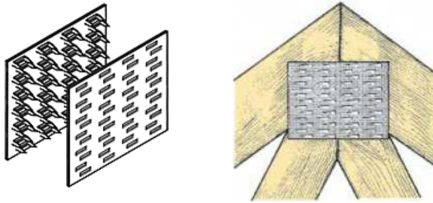
**Figure 2.2:** Punched nail plate, Truss connection with nail plate (from [mii.com/unitedkingdom](http://mii.com/unitedkingdom)).
