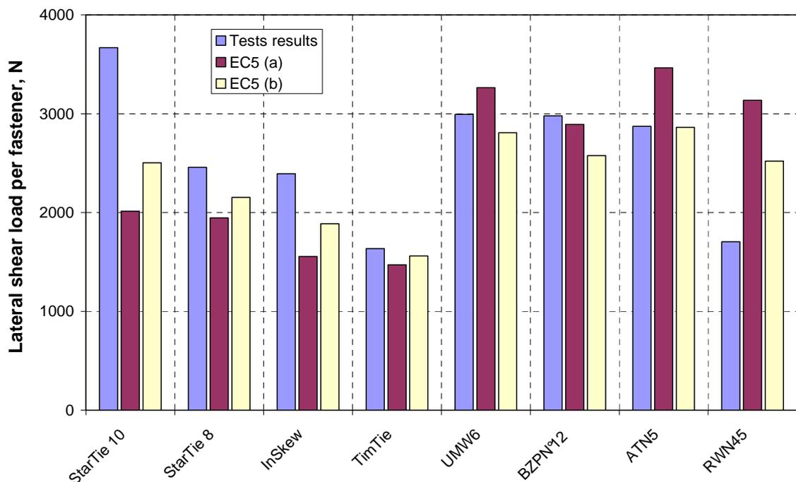
**Figure 7.11:** Fixings characteristic shear capacity in timber to concrete connections
