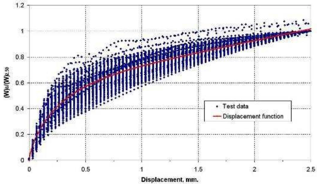
**Figure 4.10:** Regression graph for all helically shaped fasteners and corresponding displacement function  $f_1(\delta)$ .
