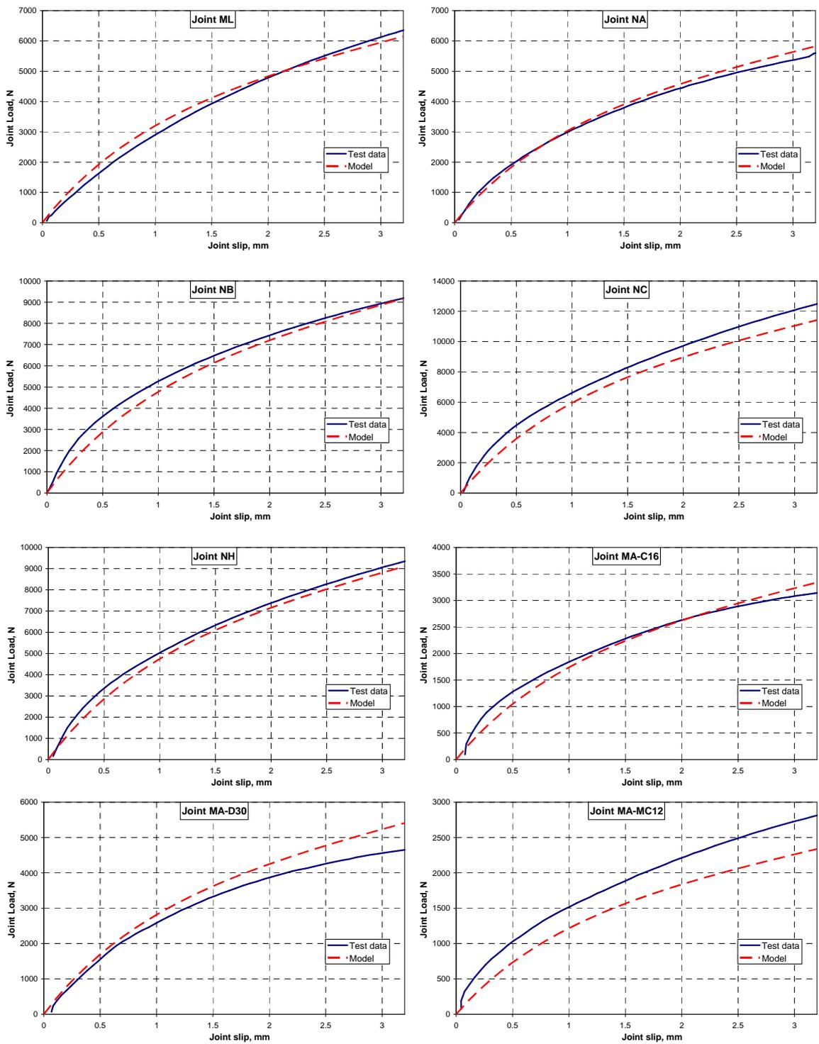
**Figure 5.21 (Continued):** Comparison between load displacement behaviour of timber connections with helically shaped fasteners loaded in single shear and semi-empirical model
