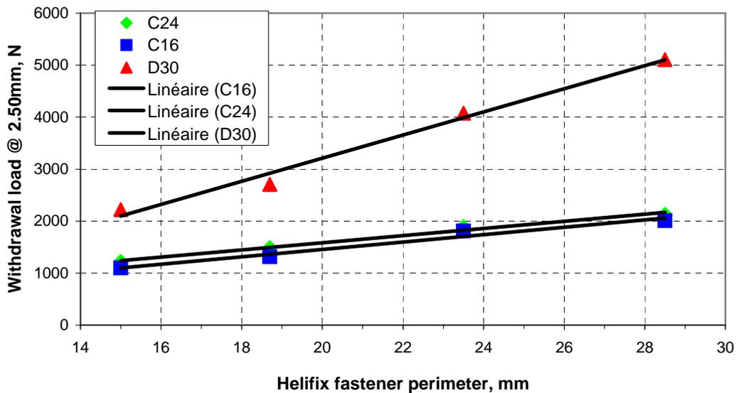
**Figure 4.11:** Relationship between withdrawal load and fastener perimeter.
