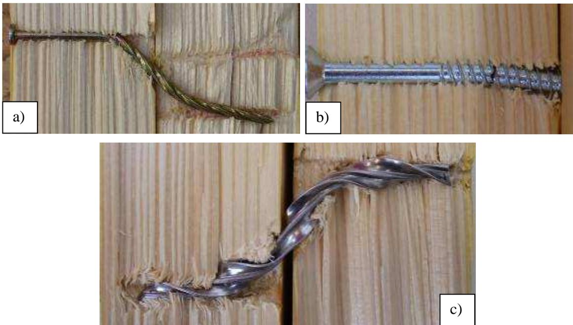
**Figure 5.8:** Typical failures for a) threaded nails; b) wood screw, c) Helically shaped fasteners
