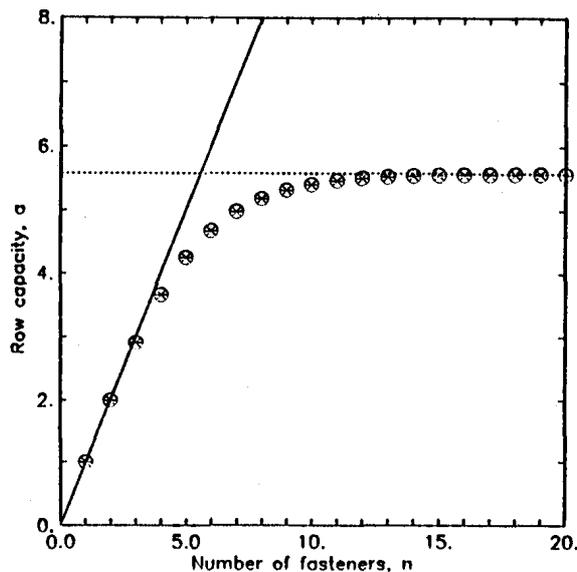
**Figure 5.13:** Effective number of fasteners in a line (Zahn, 1991)
