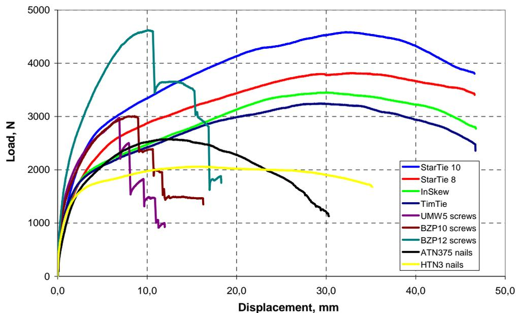
**Figure 5.7:** Typical load displacement relationships of single fastener tests
