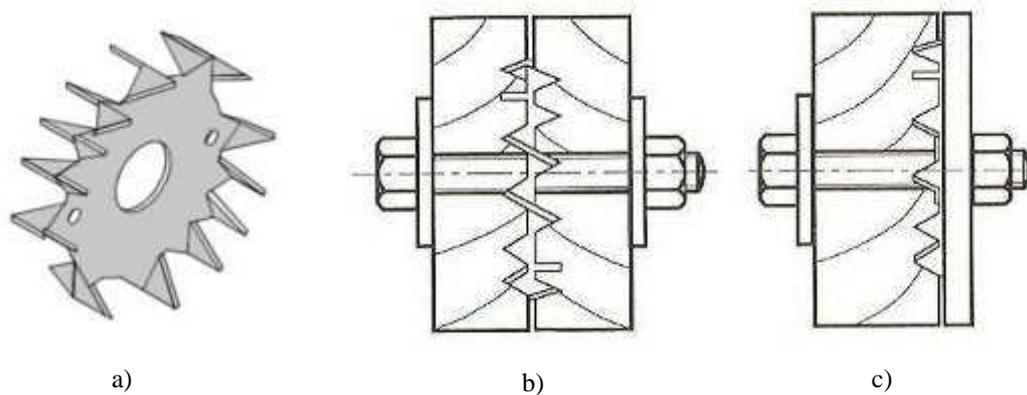
**Figure 2.4:** a) double sided toothed plate, b) timber to timber joint with double sided toothed plate, c) timber to steel joint with single sided toothed plate (STEP 1, 1995).
