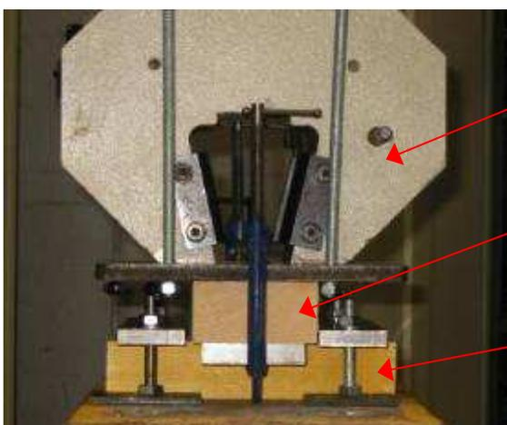
Travelling head of the testing machine, providing the tensile force for the tests
