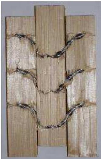
**Figure 5.14:** Mode of failure of multiple fastener samples
