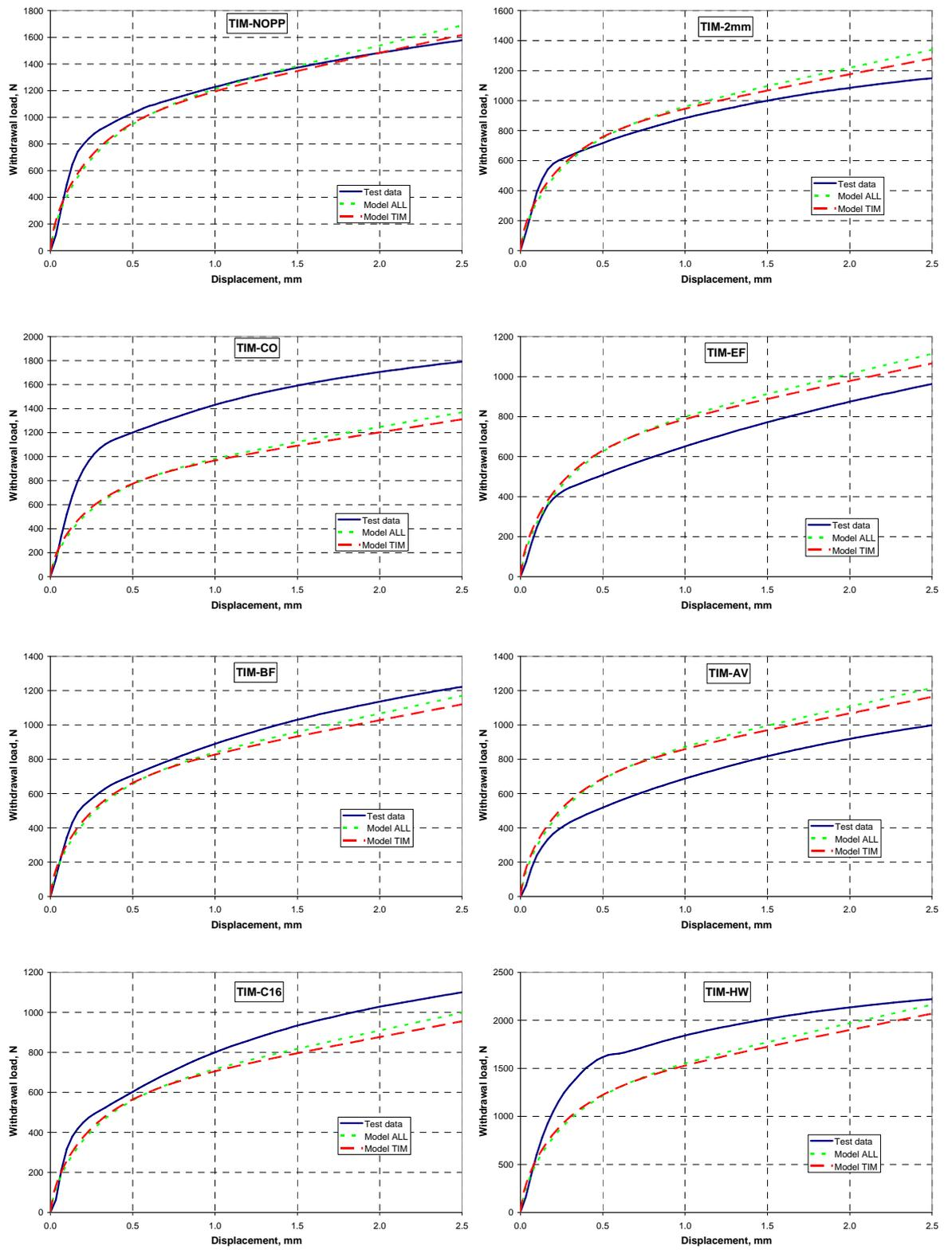
**Figure 4.19:** Withdrawal load displacement relationship from test and predicted from semi empirical models for TimTie fasteners.
