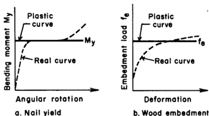
**Figure 2.9:** Idealisation of nail and wood properties (Aune & Patton-Mallory, 1986(a))
