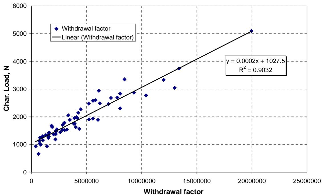
**Figure 6.1:** Relationship between withdrawal factor and characteristic load
