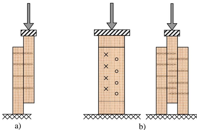
**Figure 5.4:** a) Single shear test; b) “Double single shear” set up used in the experimental programme.
