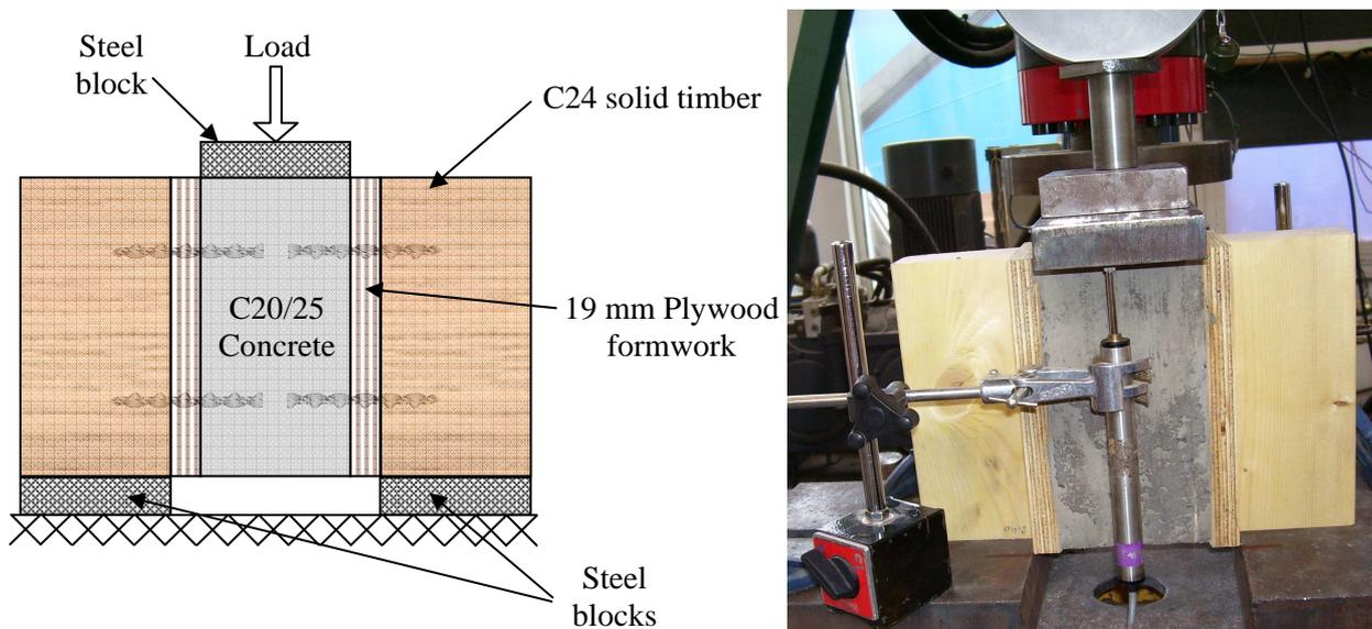
**Figure 7.10:** Typical timber to cast concrete shear test arrangement
