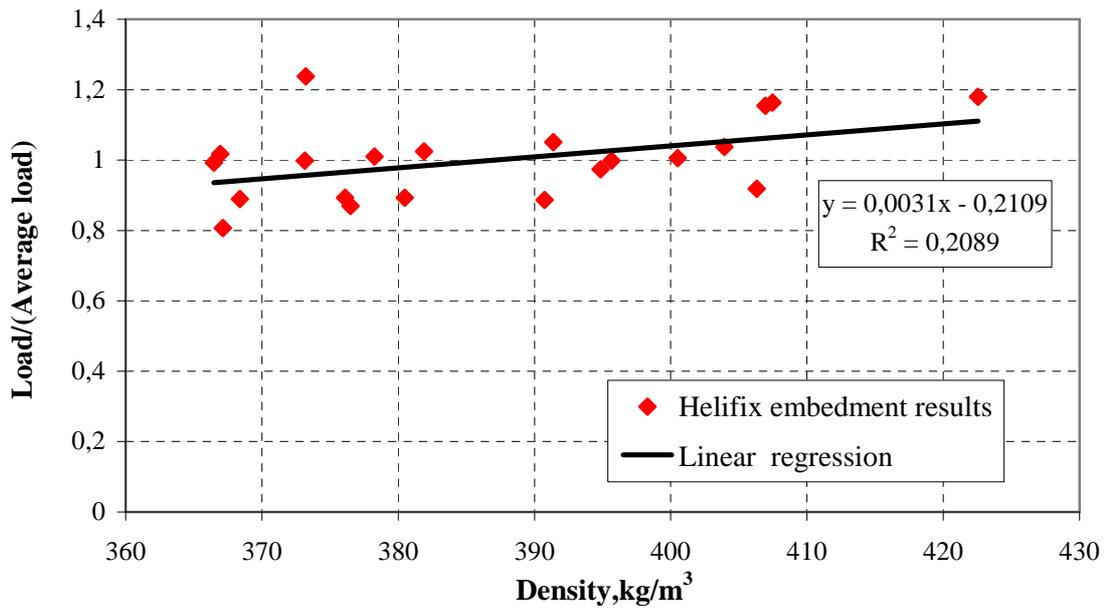
**Figure 3.16:** Influence of timber density on helically shaped fasteners embedment strength
