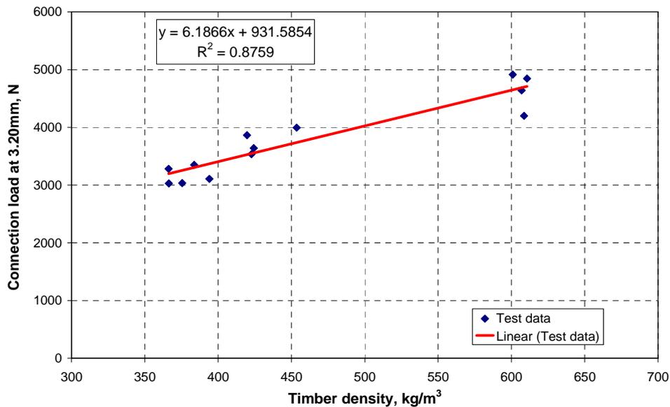
**Figure 5.17:** Connection load vs. timber density
