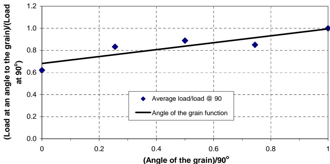
**Figure 4.15:** Angle to the grain function,  $f_6(\alpha)$
