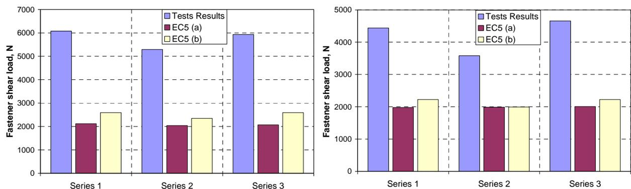
**Figure 7.9:** Results of Helically shaped fasteners test series 1, 2 and 3 for Helically shaped StarTie 10 (left) and StarTie 8 (right) fasteners
