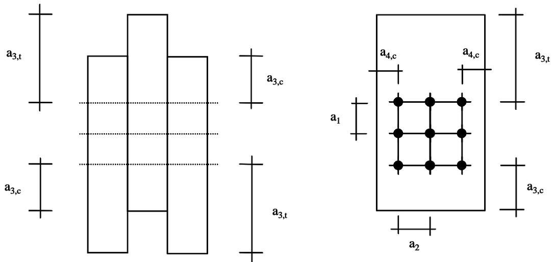
**Figure 5.5:** Spacings and end/edges distances according to EC5 (BSI, 2004)
