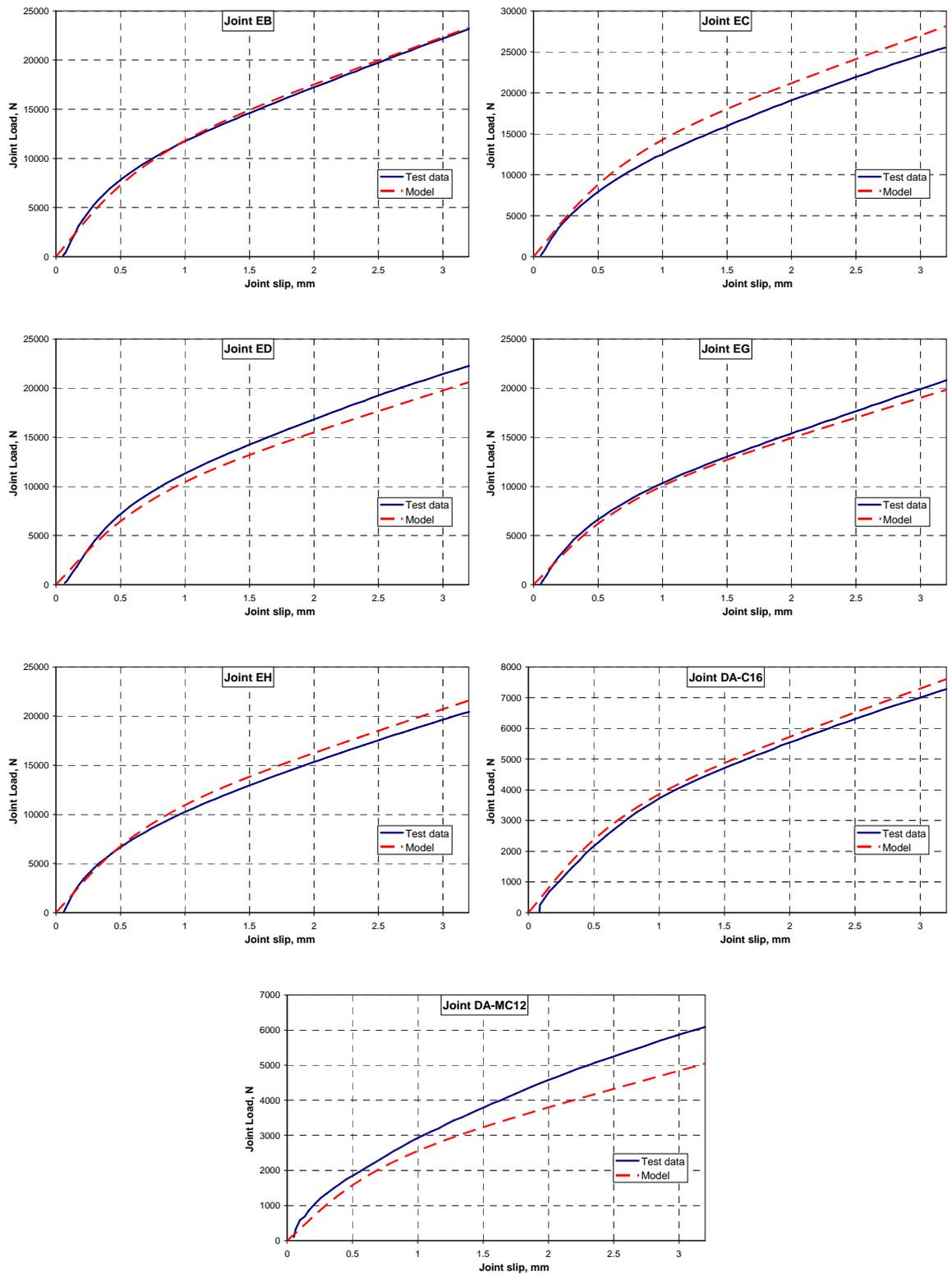
**Figure 5.22 (continued):** Comparison between load displacement behaviour of timber connections with helically shaped fasteners loaded in double shear and semi-empirical model
