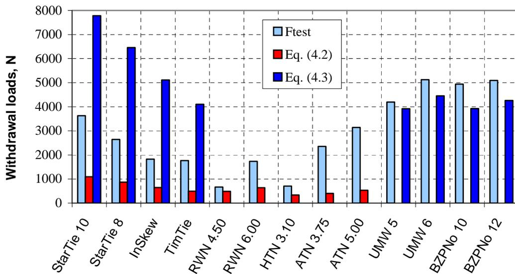
**Figure 4.7:** Characteristic withdrawal values from tests and EC5
