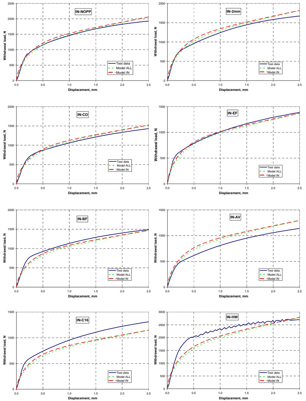
**Figure 4.18:** Withdrawal load displacement relationship from test and predicted from semi empirical models for InSkew fasteners.
