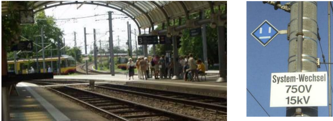
Figure 8-8 Ramp at Albtalbahnhof with interchange from 750 V DC to 15kV AC
