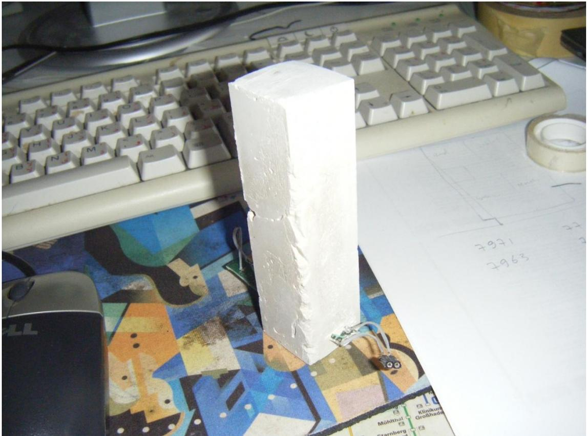
**Figure 5.17** Plaster column with two embedded TF sensors
