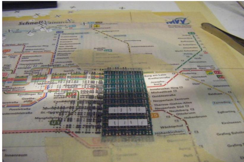
**Figure 4.10** Two arrays of four TF sensors mounted on PCB
