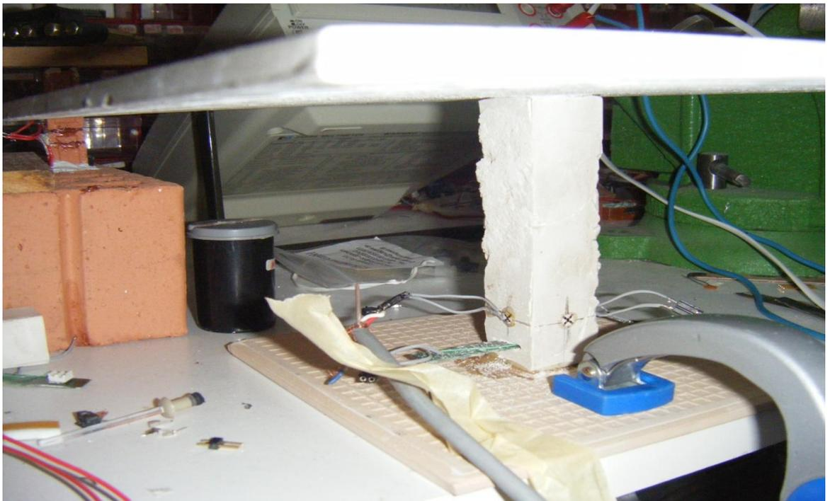
**Figure 6.13** TF sensors embedded and on surface of plaster column
