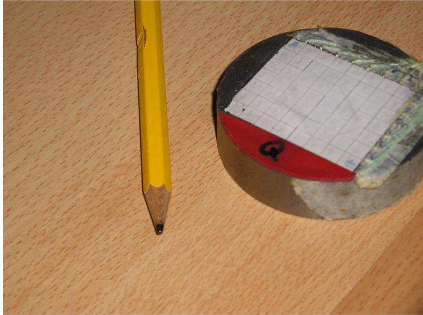
**Figure 5.7** An array of TF sensors mounted in SM technology
