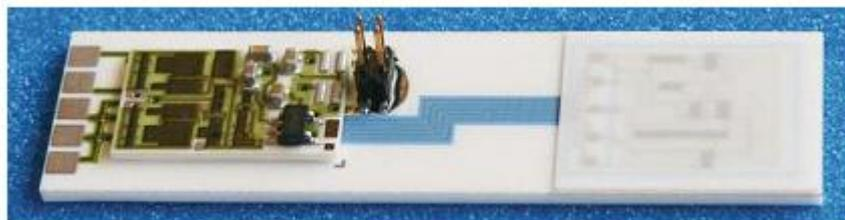
**Figure 6.2** Liquid level sensor
