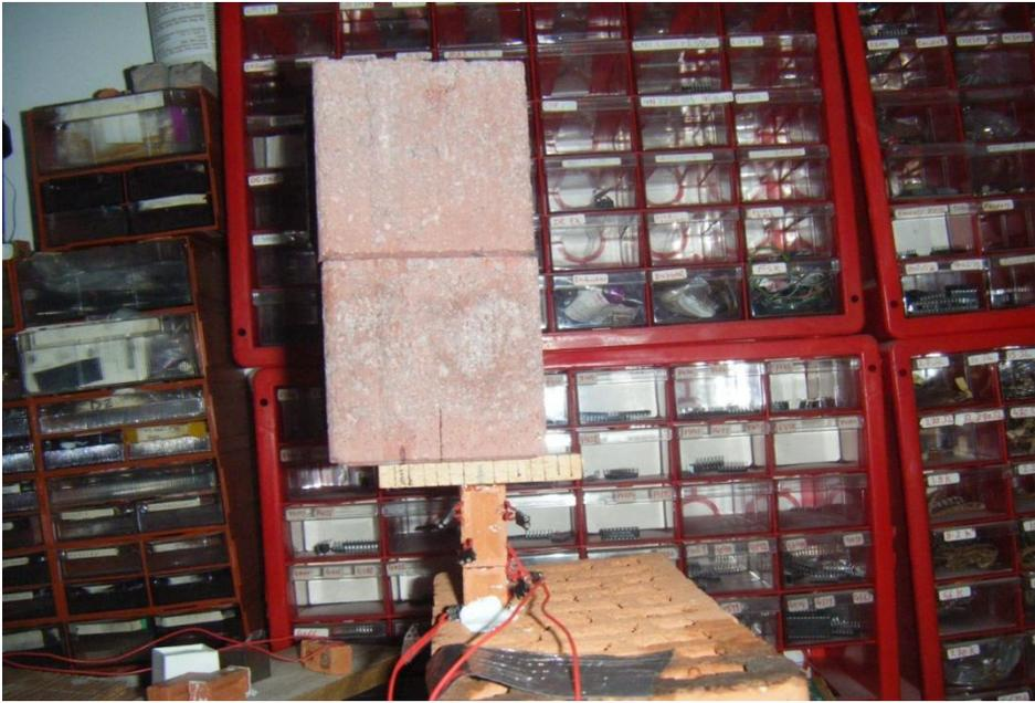
**Figure 6.7** TF sensors on sides of Brick column with moving load
