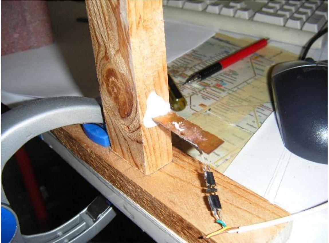
**Figure 5.13** Surface Mounted sensor embedded in wood
