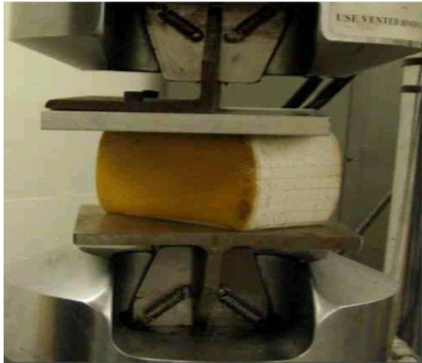
**Figure 7.2** Bulge occurs in the middle in relatively flexible material
