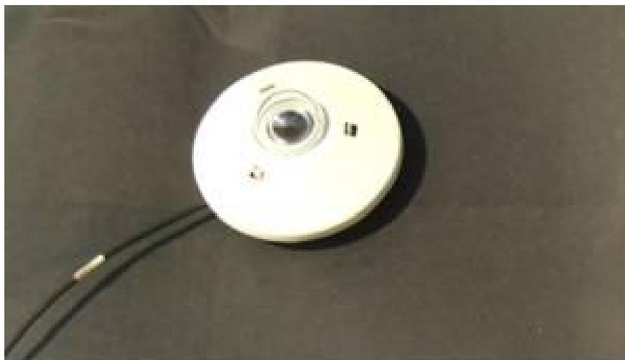
**Figure 4.6: Pyranometer instrument employed to measure the solar radiation.**
