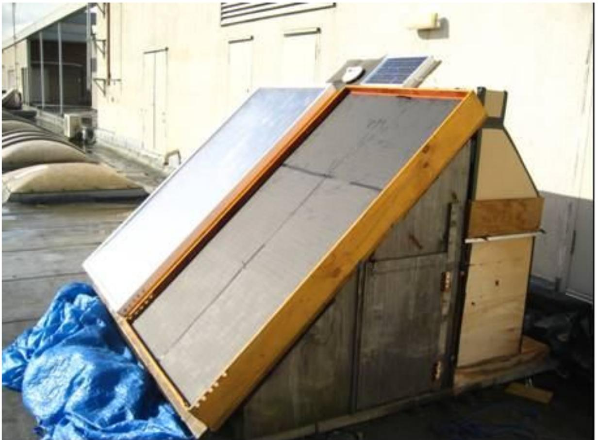
**Figure 4.4: Solar collector testing rig on the roof.**
