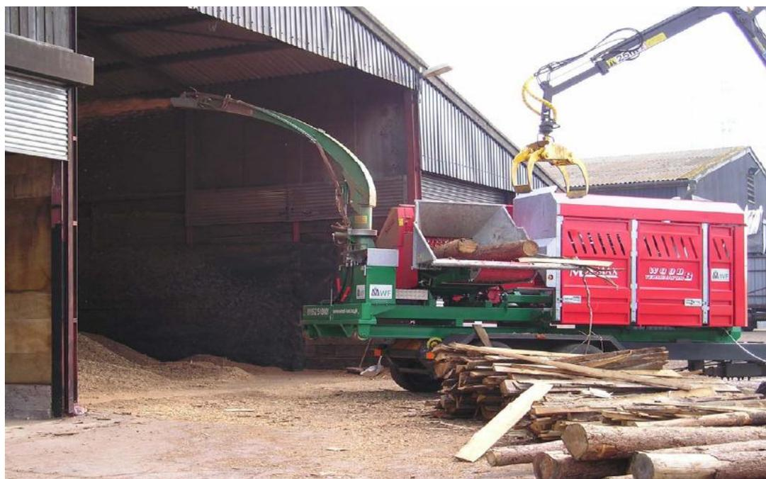
**Figure 1.3: Wood chipper machine in operation.**
