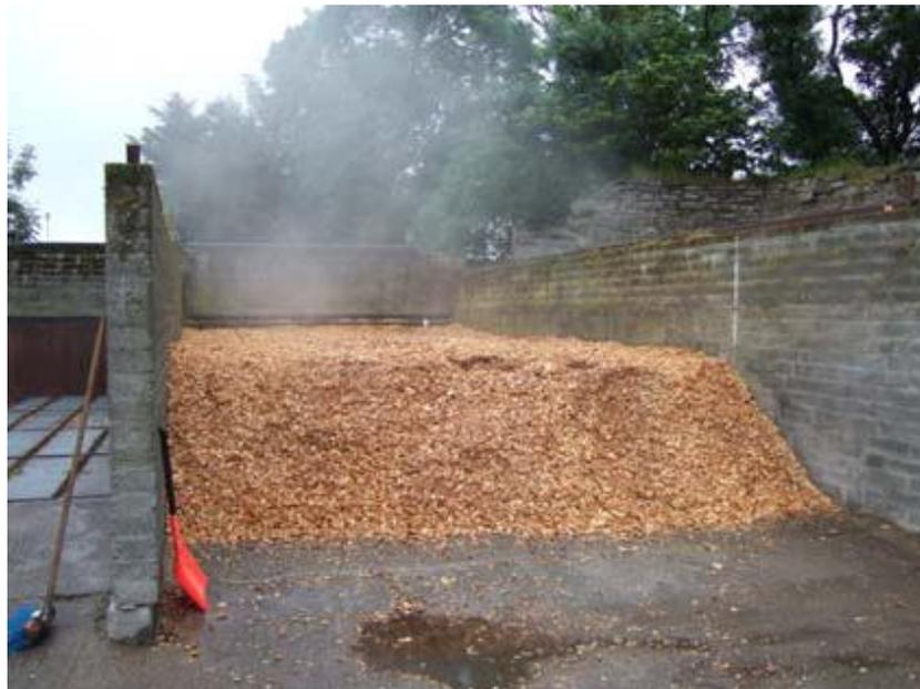
**Figure 2.9: Fresh woodchip being dried with forced air ventilation.**
