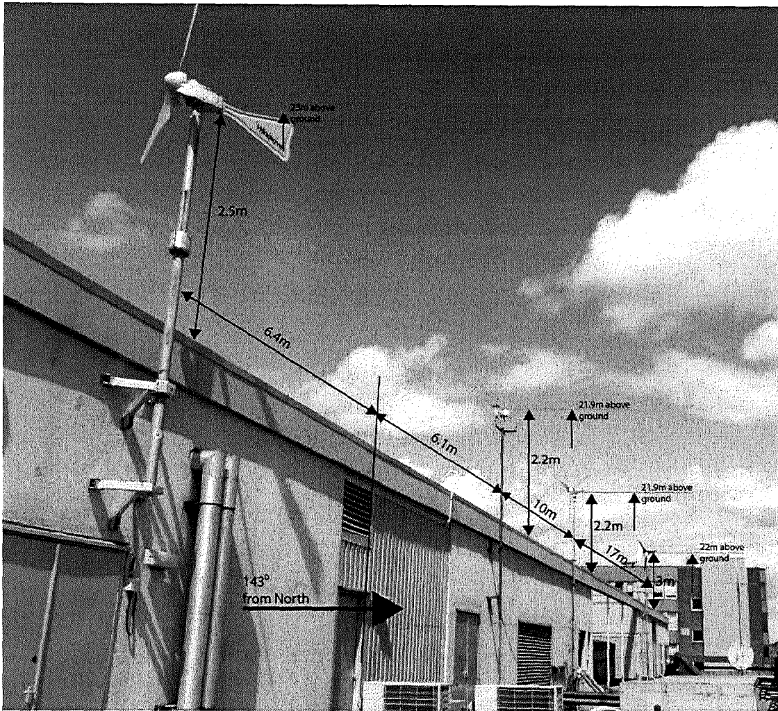
Figure 3.1 Edinburgh Napier University Merchiston Campus rooftop test site. (From the left, Windsave turbine, wind monitoring station, Air-Dolphin turbine, Ampair 600 turbine and anemometer).
