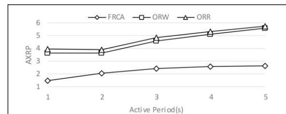
Fig. 14. Average Number of Redundant Packets varying active periods.
