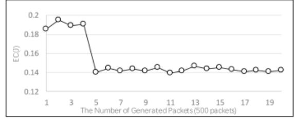
Fig. 17. The variations of the Energy consumption after changing network routing policy.
