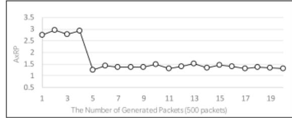
Fig. 18. The variations of the average number of redundant packets after changing network routing policy.
