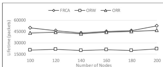
Fig. 12. Network lifetime varying number of nodes.
