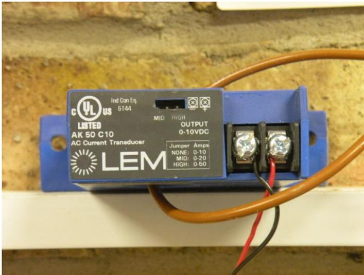
Figure 4-7: AC current sensor.
