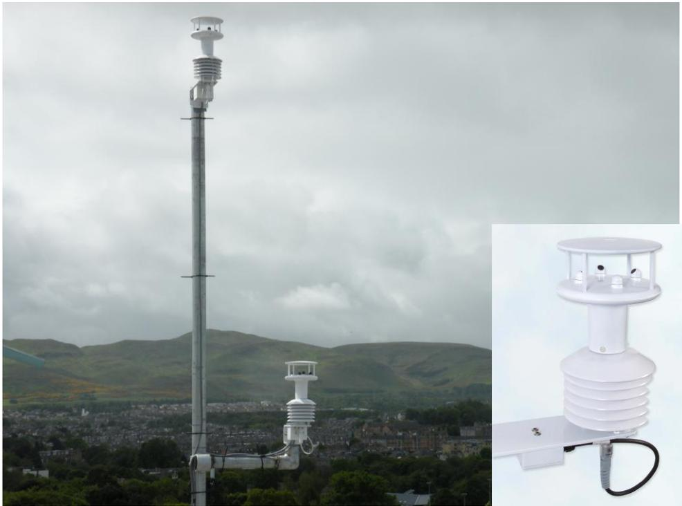
Figure 4-10: MetPak weather station on the right side and MetPak installed on the Merchiston roof on the left side.
