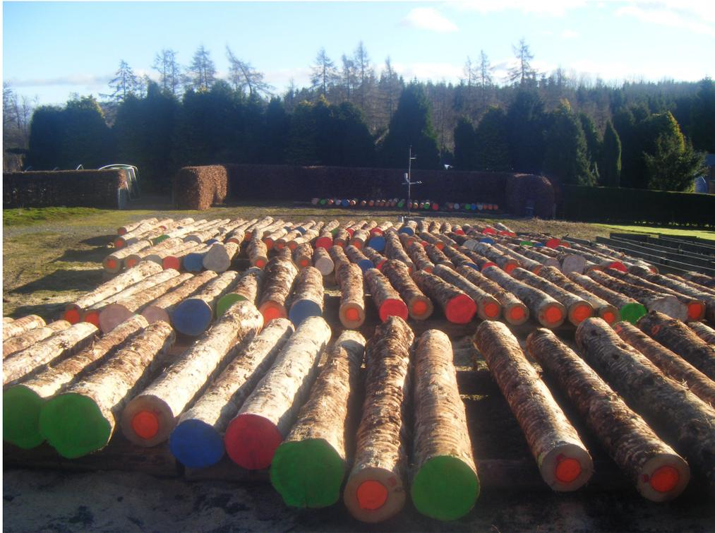
*Figure 6.3. Logs after being painted to identify log group and juvenile core.*
