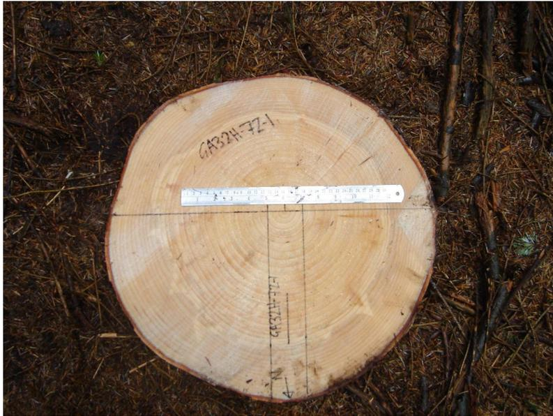
*Figure 4.2. Marking of 50 mm wide strip that was extracted from the breast height disc to verify corer density measurements.*
