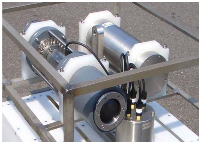
Figure 3.8: An image of a water and microplankton sampler (WMS) Envirotec AquaMonitor like that used by Cefas attached to the Smartbuoy moorings station Liverpool Bay and West Gabbard.
