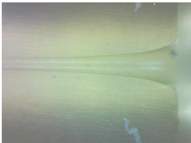
Figure 11.13: Cross section of one of the epoxy hyperbolic dies.
