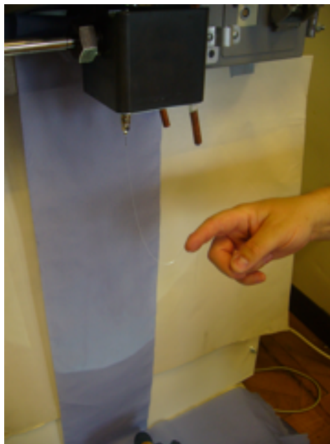
Figure 6.16: 100 micron wet fibre spun being drawn by hand from the die.
