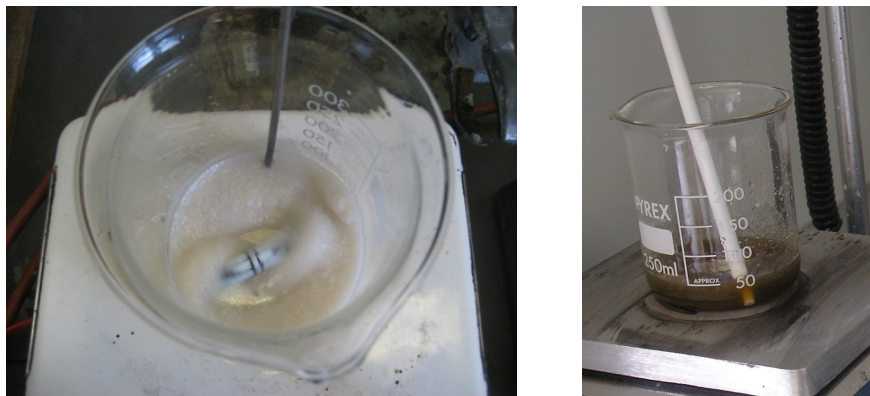
Figure 3.2: Hydrolysis of filter paper under 52.5% acid concentration at 46°C.
