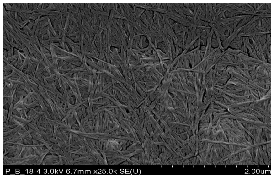
Figure 3.21: FEG-SEM image of bacterial cellulose nano-fibrils suspension after the fourth wash.
