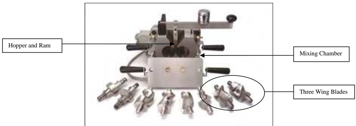
**Figure 5.4, Brabender Mixer Measuring Head**
