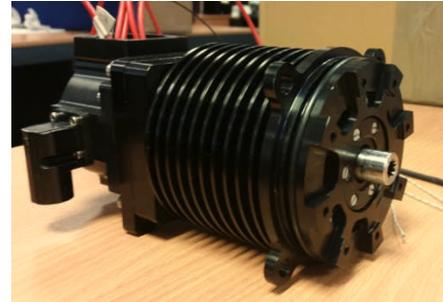
Fig. 5. Assembled PMSM prototype.
