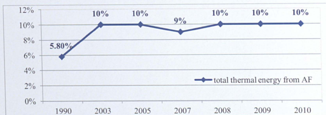
Figure 5.8 Improvement trends of total thermal energy efficiency from alternative fuels at Holcim between 1990 and 2010
