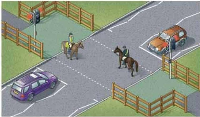
**Figure 2. 4: Pegasus crossing facility (sources: Highway Code)**
