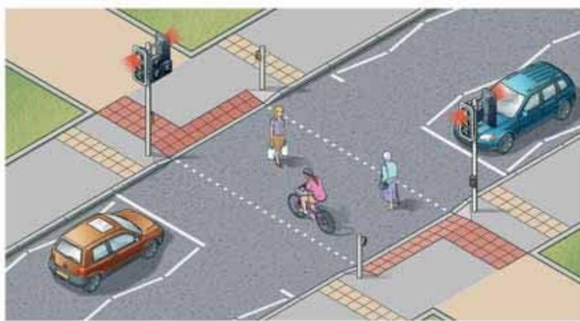
**Figure 2. 3: Puffin crossing facility (source: Highway Code)**
