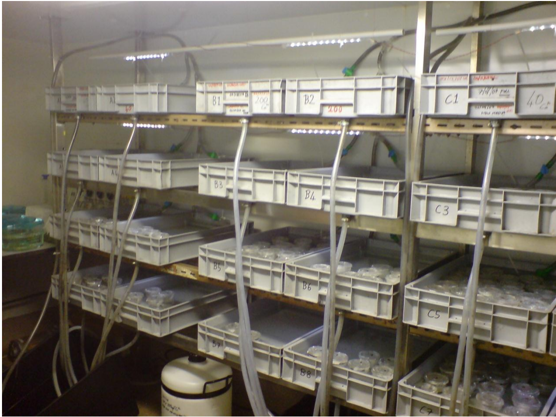
Figure 2.10. Flow through apparatus. Displaying systems A-C, with lighting system clearly visible above tanks.
