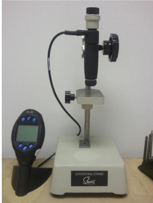
Fig. 3.22 The Shore 00 digital durometer
