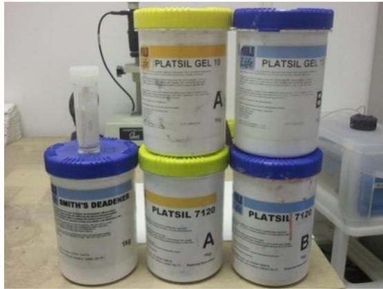
Figure 3.9 RTV raw silicone materials
