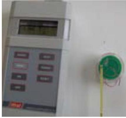
(c) Gauss meter measuring the magnetic flux density
