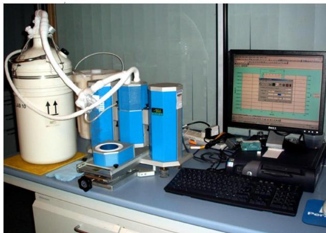
Fig 3.24 DMA tester [PE DMA 8000]
