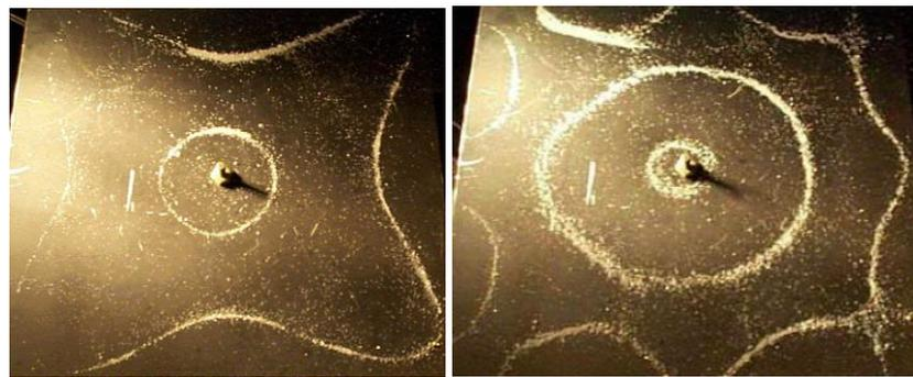
(a) Mode of the square panel at 340 Hz (left) and 800 Hz (right)
