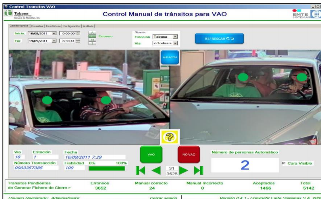
Figure 11-12 Automatic image processing to detect the number of occupants in each vehicle
